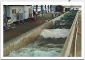
104 m long, 3.7 m wide, 4.6 m deep West Tank, W. M. Keck Hydraulics Laboratory of the California Institute of Technology US
