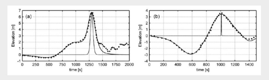
Superimposition of solitary waves on measurements for a) the Tohoku tsunami and b) the Indian Ocean tsunami, from Schimmels et al (2016)
