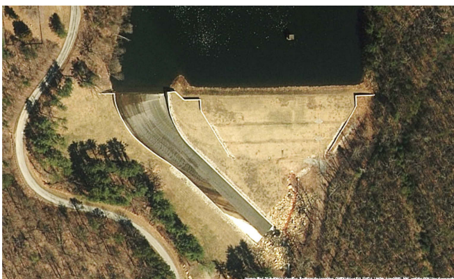
Figure 3. Stoney Creek Dam with Buried RCC Protection.
