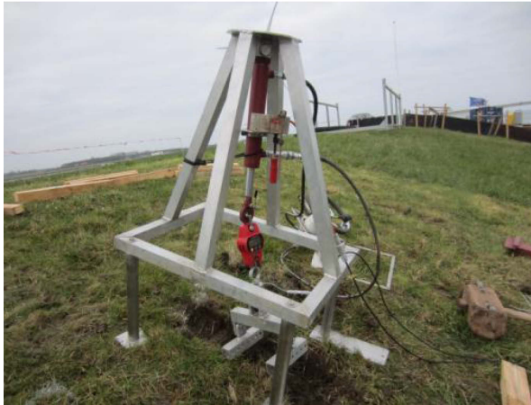
Figure 2.3 Overview of the sod pulling device
