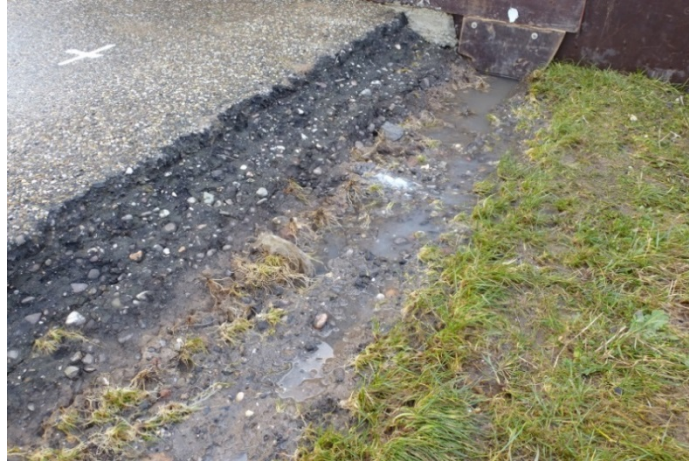
Figure 3.1a Less damage at transition from asphalt road to grass revetment (after 6h at the end of q = 1 \ell/s per m)
