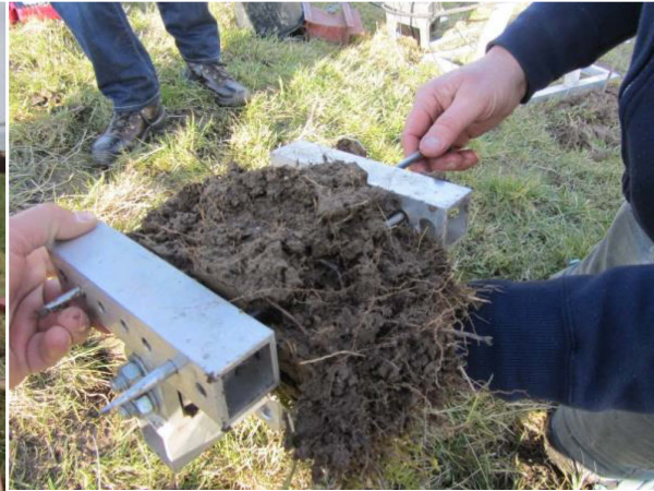
Figure 2.4 Small pull frame which anchors the sod
