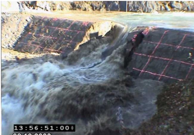
Figure 10. Breach erosion by vortex action undermining breach sides (Photo: IMPACT Project)
