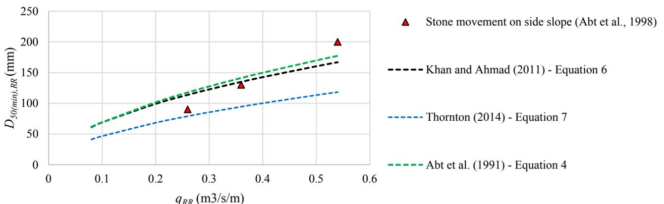
Figure 3: Empirical evaluation of Eq 4, 6 and 7 for stone movement on embankment side slope
