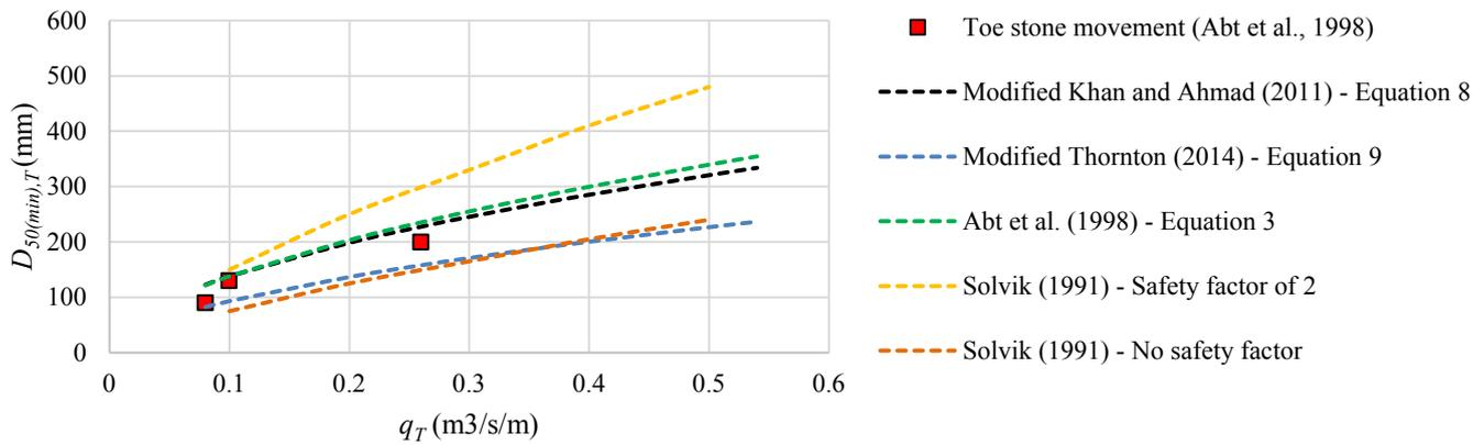
Figure 4: Empirical evaluation of toe stone sizing criteria
