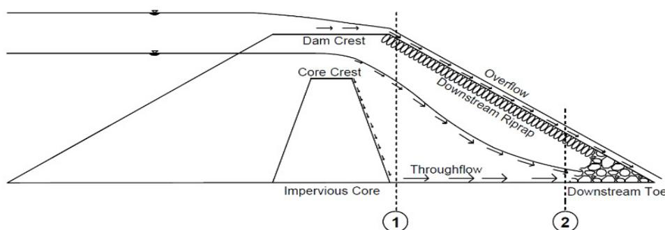
Figure 1: Throughflow and overflow scenarios in embankment dams
