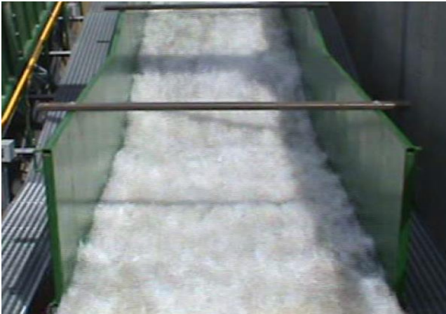
Figure 7. ARMORMAX tested on a full scale levee section for USACE (Thornton et al. 2012).
