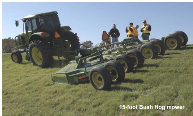
Figure 5. Anchored HPTRM reinforced vegetation being field tested in St. Charles Parish, Louisiana. USACE findings are that HPTRM technology is durable, maintainable, and is suitable for levee armoring.
