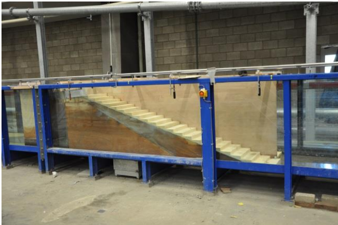
Figure 5. Impression of test series with 1:3 slope
