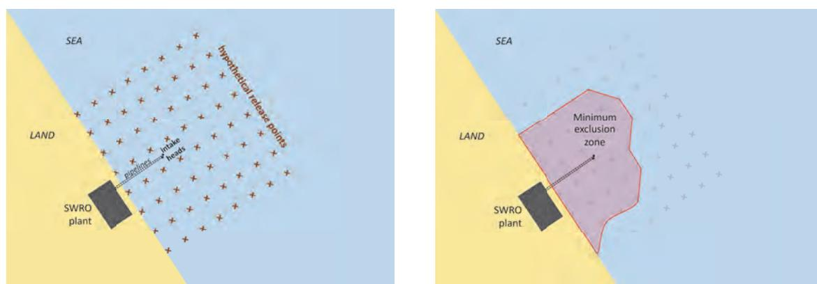
**Figure 1.** Example of (left) hypothetical pollutant / sediment release points around a coastal SWRO submerged pipeline intake system and (right) establishment of "minimum exclusion" buffer zone using release points found to affect the intake at an agreed threshold level.
