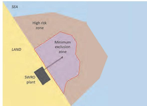
**Figure 2.** Example of a wider area high risk zone around an intake, established through testing of hypothetical coastal and offshore developments, chosen to protect wider hydrodynamic pathways to the intake.
