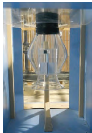
Figure 2. Swirl meter installation scheme as per ANSI/HI-9.8 standard (left) and example swirl meter installation in a physical model (right).
