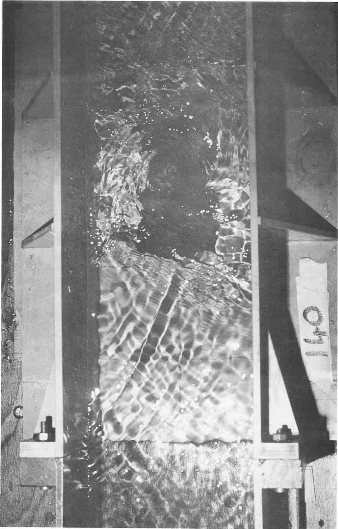
Plate II Orifice flow at rectangular outlet (Test C3) by courtesy of BHRA
