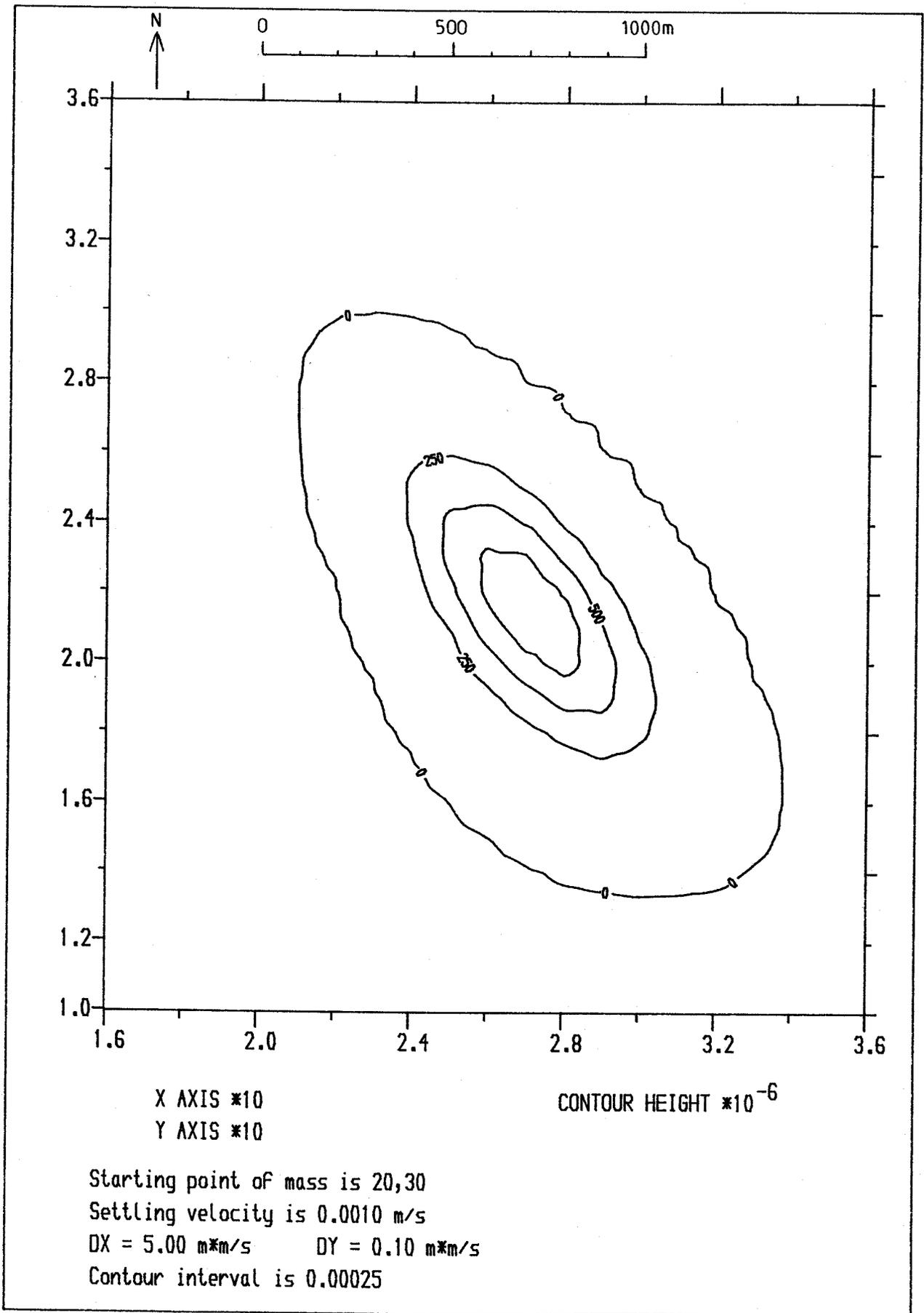
Fig 14 Concentrations in suspension
