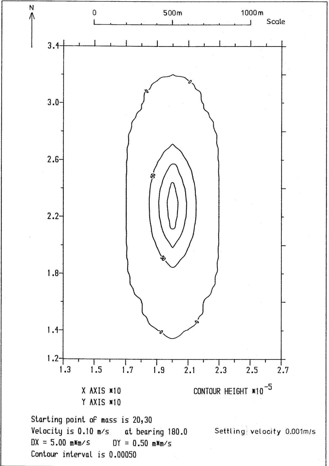
Fig 3. Concentrations in suspension after 120 minutes
