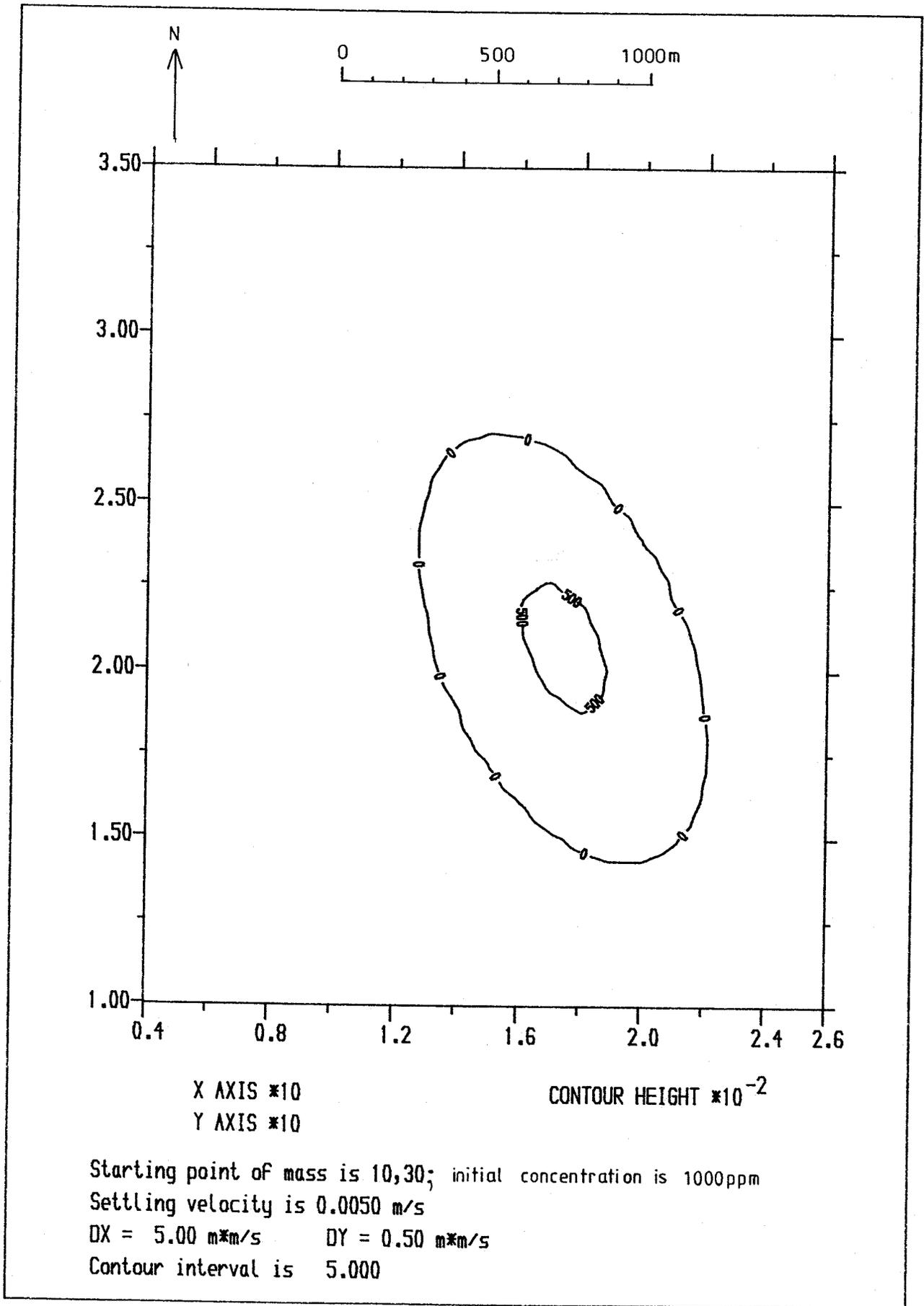
Fig 18 Concentrations in suspension (in ppm)
