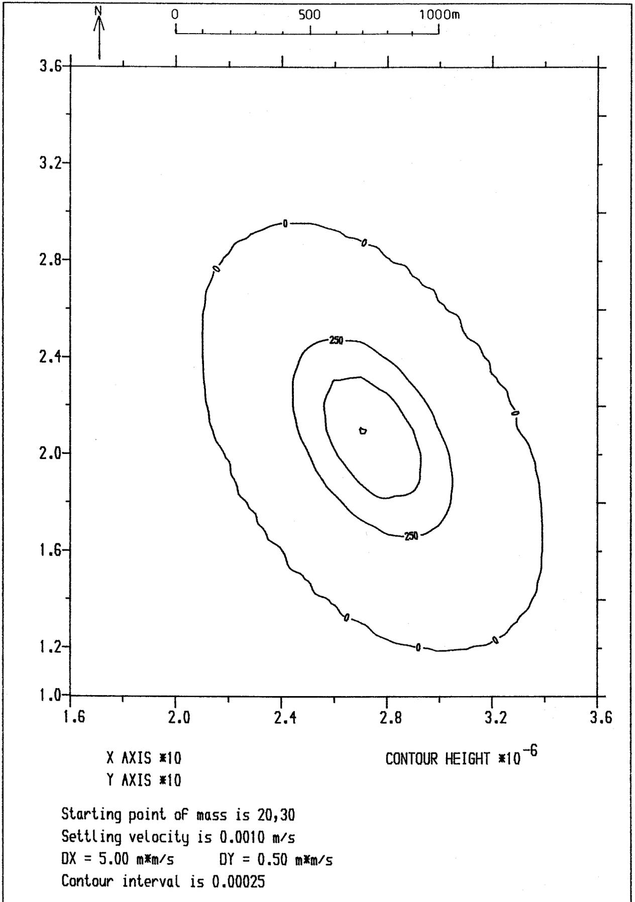
Fig 13 Concentrations in suspension
