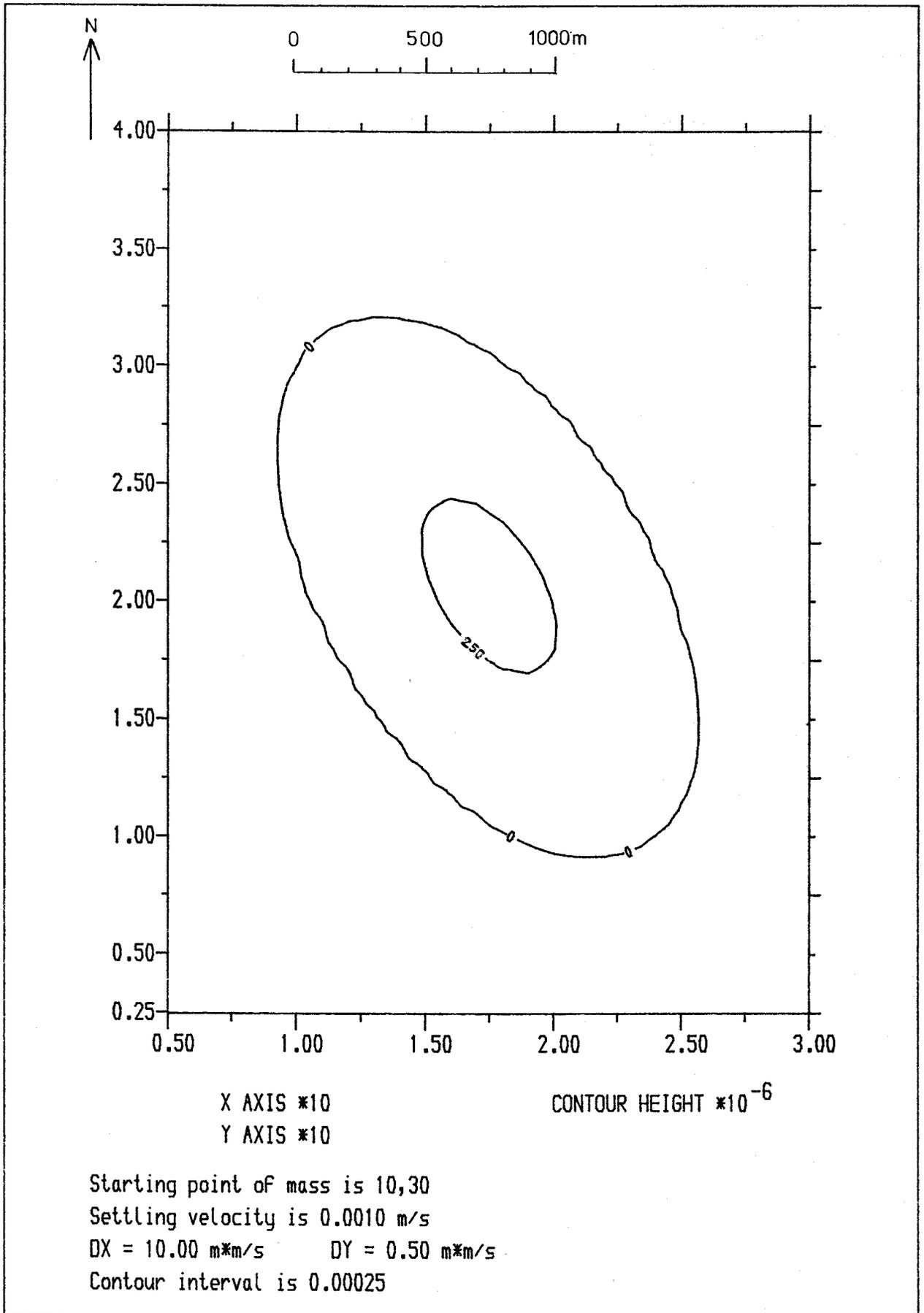
Fig 9      Concentrations in suspension
