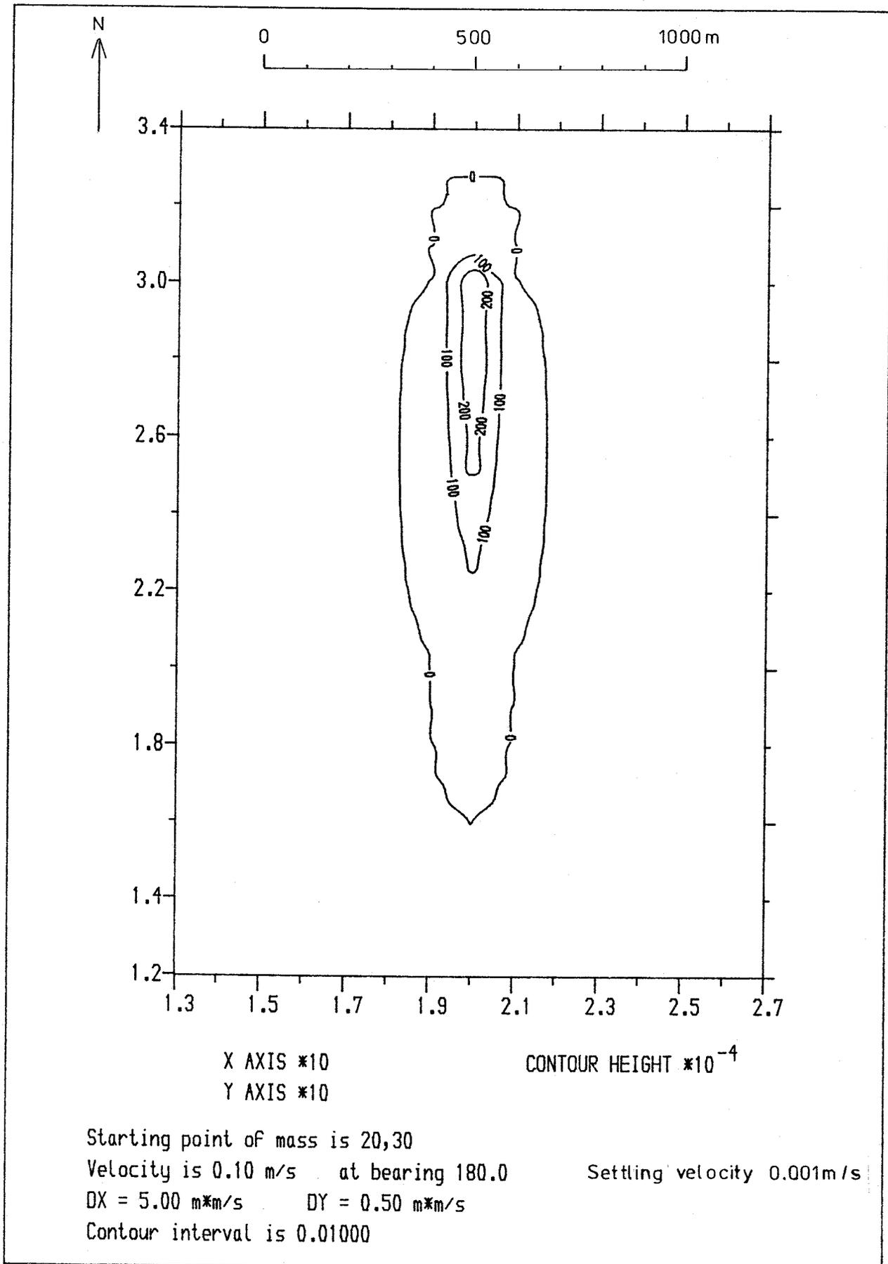
Fig 8 Distribution of mass on the bed after 120minutes
