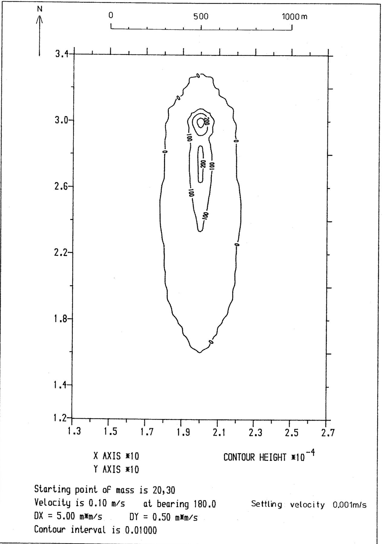
Fig 7 Distribution of mass on the bed after 120 minutes
