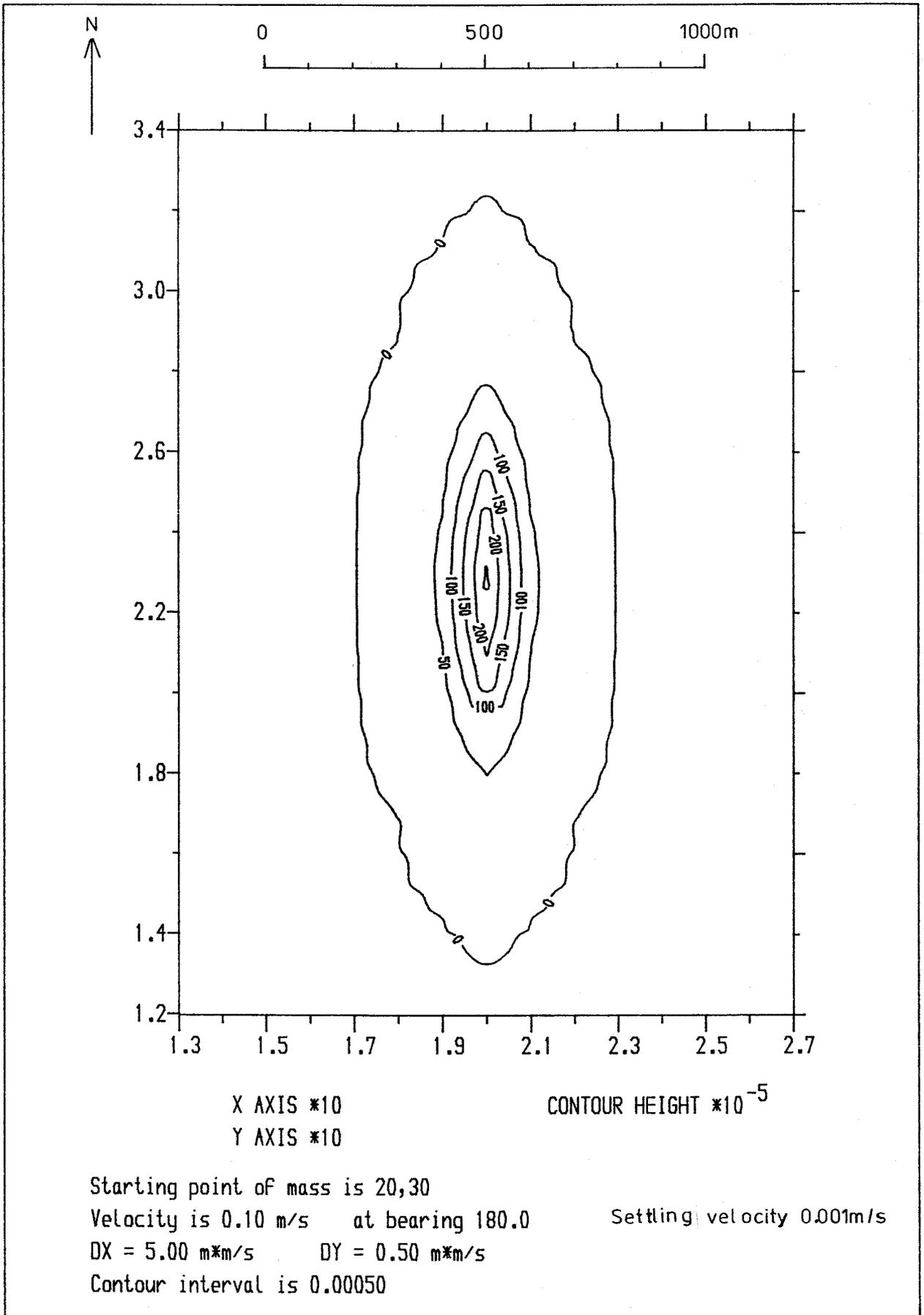
Fig 5 Concentrations in suspension after 120 minutes
