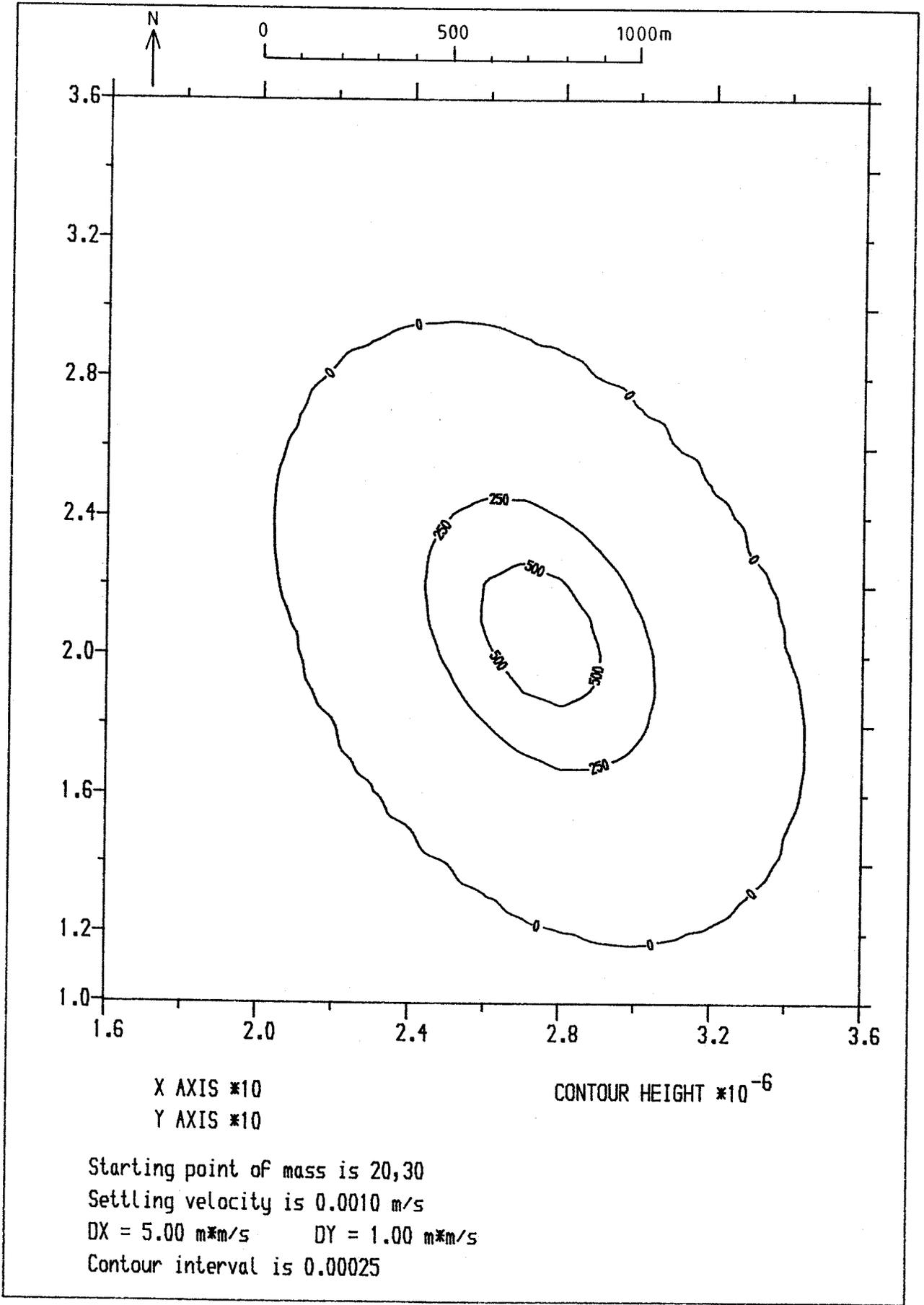
Fig 12 Concentrations in suspension
