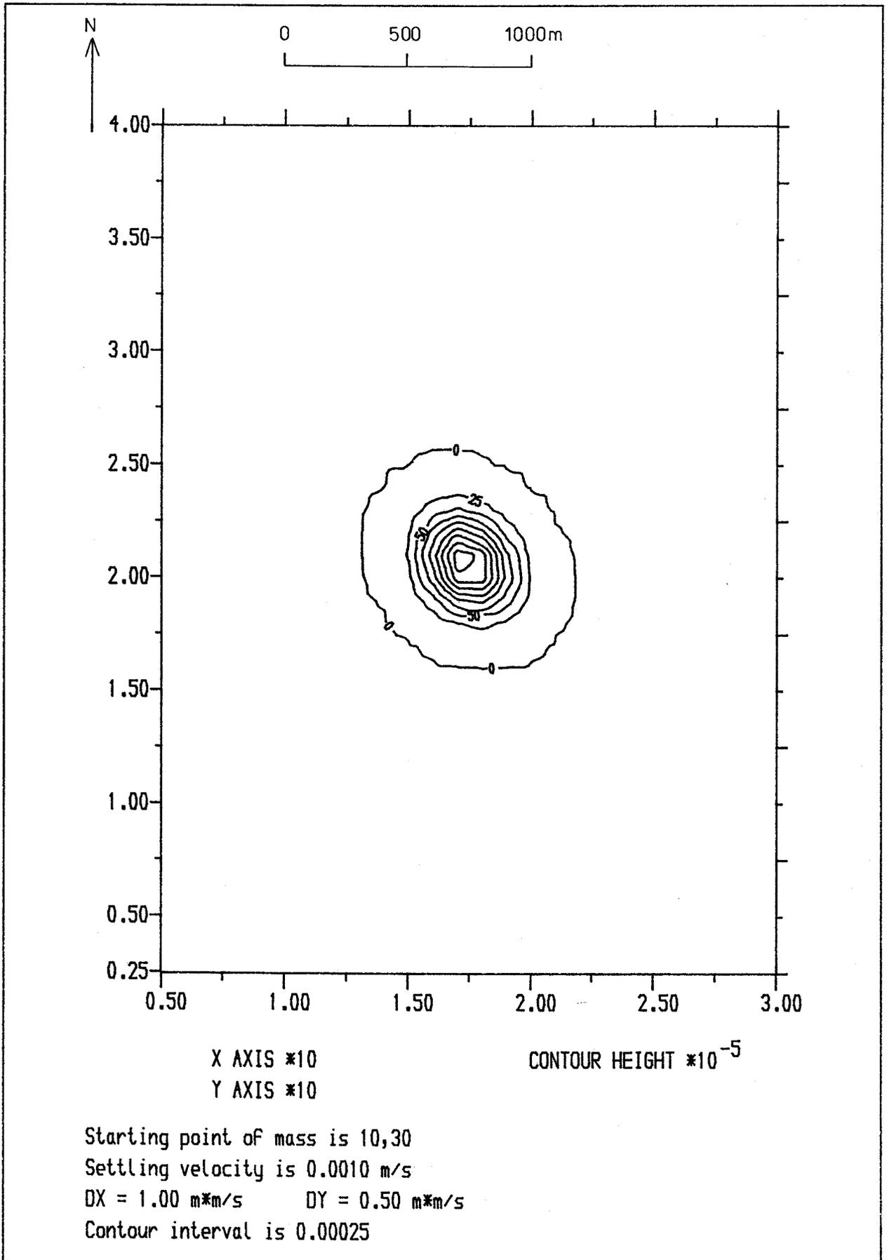
Fig 11 Concentrations in suspension
