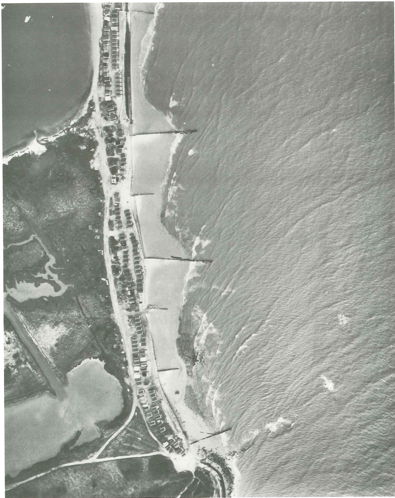
Plate 1 Coastline at Mudeford Sandspit near Bournemouth, England showing refraction of waves
