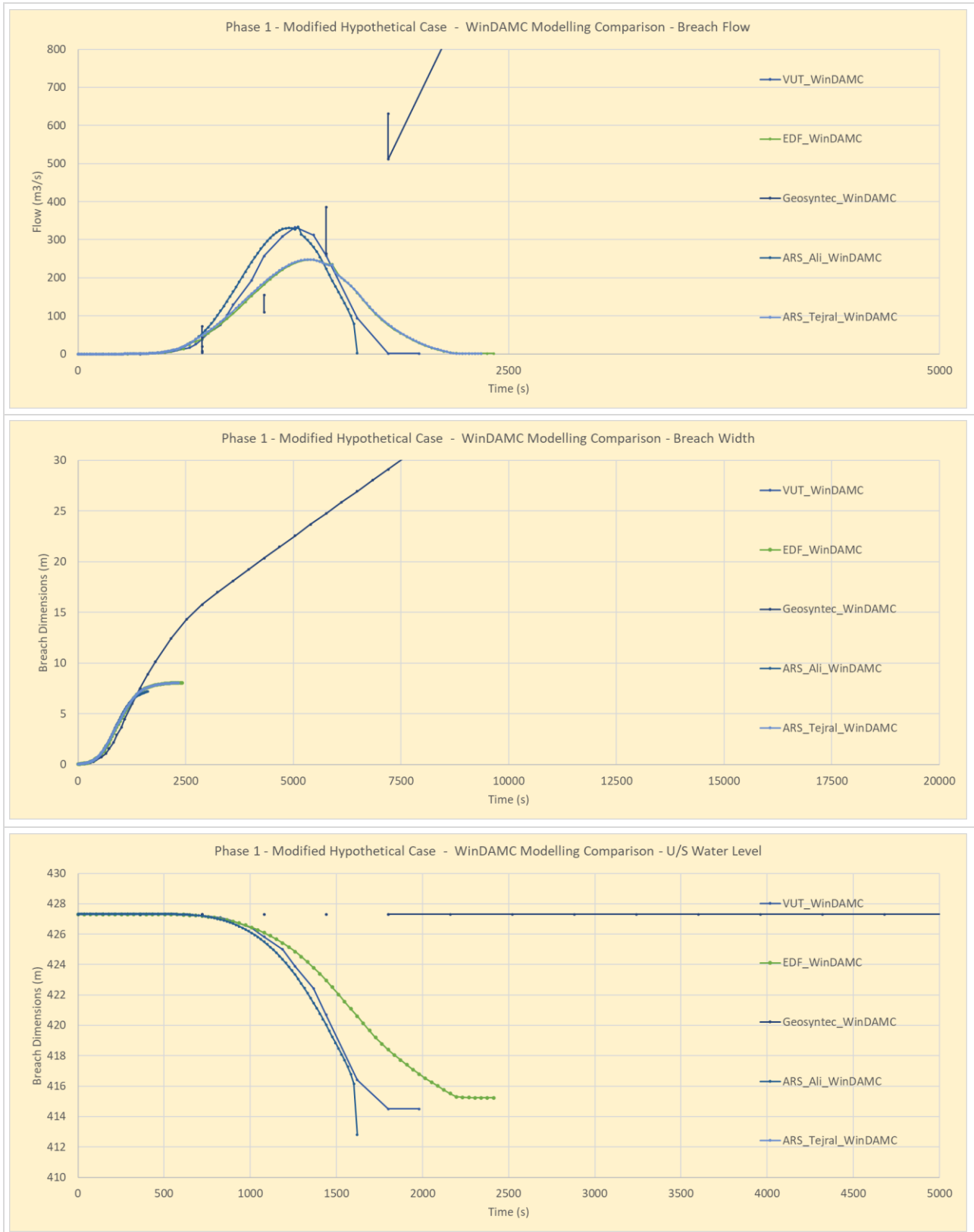
Figure C.8: Phase 1 – Modified Hypothetical: Modelling results using WinDAM C
