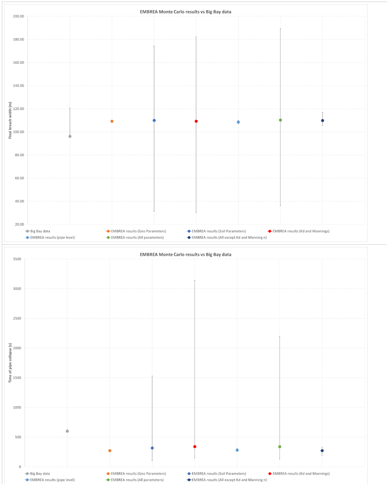
Figure J.19: Phase 3: Big Bay – HRW: Bw range and Tpc range for different MC analyses
