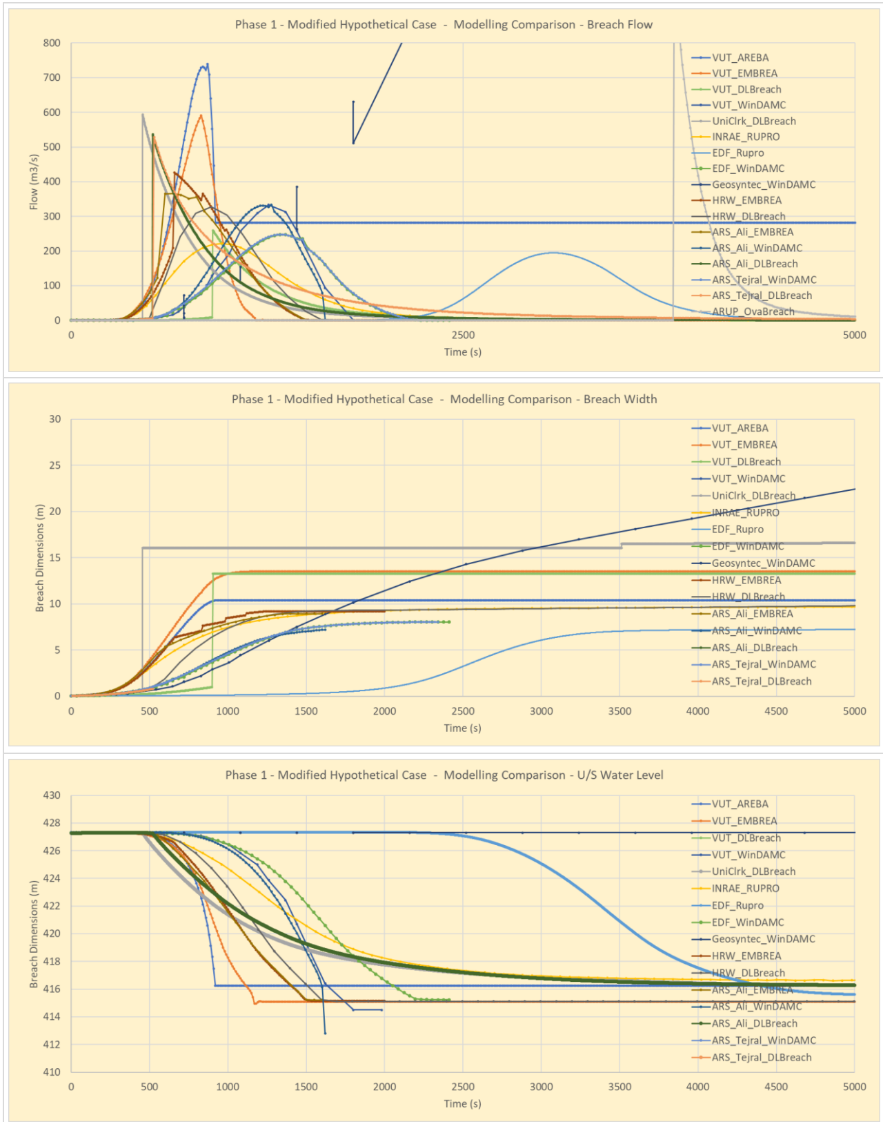
Figure C.3: Phase 1 – Modified Hypothetical: All modelling results – focus on t=0-5000 s
