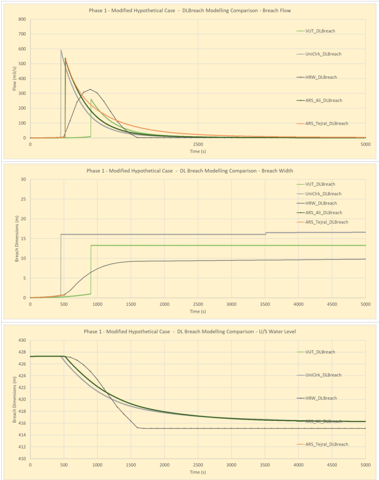
Figure C.7: Phase 1 – Modified Hypothetical: Modelling results using DLBreach
