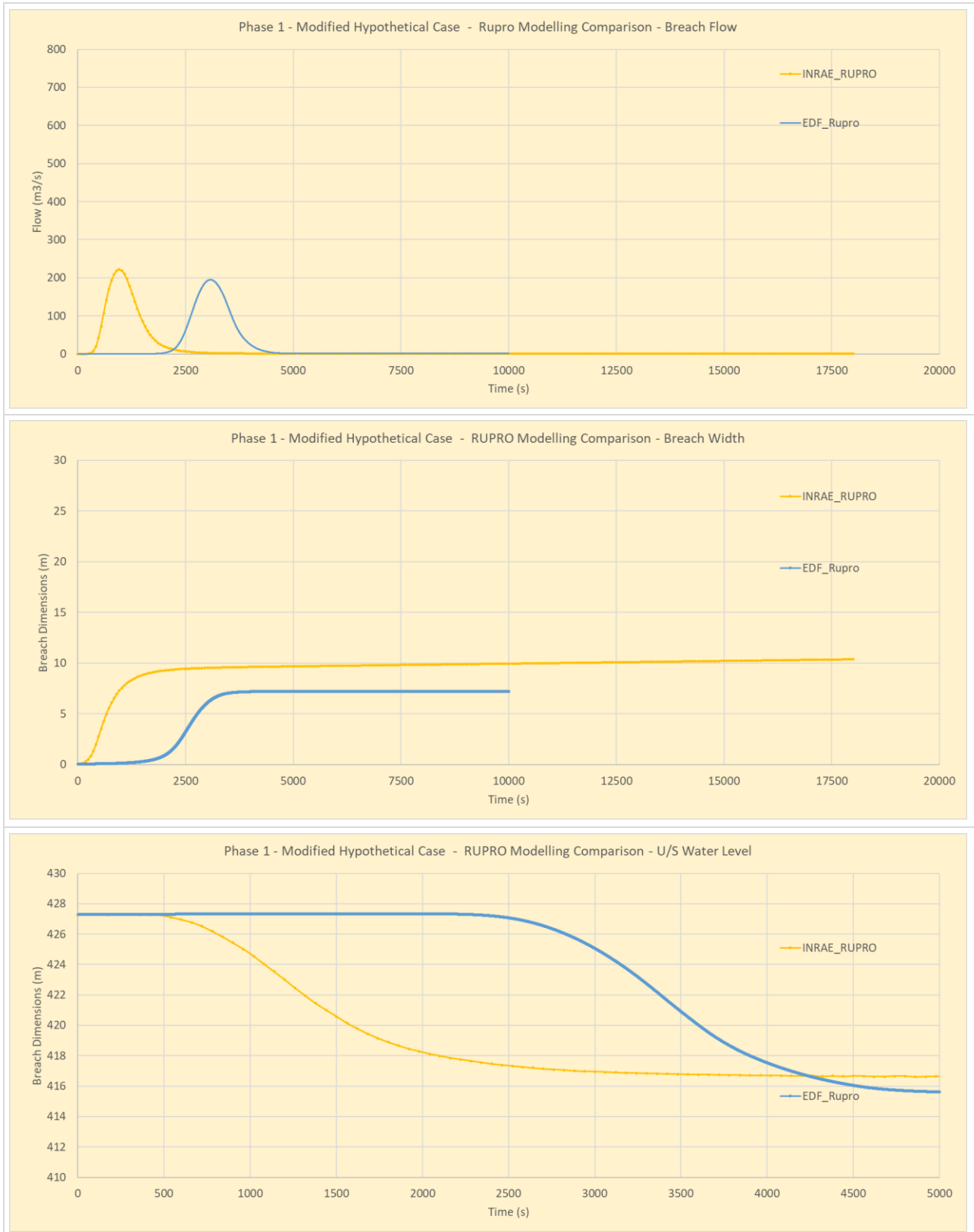
Figure C.9: Phase 1 – Modified Hypothetical: Modelling results using Rupro
