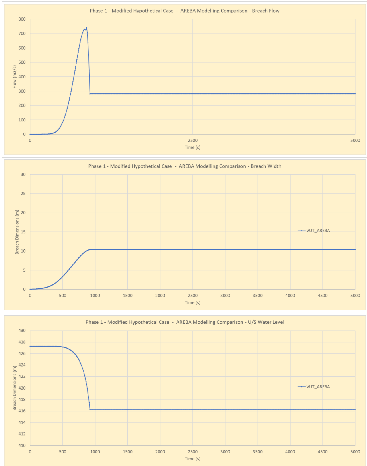
Figure C.5: Phase 1 – Modified Hypothetical: Modelling results using AREBA
