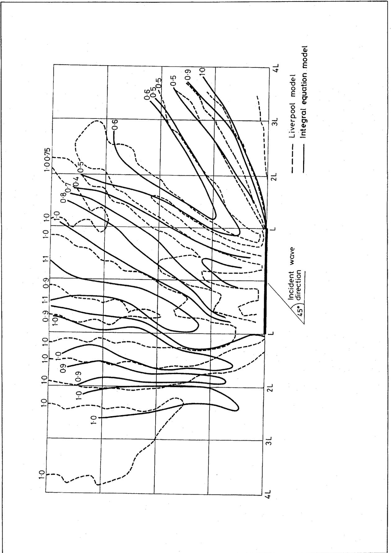
Fig 6 Liverpool model - wave height coefficients for an insular breakwater, length 2 wavelengths (L), constant depth profile, 45° incidence
