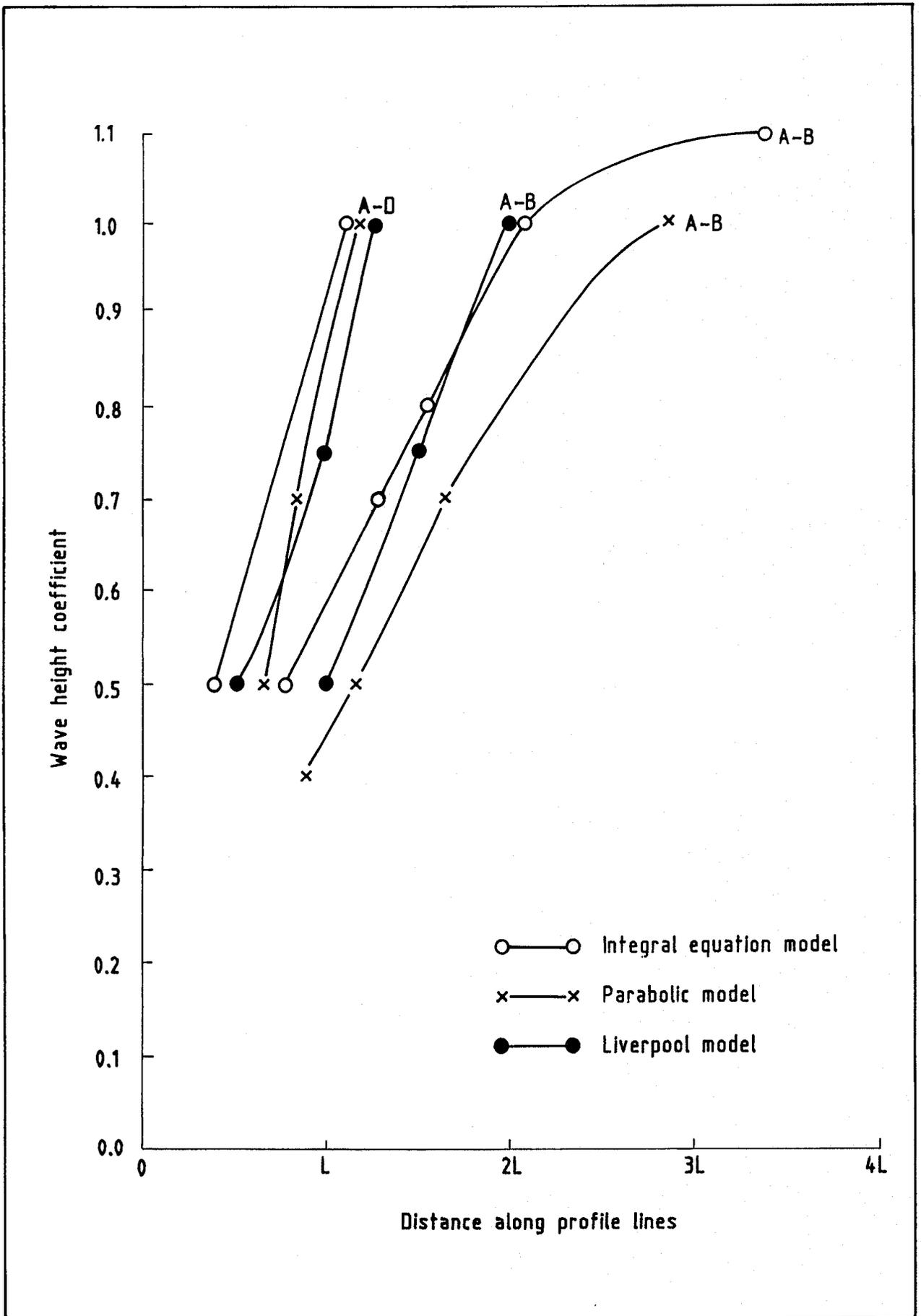
Fig 7 Comparison of model results - 45° incidence, constant depth.
