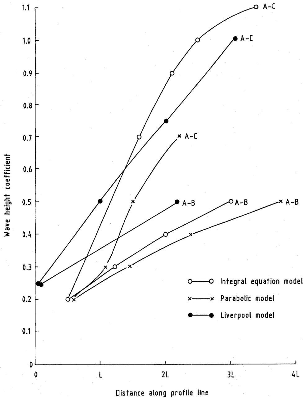
Fig 4 Comparison of model results - normal incidence, constant depth
