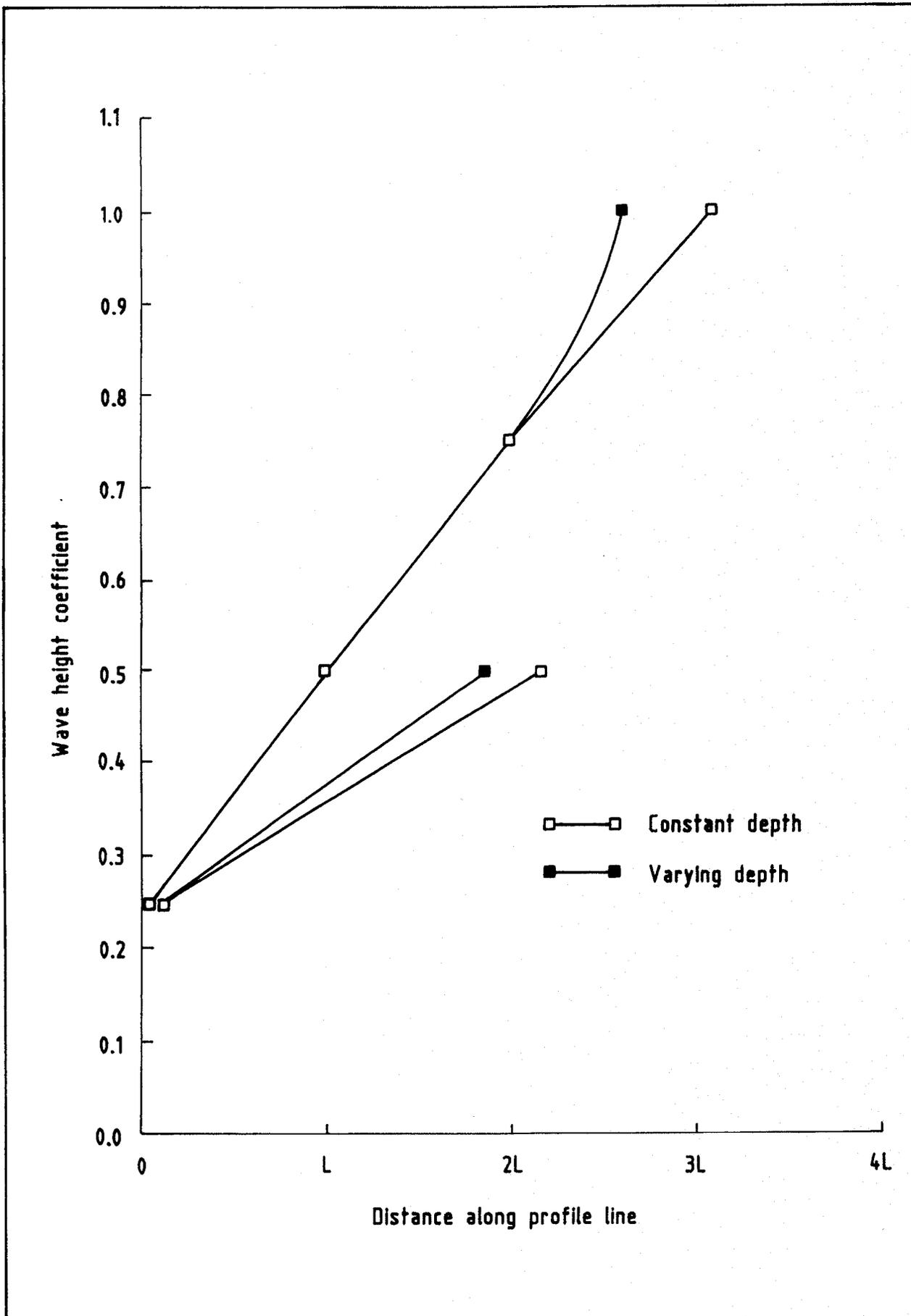
Fig 11 Comparison of Liverpool model results for constant and varying depth cases
