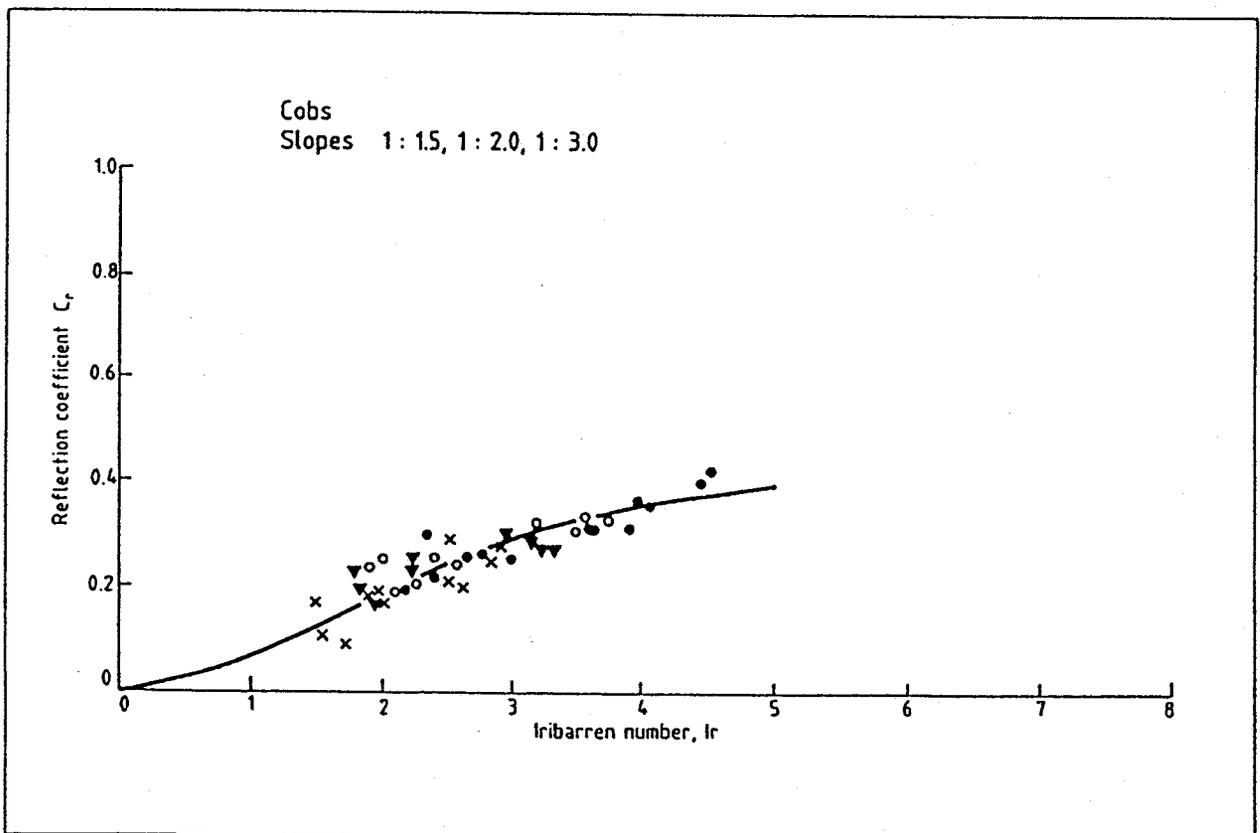
Fig 3.2 Reflection performance of cob armoured slopes
