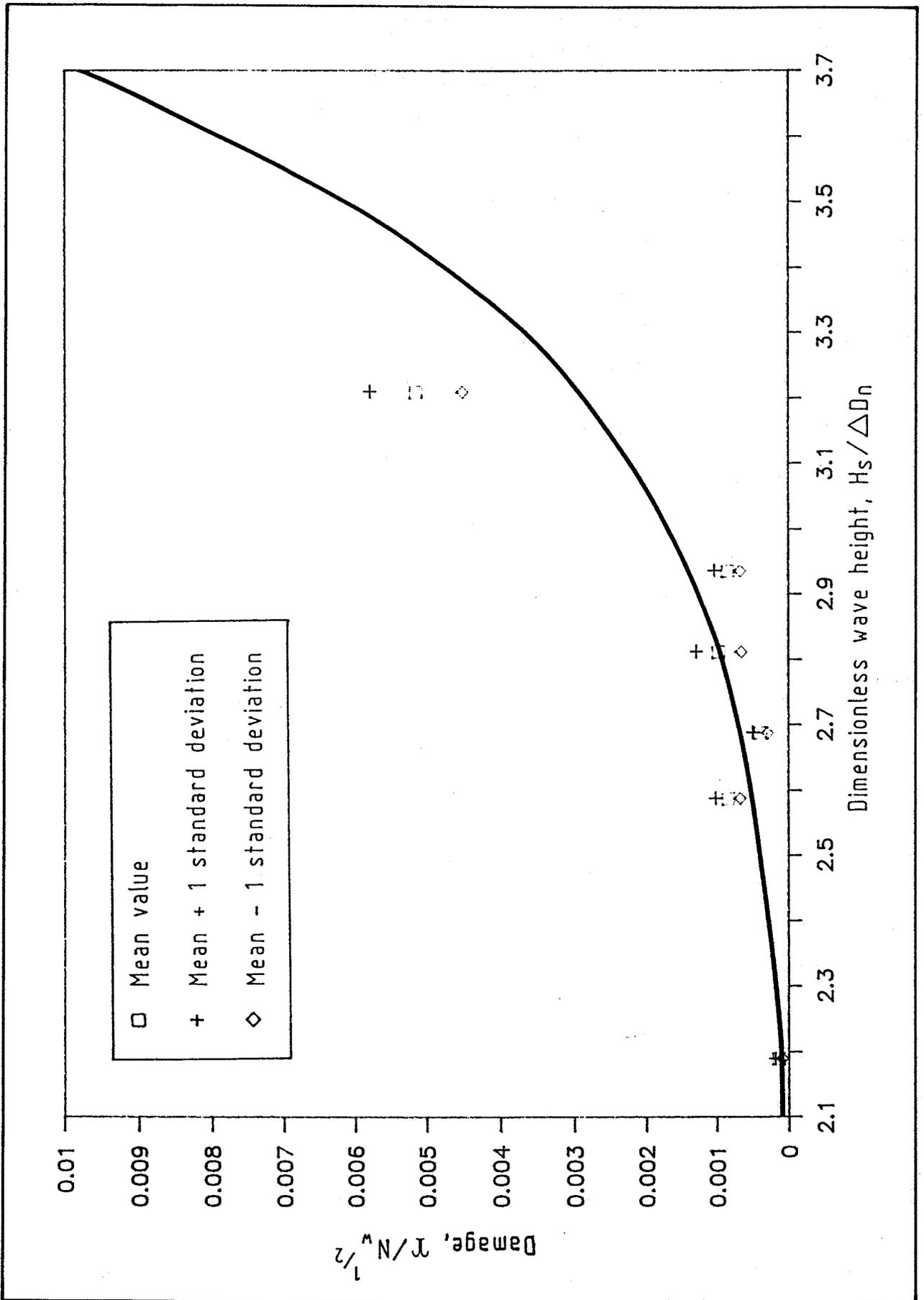
Fig A2.6 Damage against  $H_s/\Delta D_n$ , short crested waves, mean values
