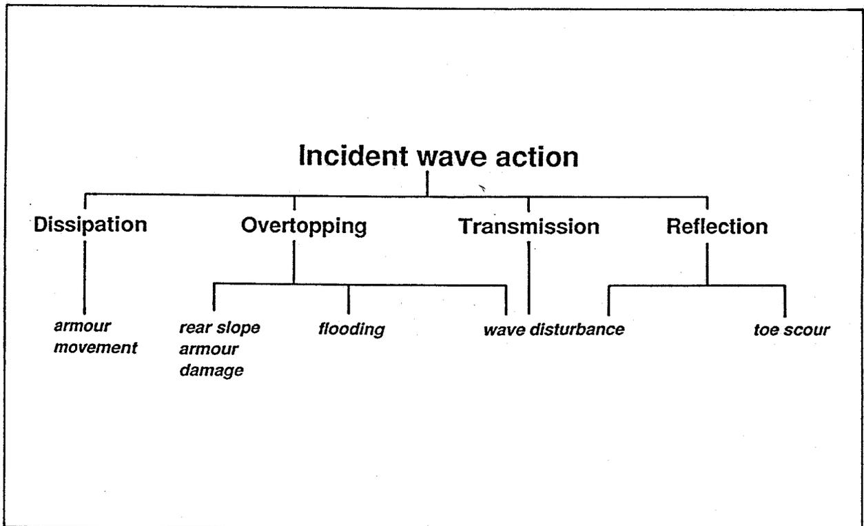
Fig 1.2. Effects of incident wave energy
