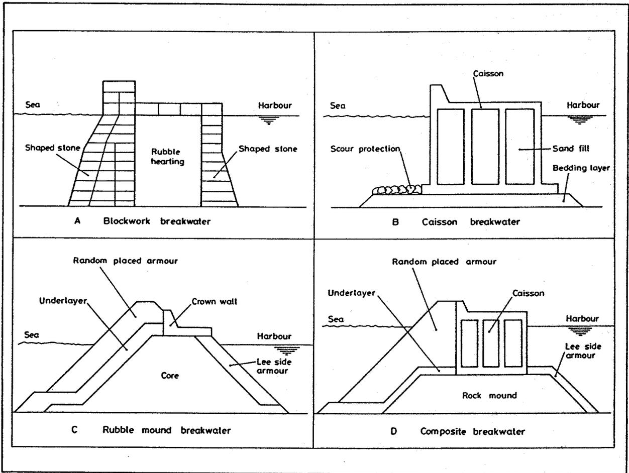
Fig 1.1 Breakwater types, after Owen (Ref. 1)
