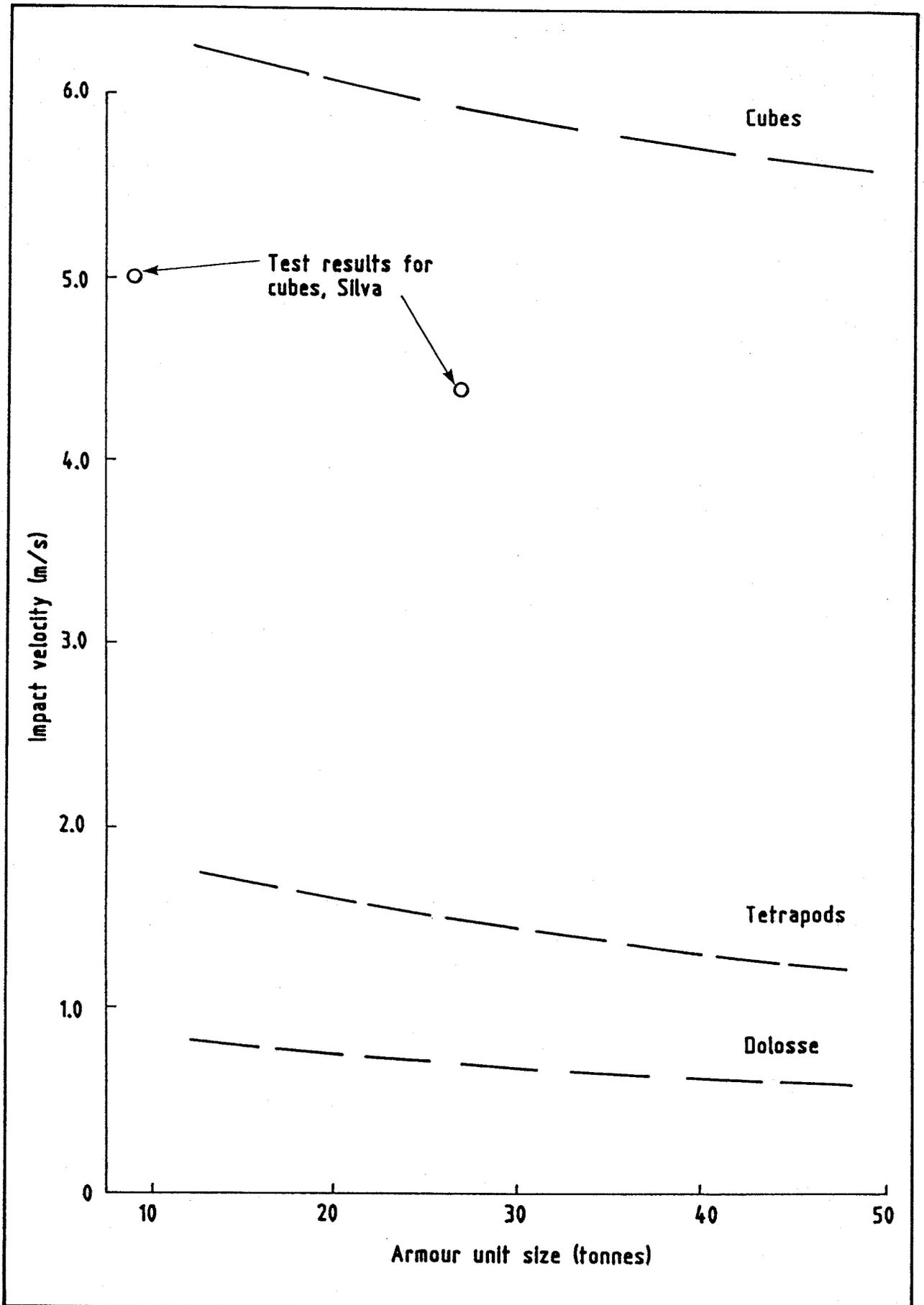
Fig 5.2 Limiting impact velocity for failure of Dolos, Tetrapod or Cubes
