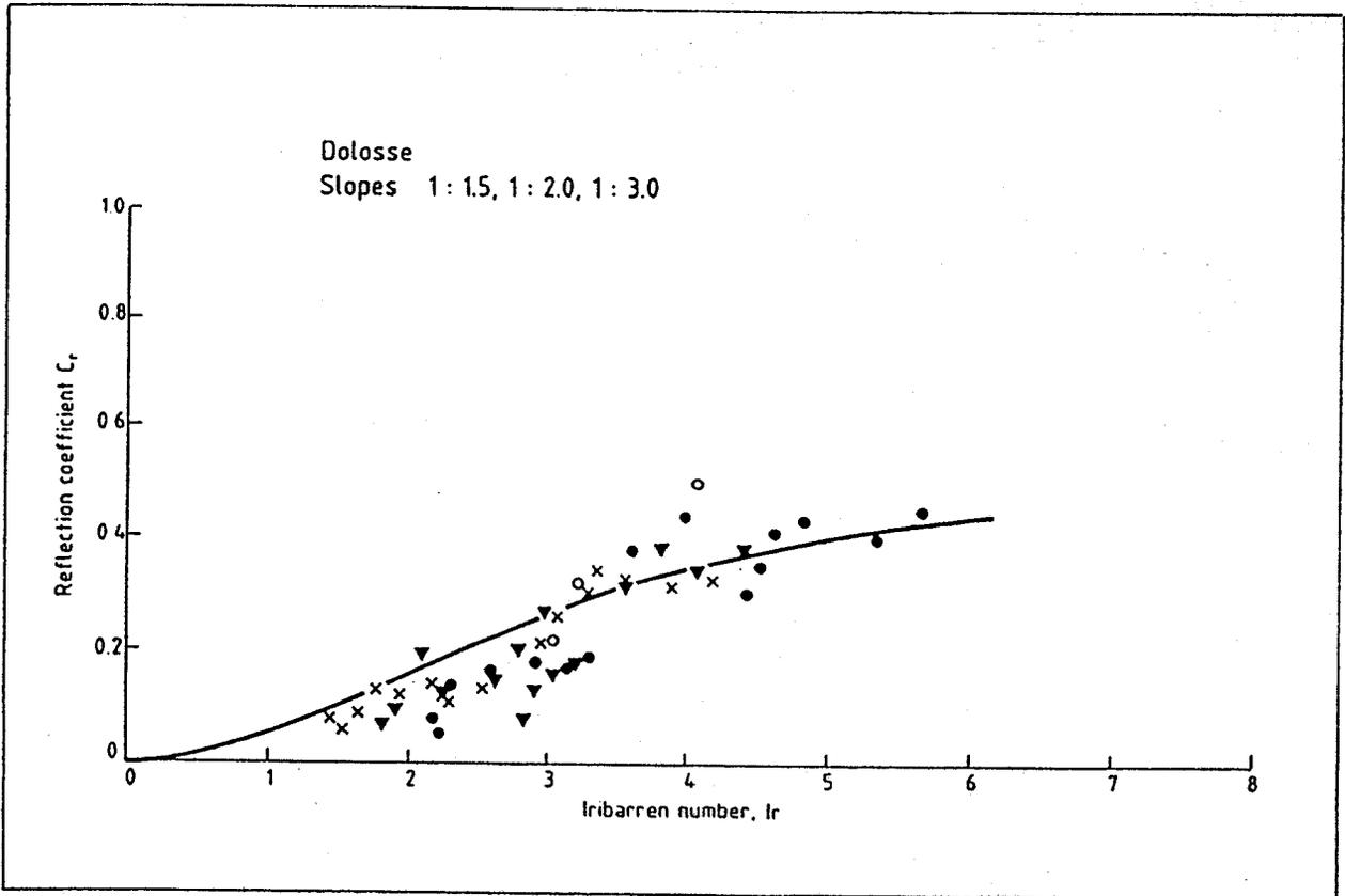
Fig 3.1 Reflection performance of Dolos armoured slopes
