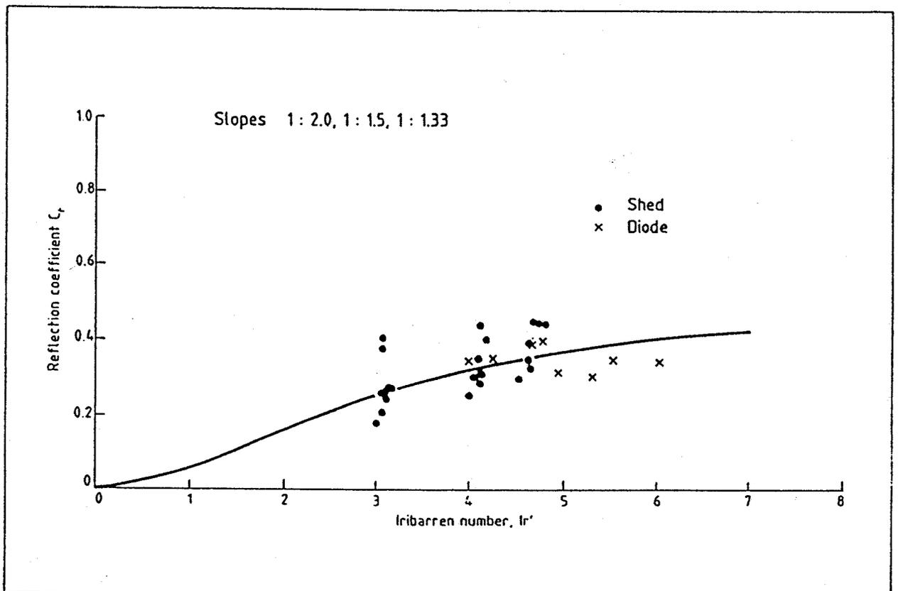
Fig 3.4 Reflection performance of Shed or Diode armoured slopes
