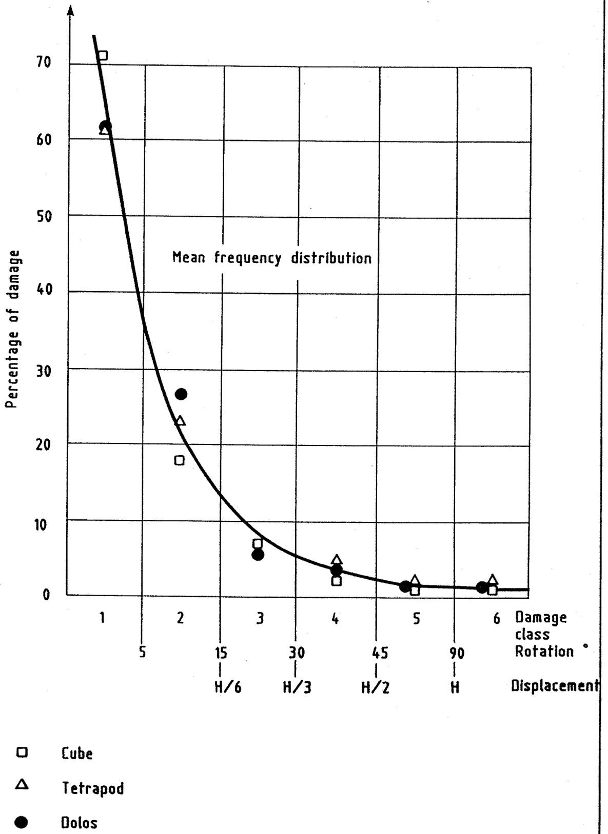
Fig 4.2 Distribution of levels of damage after Partensky et al (Ref 62)
