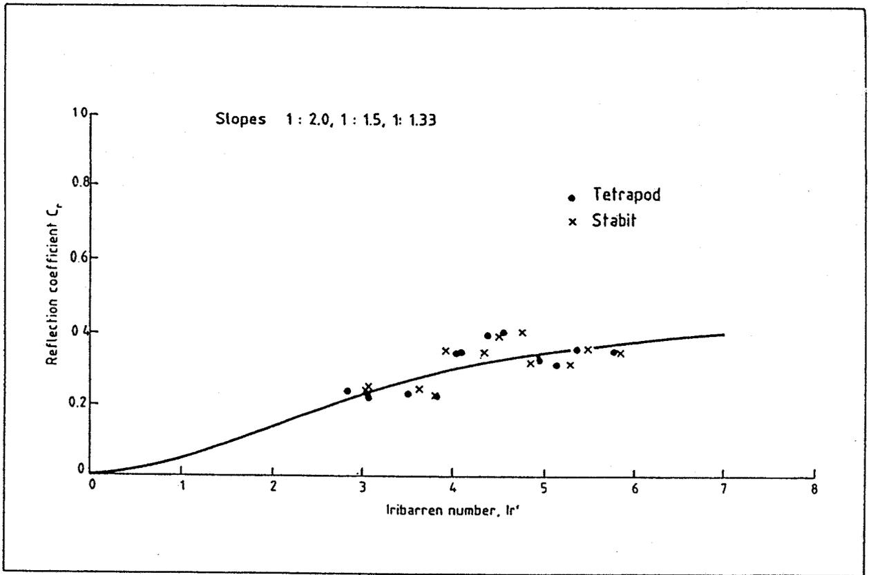
Fig 3.3 Reflection performance of Tetrapod or Stabit armoured slopes
