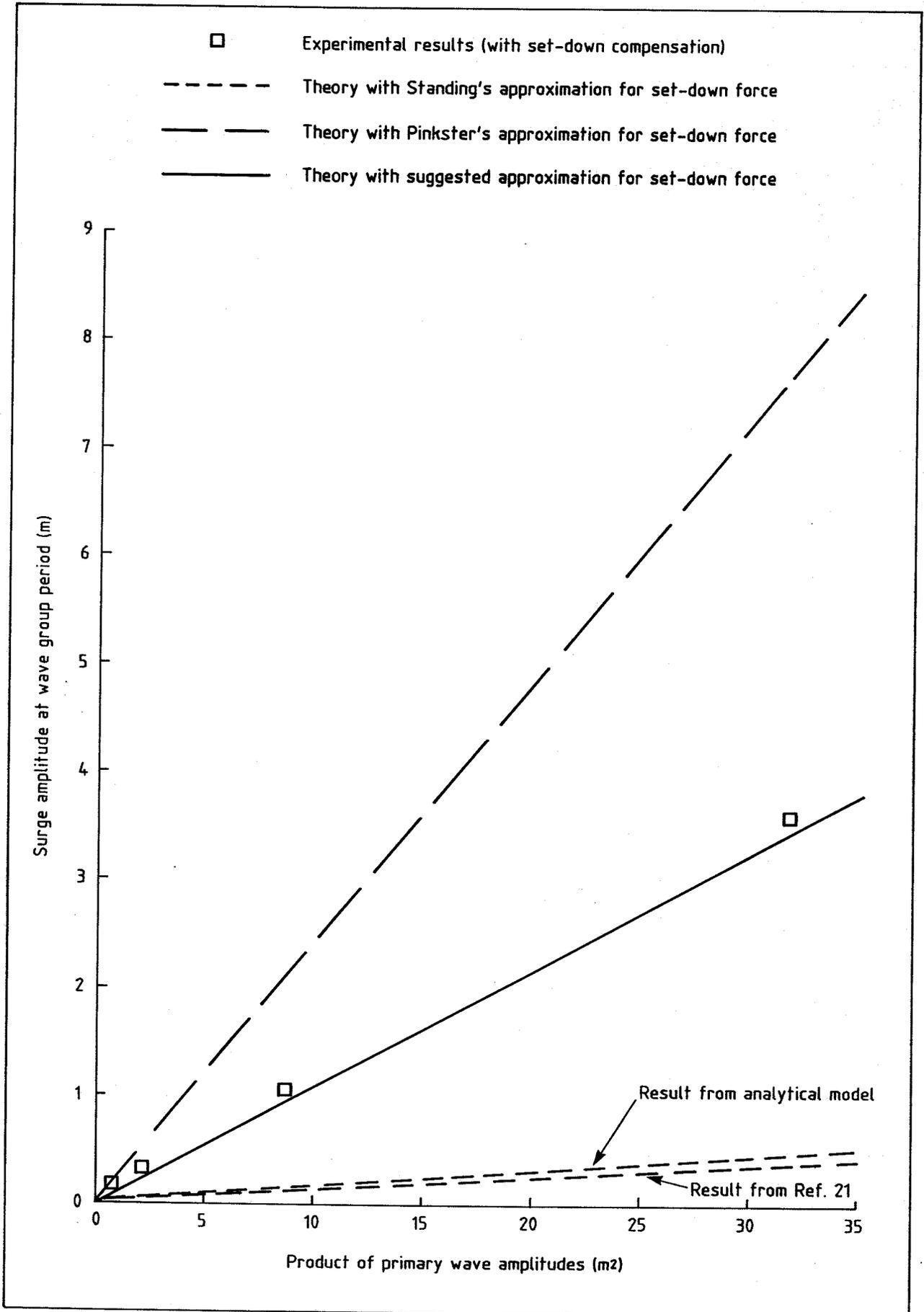
Fig 10 Experimental and theoretical non-linear surge ( $T_1 = 20s, T_2 = 14.5s$ )
