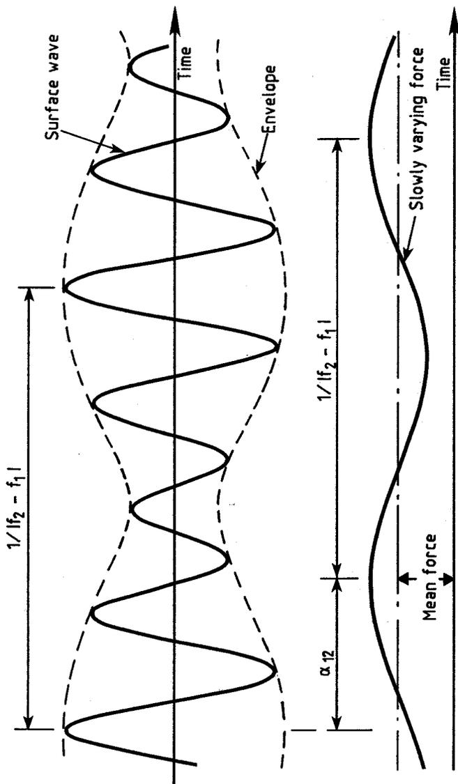
Fig 3 Regular wave groups and resulting non-linear wave force
