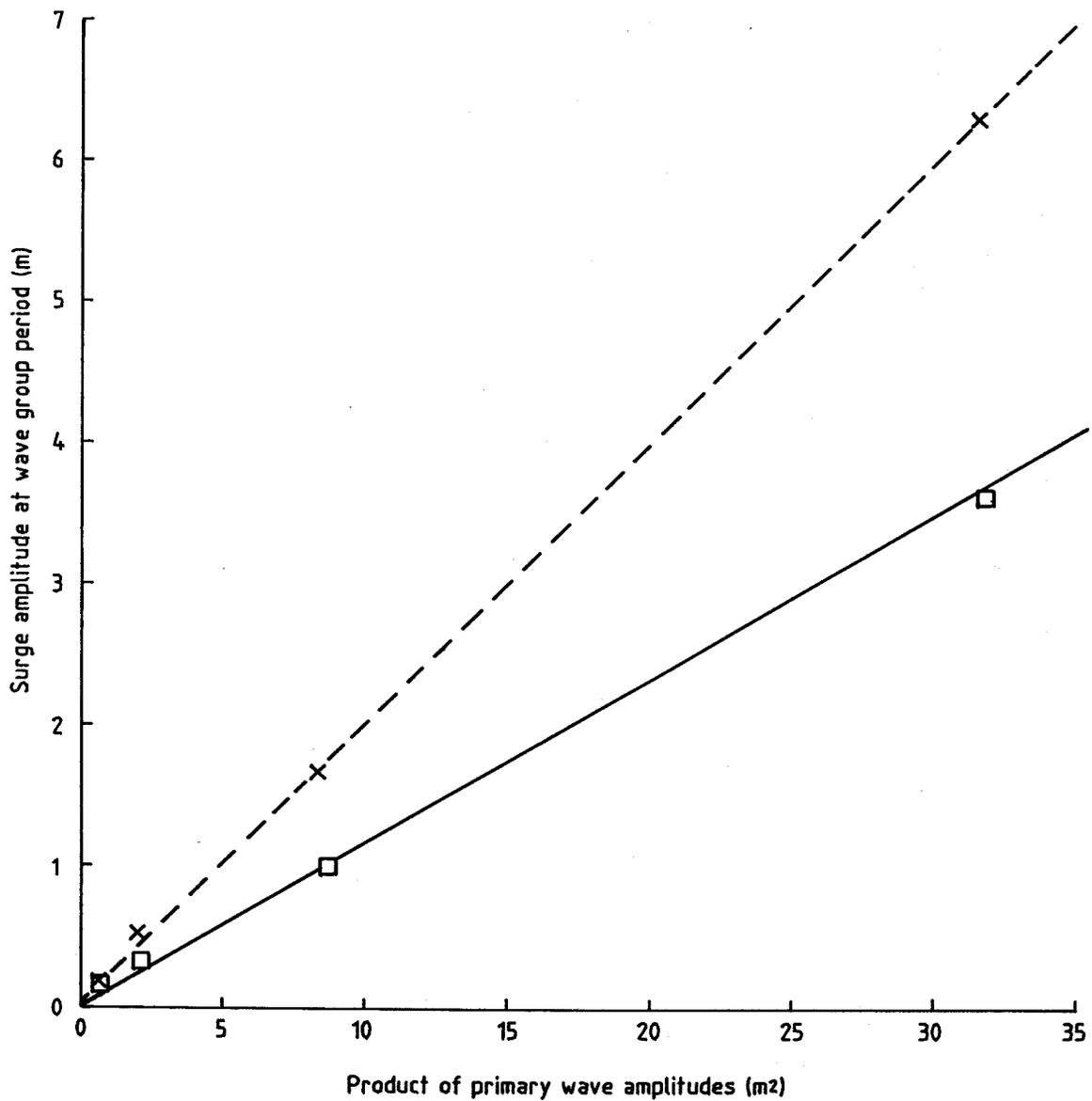
Fig 7 Experimental non-linear surge ( $T_1 = 20s$ ,  $T_2 = 14.5s$ )
