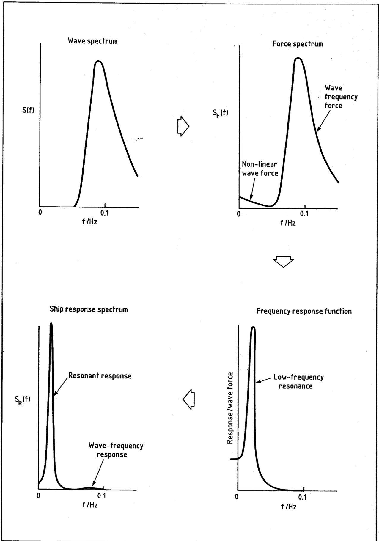
Fig 1 Schematic diagram of resonant excitation of a ship on its moorings
