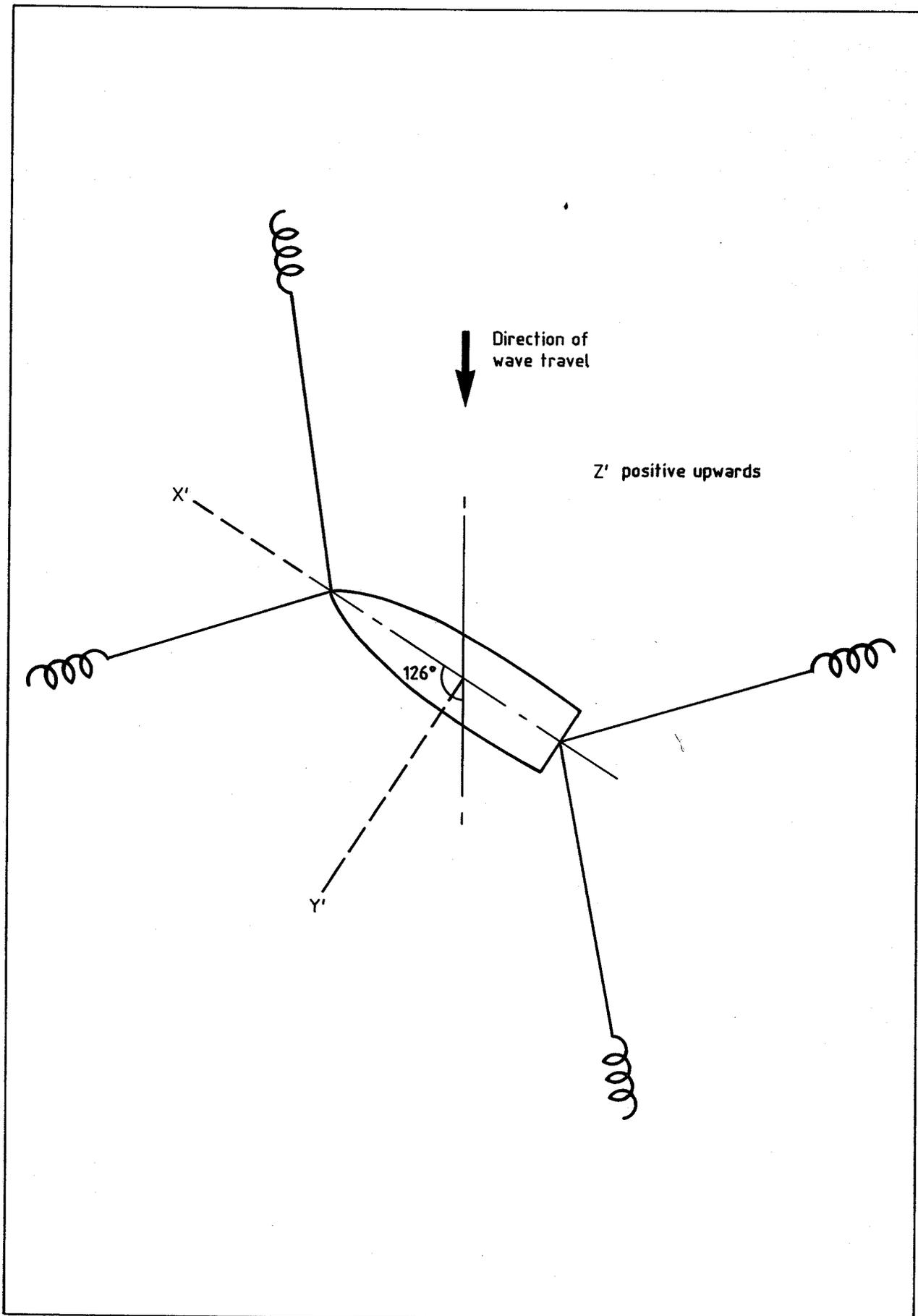
Fig 4 Mooring layout of a vessel in quartering seas
