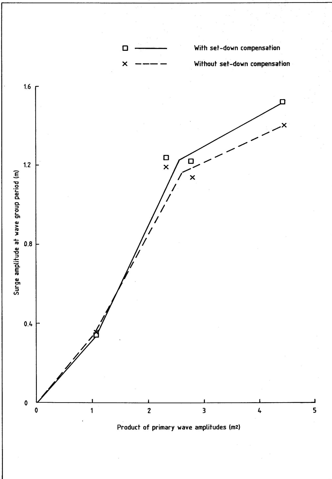
Fig 9 Experimental non-linear surge ( $T_1 = 10.0s$ ,  $T_2 = 8.4s$ )
