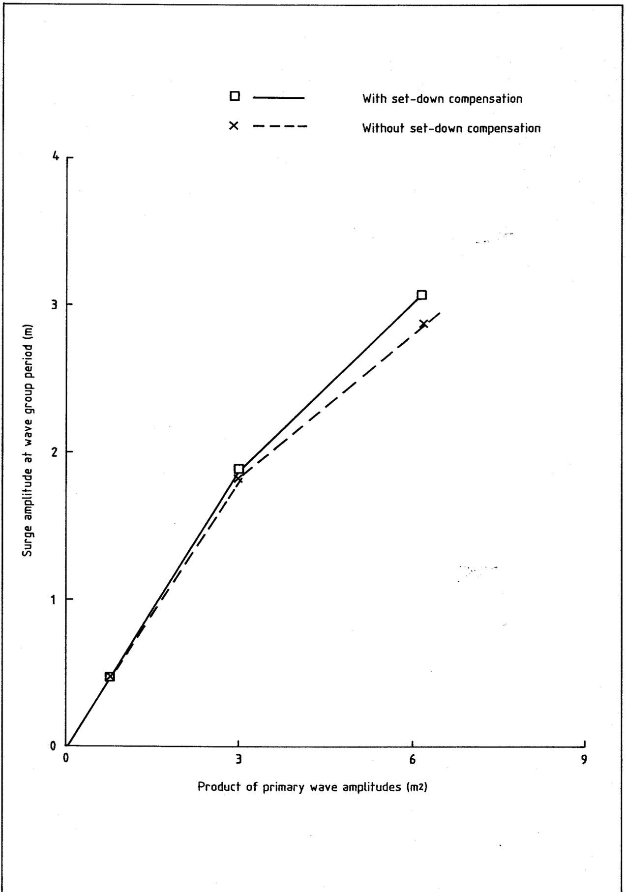
Fig 8 Experimental non-linear surge ( $T_1 = 12.4s$ ,  $T_2 = 10.0s$ )
