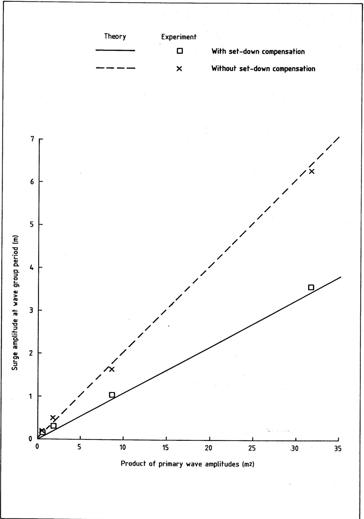
Fig 11 Comparison of experimental results with theory using suggested approximation for set-down force ( $T_1 = 20s$ ,  $T_2 = 14.5s$ )
