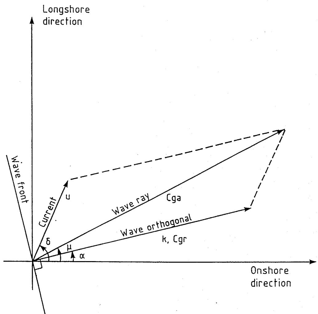
Fig 1 Geometry of currents, wave orthogonals and wave rays
