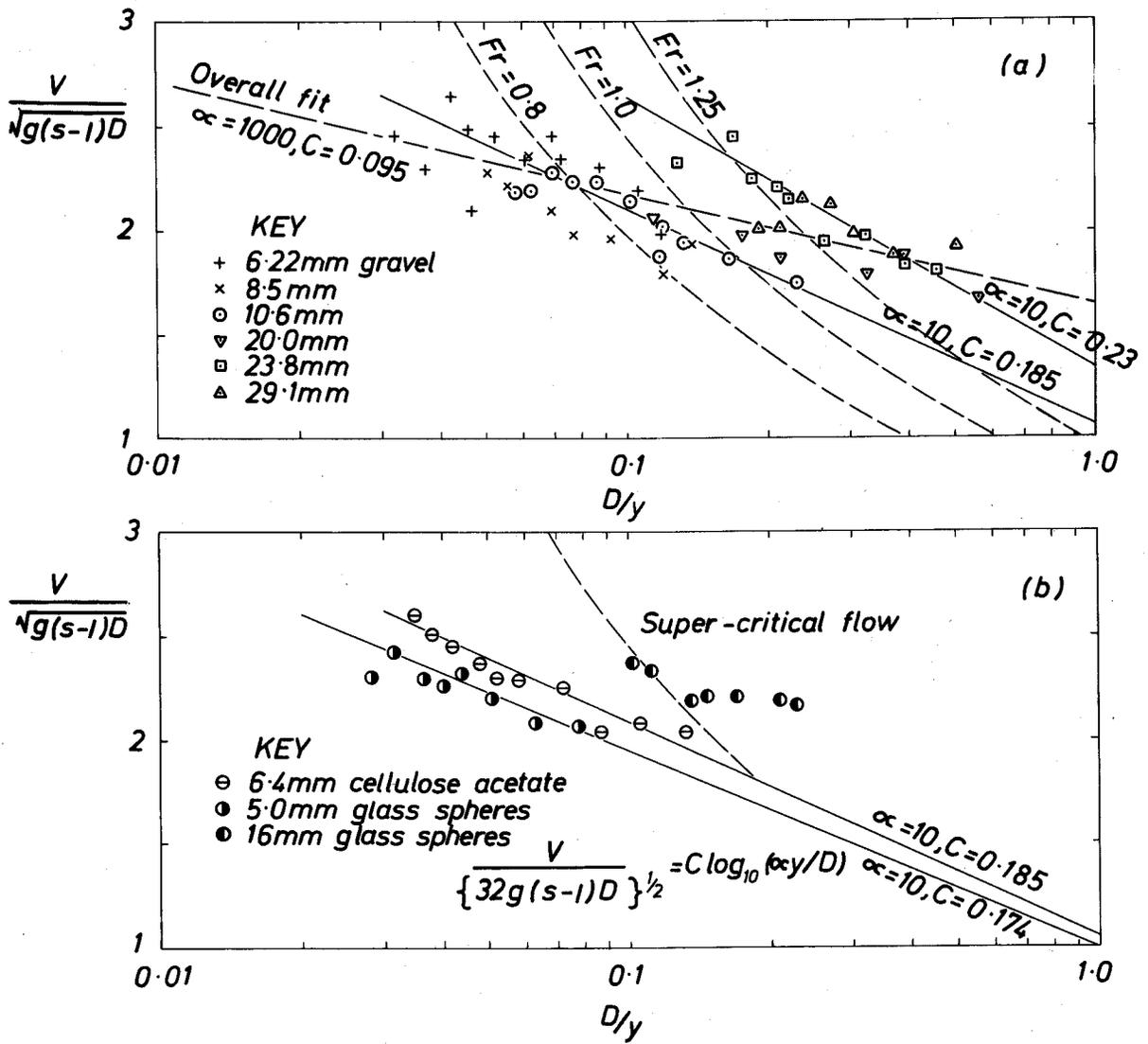
FIG 2. EVALUATION OF COEFFICIENT  $\alpha$  FROM INITIAL MOTION OF COARSE SEDIMENTS
