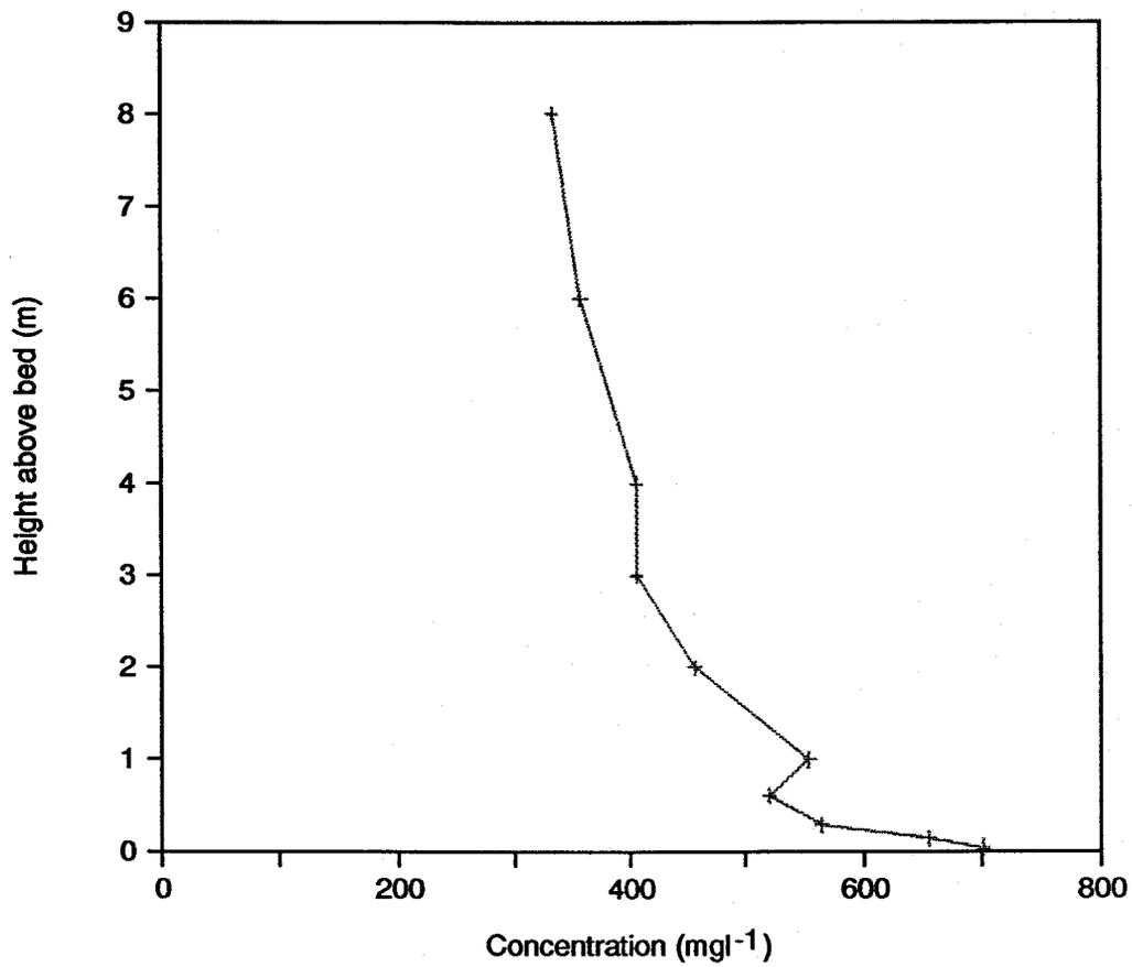
Fig 1 Example of suspended sediment concentration profile
