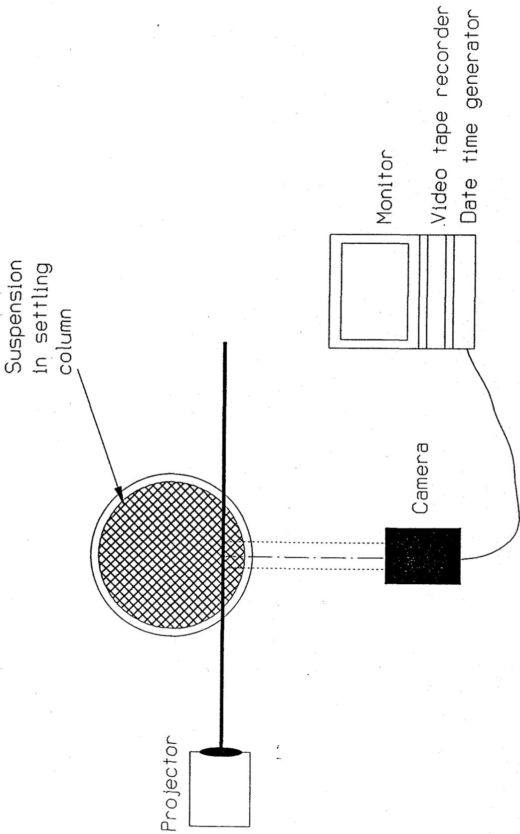
Fig 1 Apparatus for filming settling flocs.
