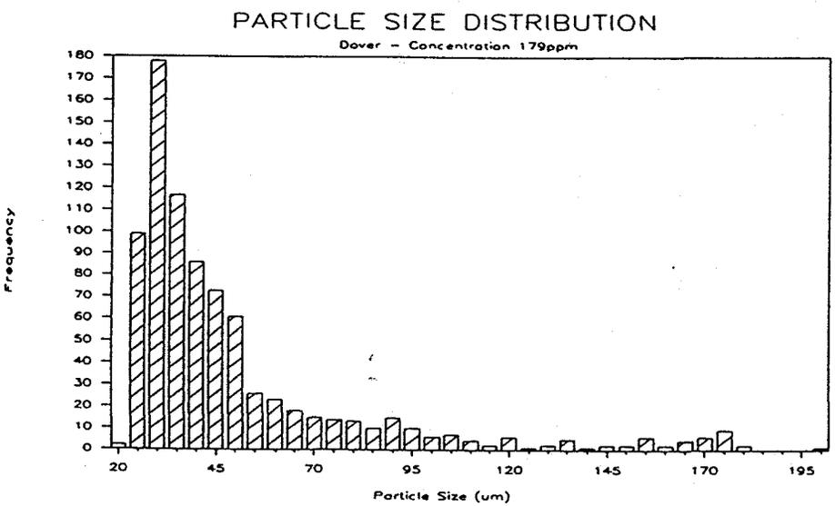
Fig 23 Effect of concentration on floc size distributions for Dover Harbour
