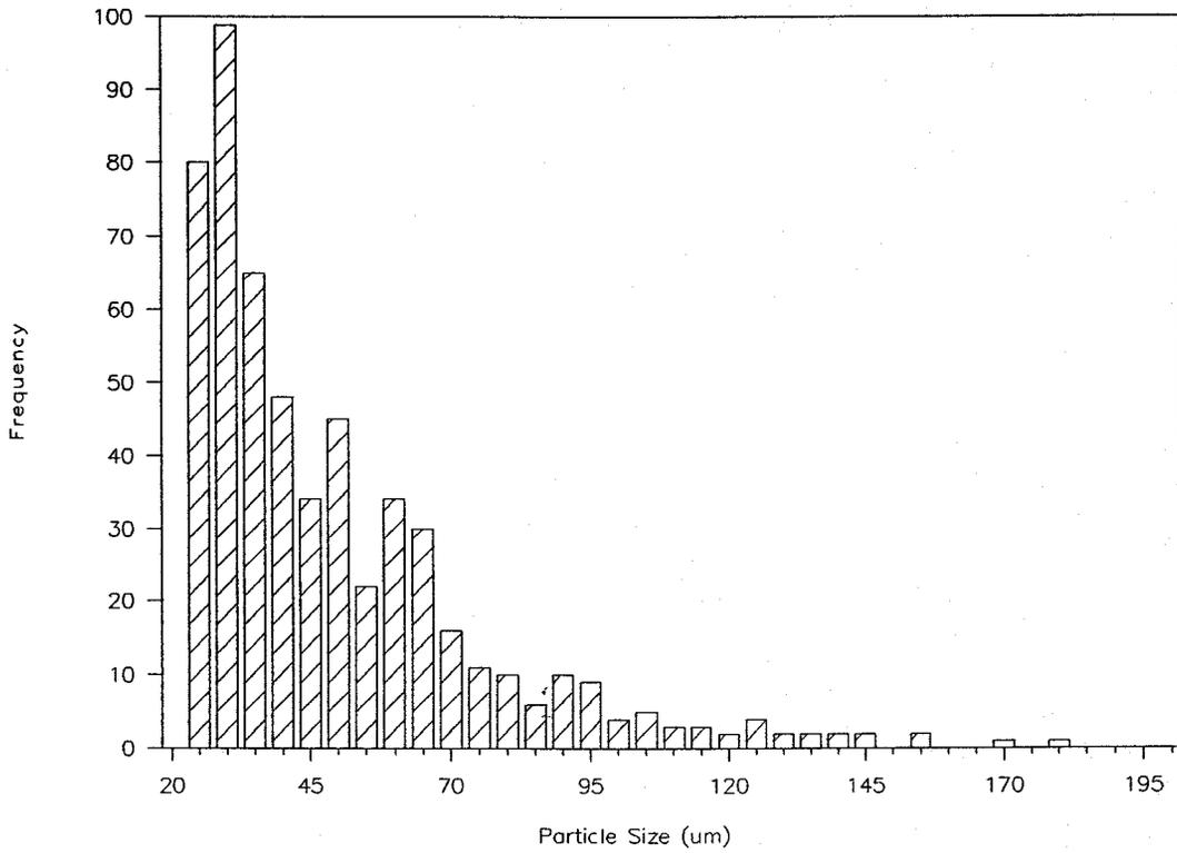
Fig 9 Effect of time on floc size distribution
