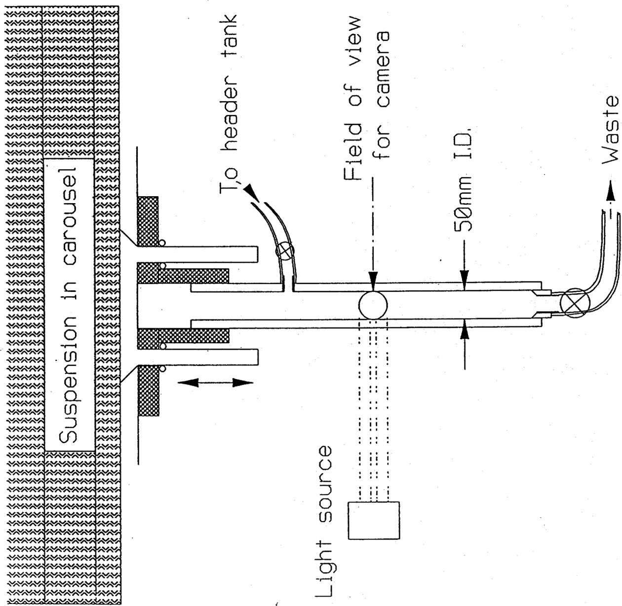
Fig 7. Sampling system for base of carousel
