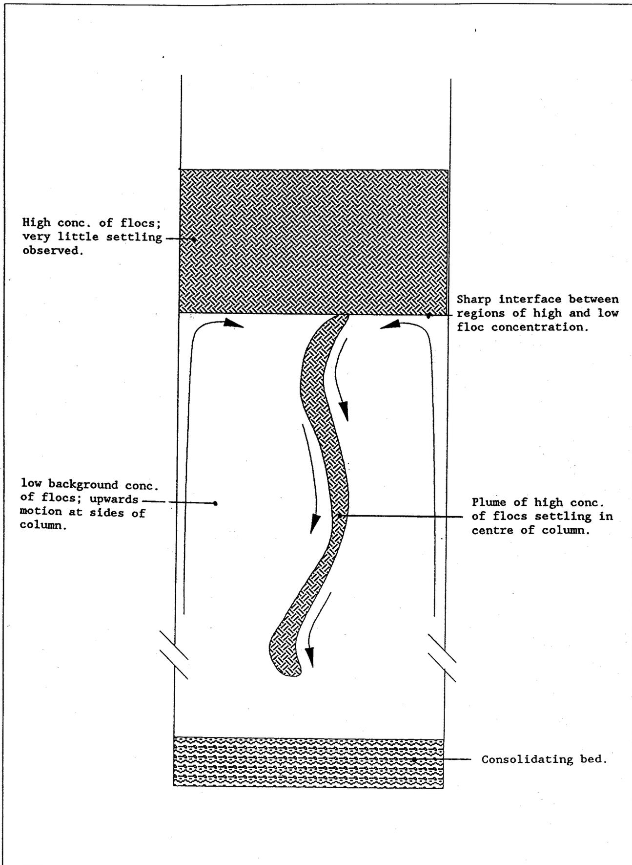
Fig 16 Schematic representation of interface and circulation after 25 minutes of settling
