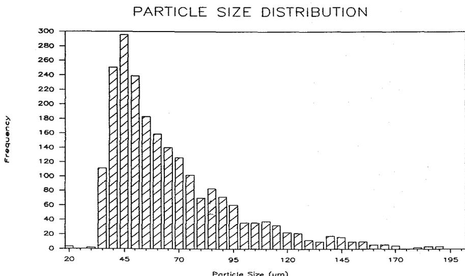
Fig 25 Effect of concentration on floc size distributions for Mersey Estuary
