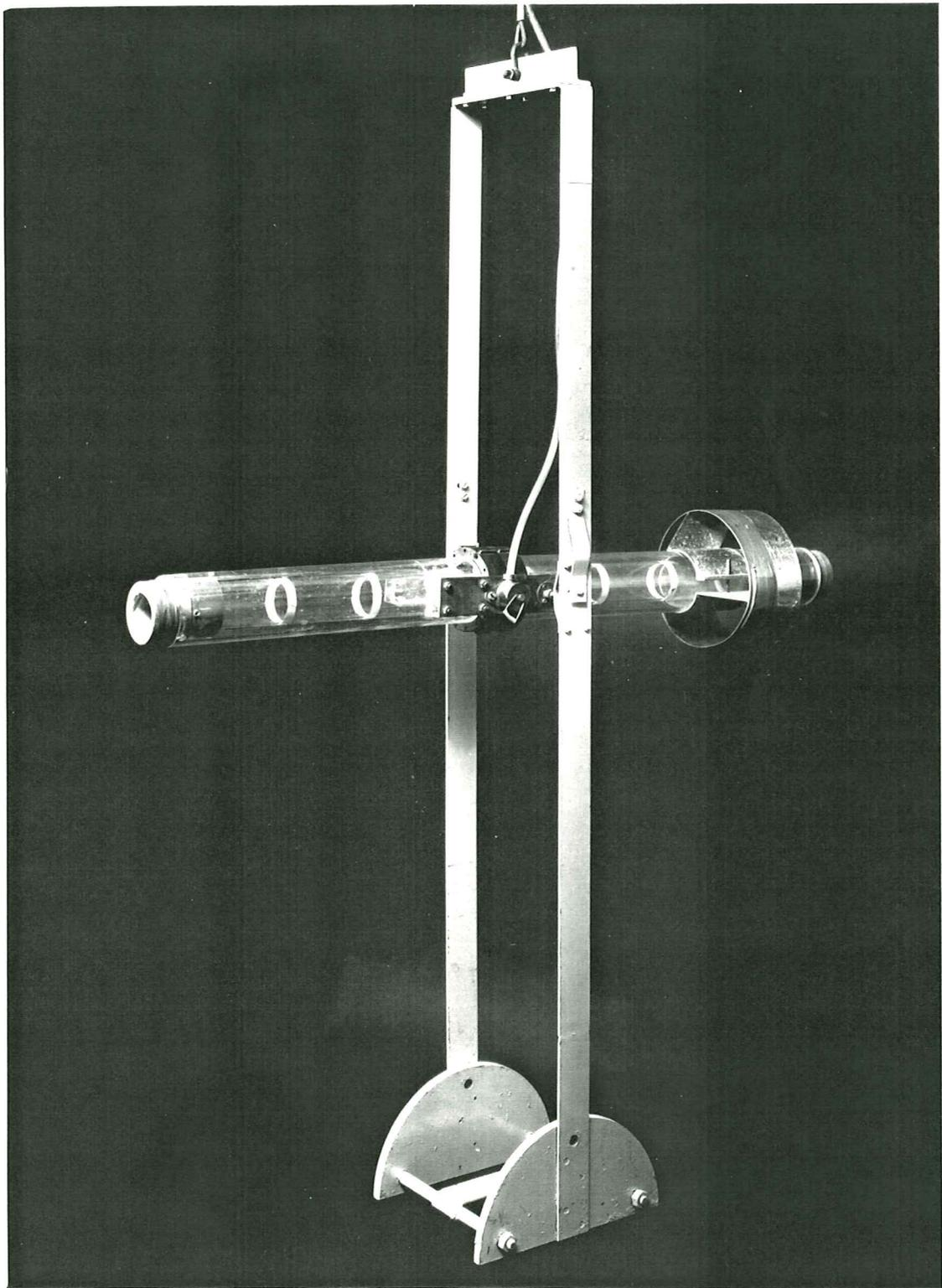
Plate 1 Owen tube in submerged position
