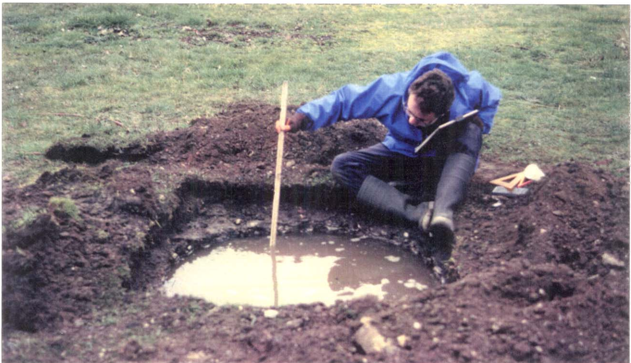
Plate 4 Soakage test pit 1.2m diameter, field experiment
