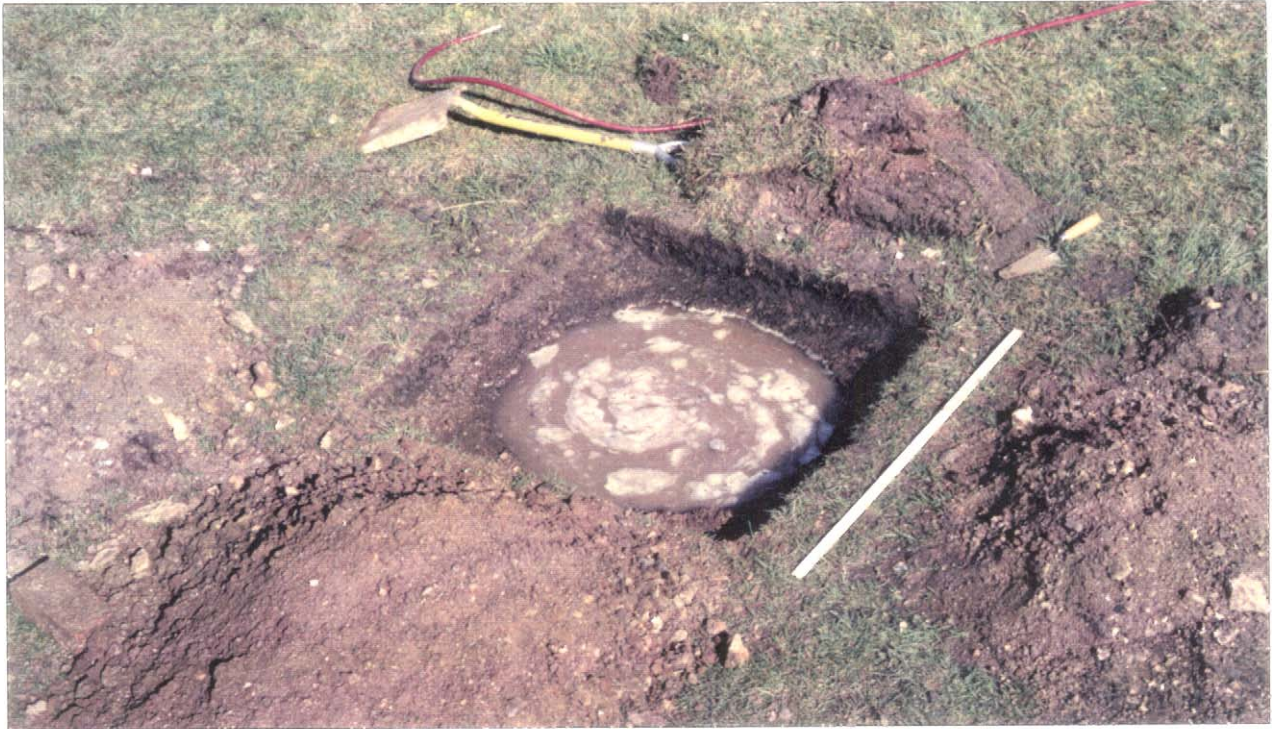
Plate 3 Soakage test pit 0.8m diameter, field experiment
