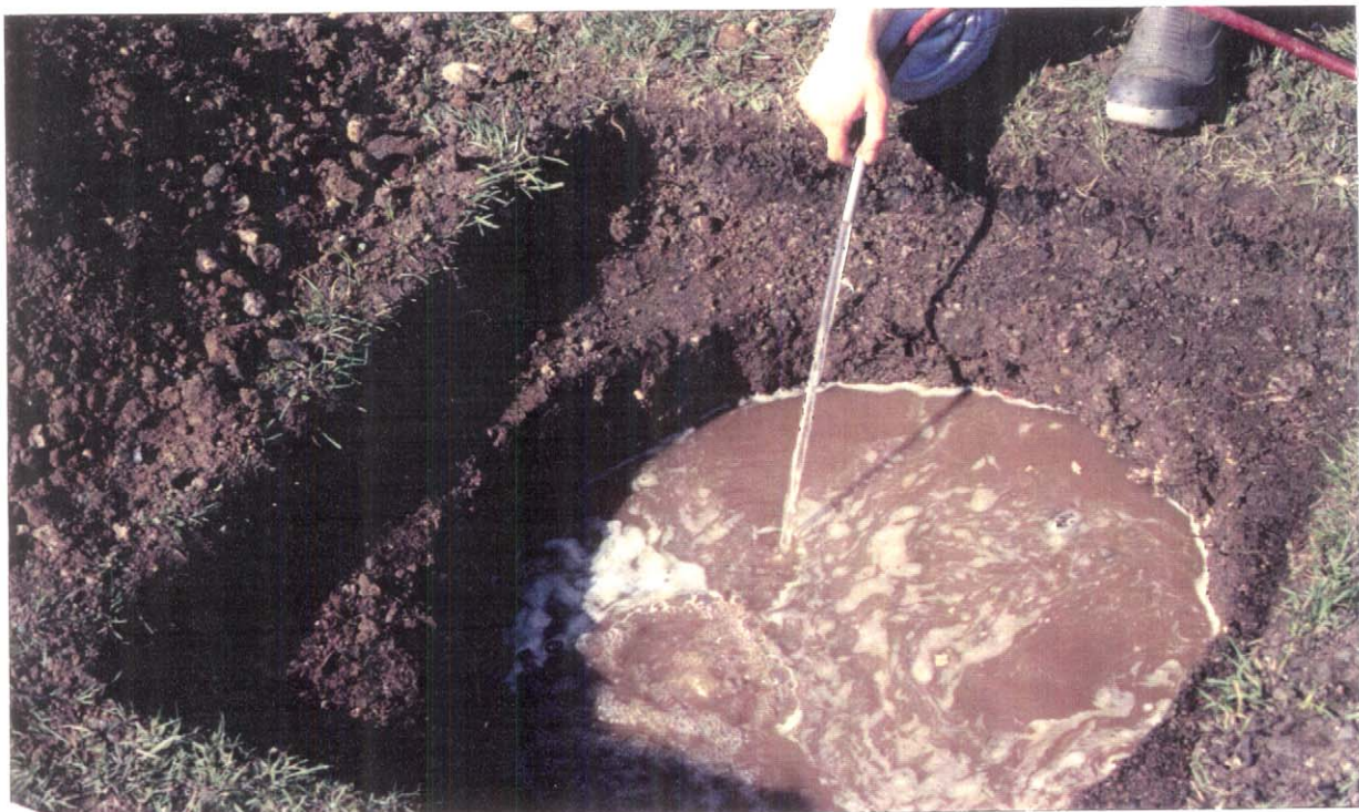
Plate 2 Soakage test pit 0.5m diameter, field experiment
