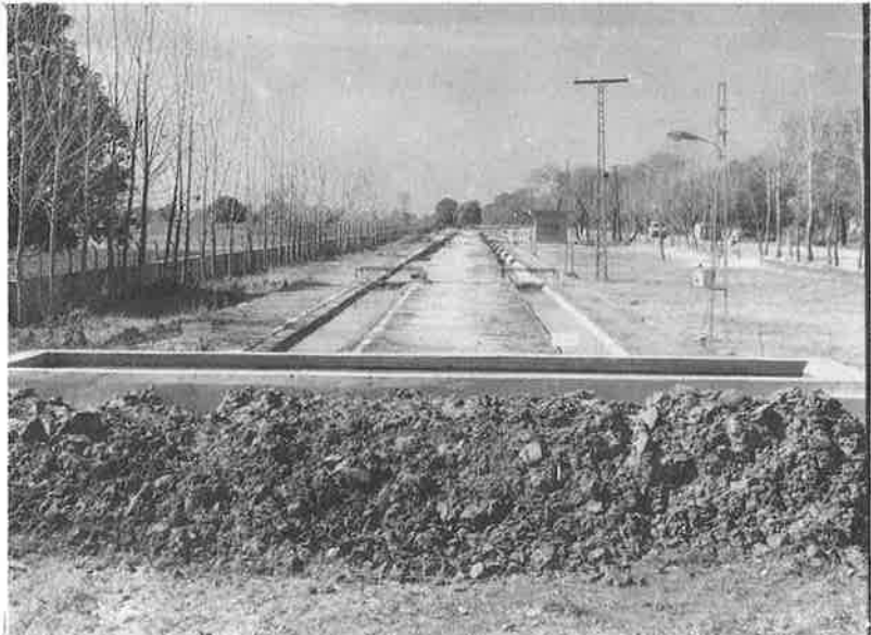
Photo 3. Permanent experimental set up of water channels for testing various lining materials at Niaz Beg Research Station, Lahore.
