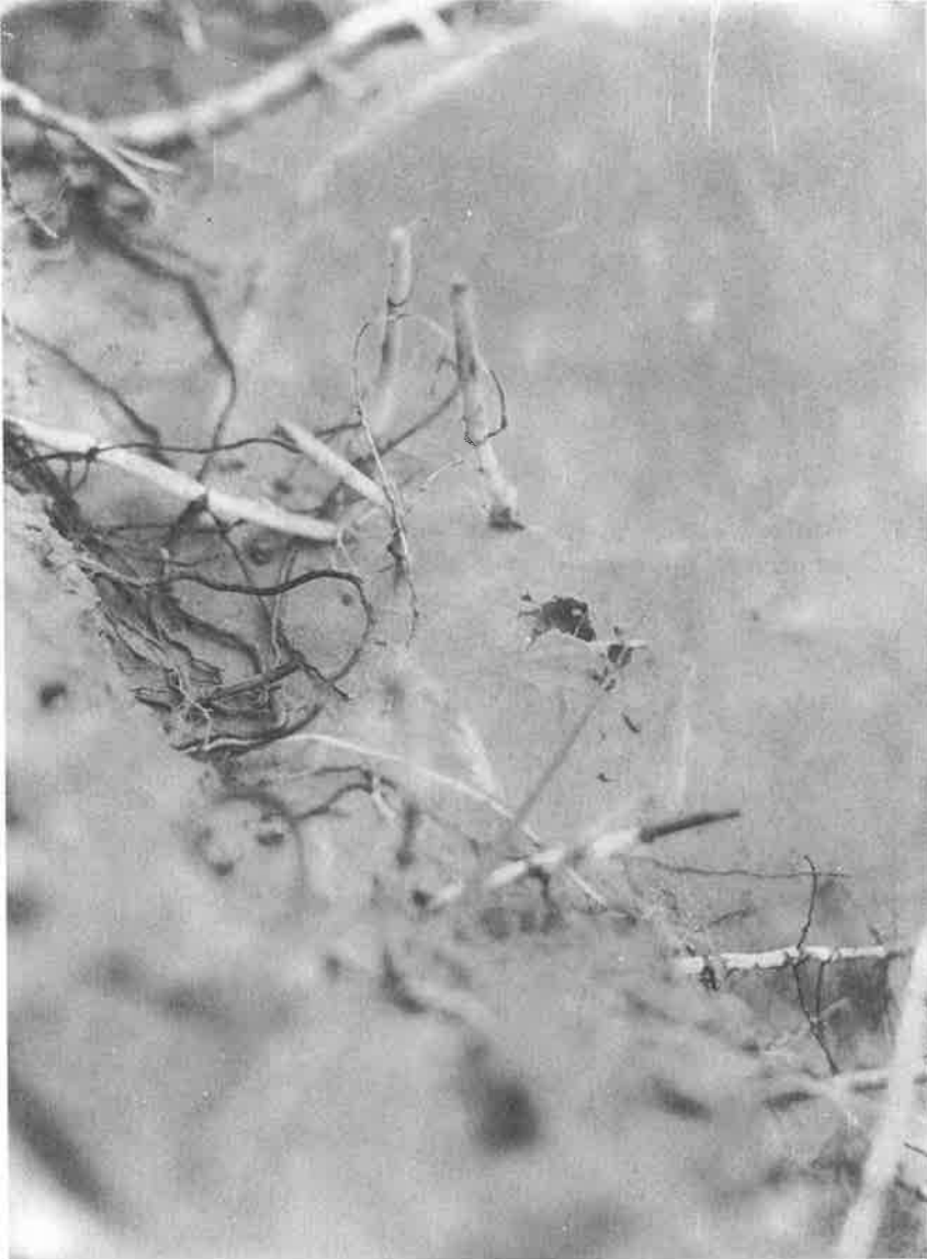
Photo 1. Weed roots puncturing the polyethylene sheet, observed after removing the soil cover (Field study).
