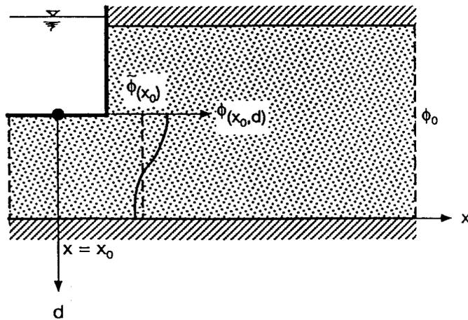
Figure 4.3 Piezometric head under a river bed.
