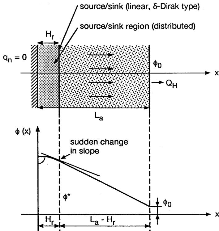
Fig.4.2. Top view of an aquifer and piezometric head for the 2D-horizontal flow model.
