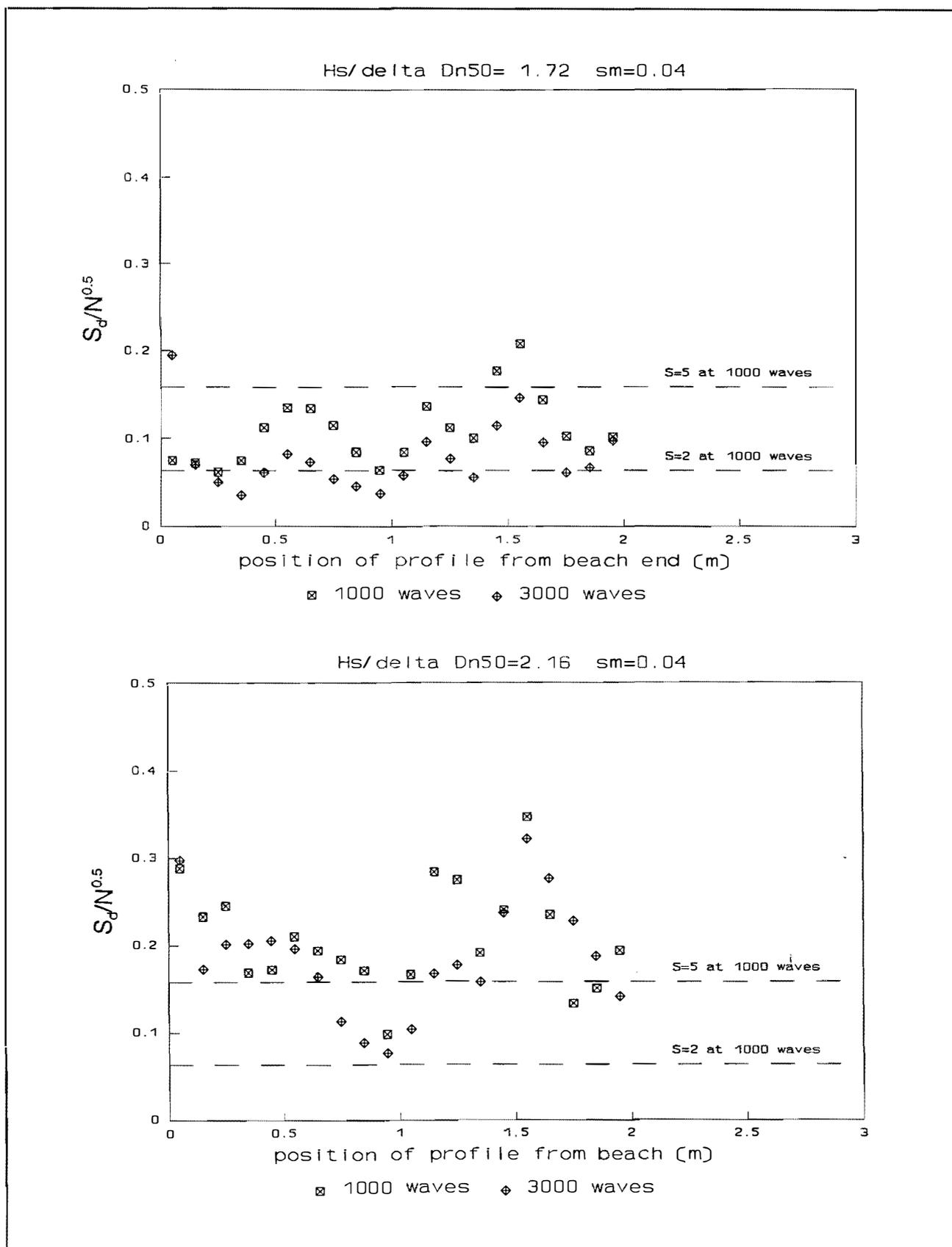
Figure 11 Damage along Type 1 groyne,  $s_m=0.04$ ,  $H_s/\Delta D_{n50}=1.72$ , and  $H_s/\Delta D_{n50}=2.16$
