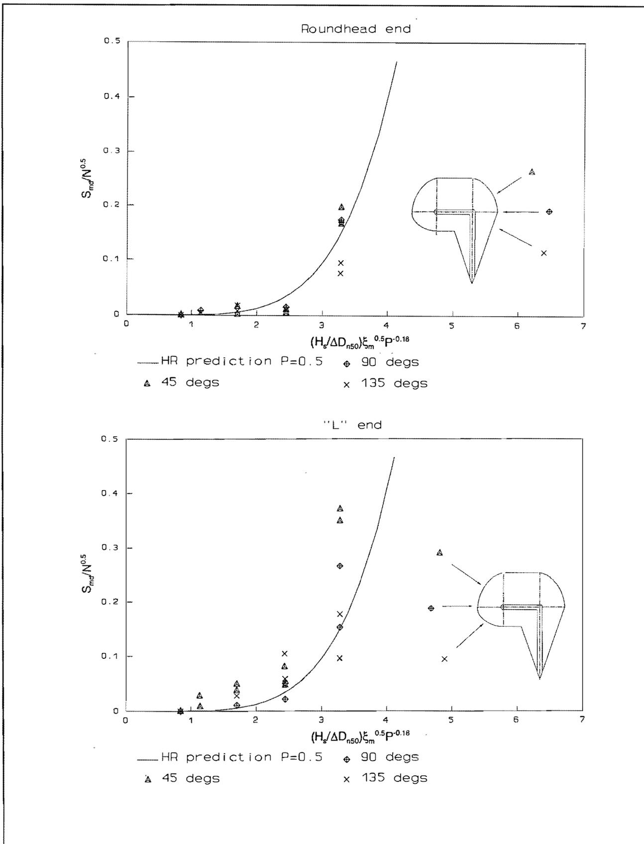
**Figure 8** Damage to curved parts of L-shaped groyne
