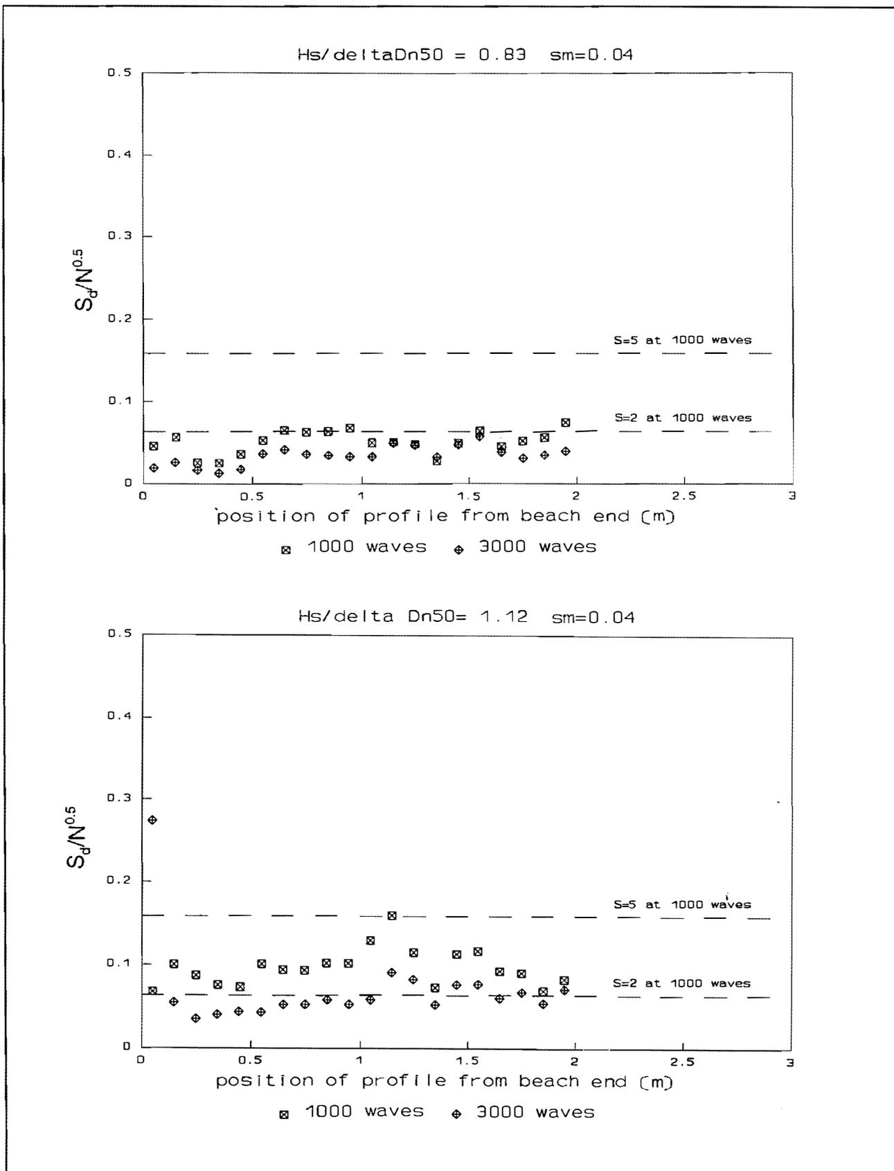
Figure 10 Damage along Type 1 groyne,  $s_m=0.04$ ,  $H_s/\Delta D_{n50}=0.83$ , and  $H_s/\Delta D_{n50}=1.12$
