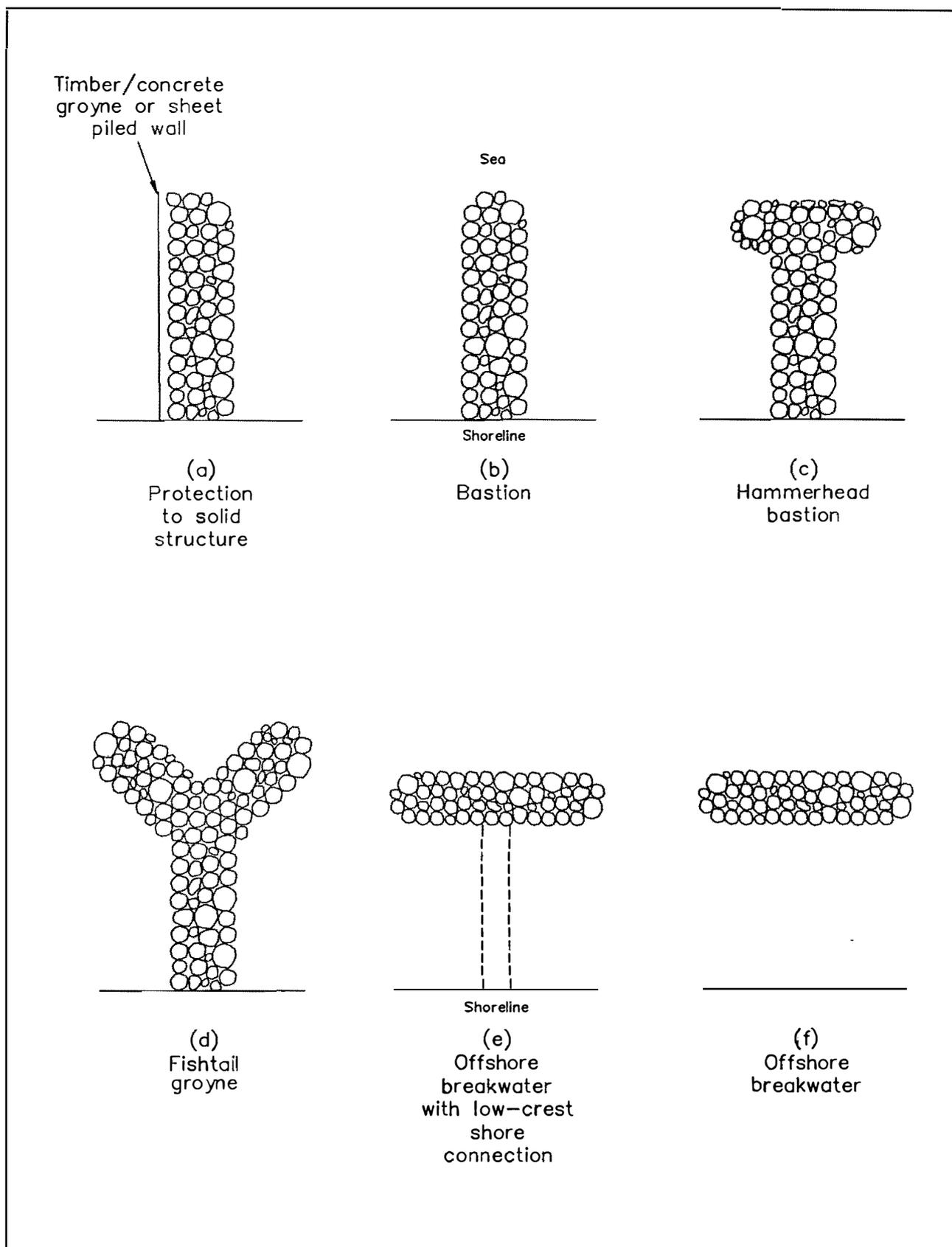
**Figure 1** Types of beach control structures from simple groynes to near-shore breakwaters
