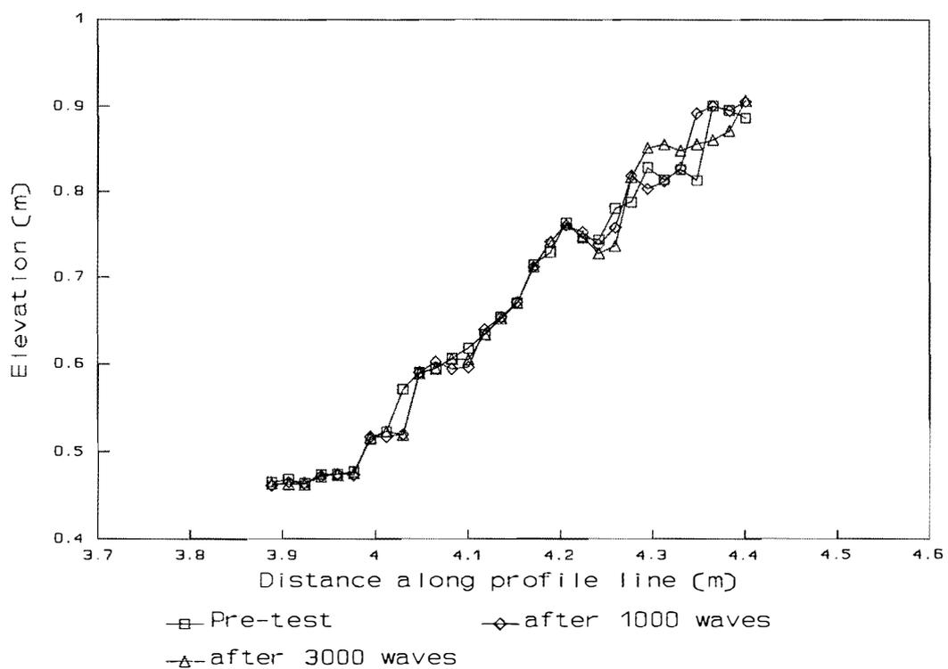
Figure 6 Example damage on Type 2 groyne
