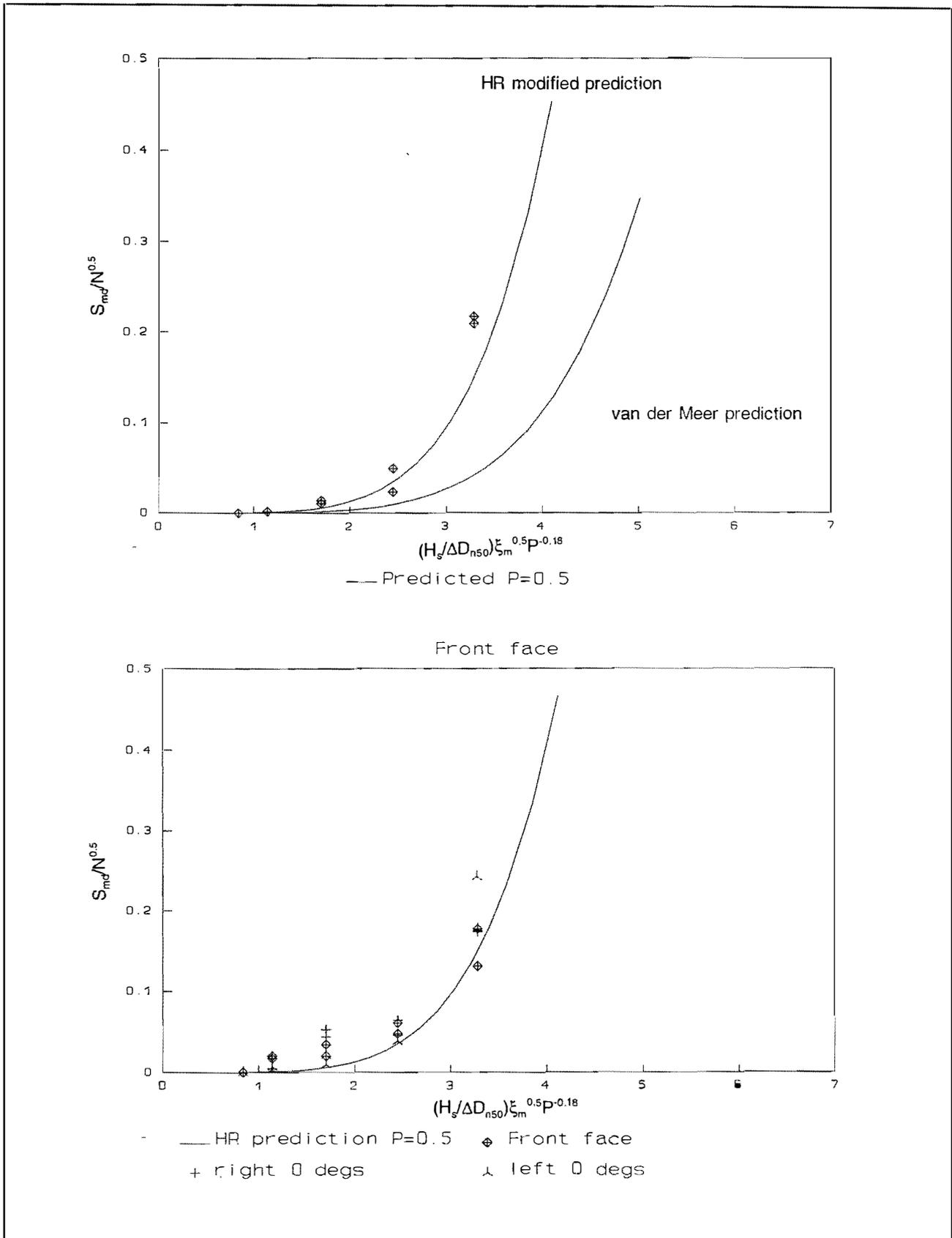
Figure 7 Damage to 1:2 sea wall and front face of L-shaped groyne
