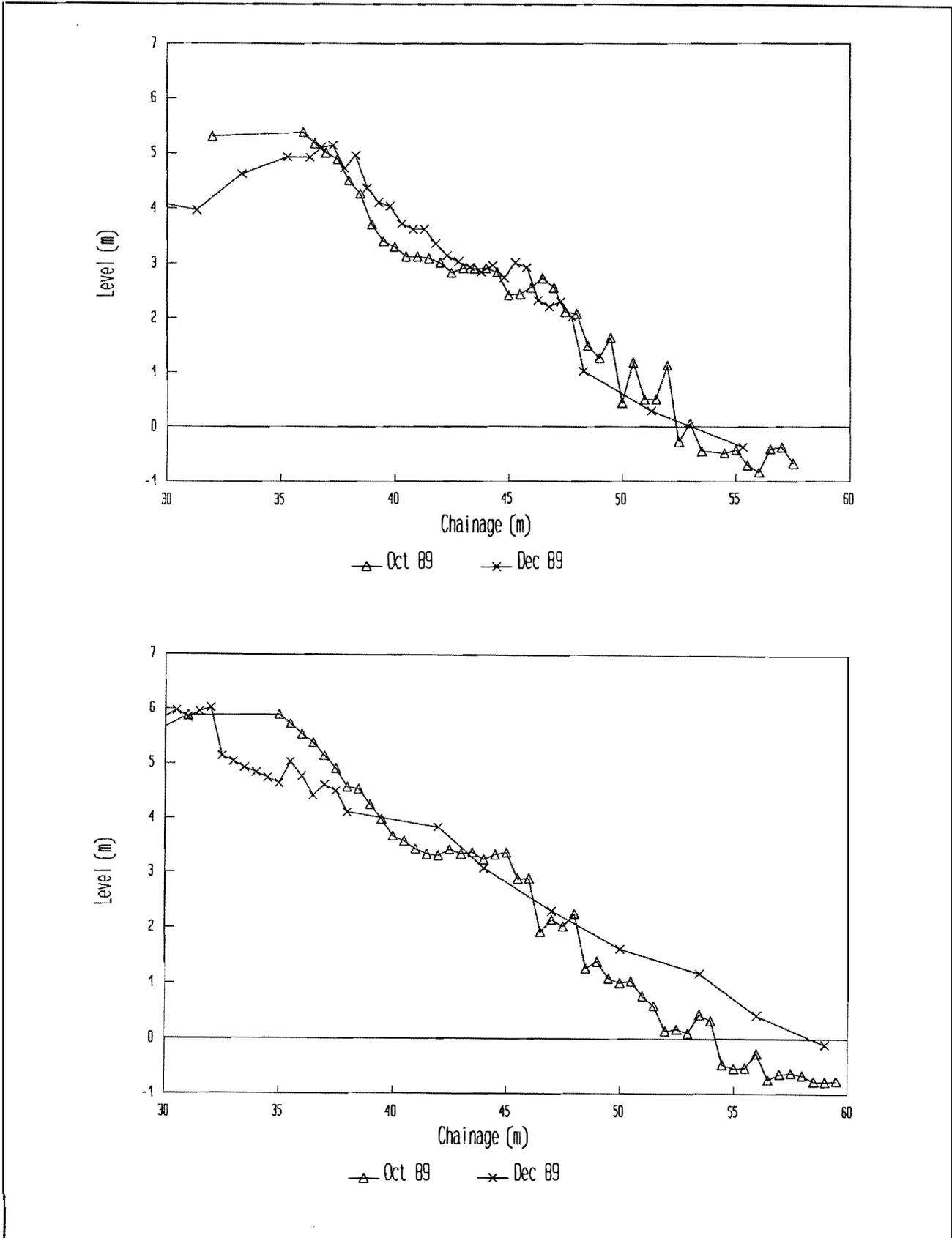
Figure 12 Damage to rock revetment at Hurst Spit, profiles 2 and 4
