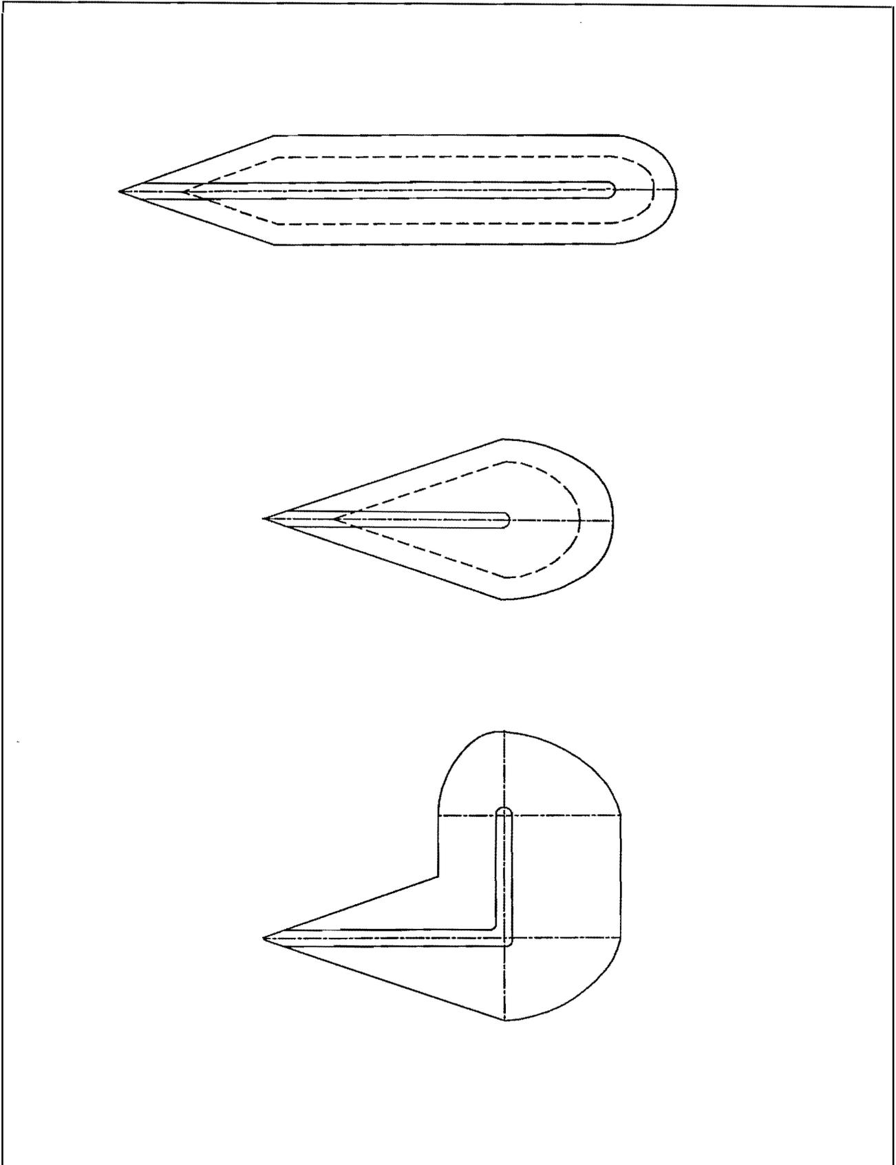
**Figure 4** Type 1, Type 2, and L-shaped groynes, plan
