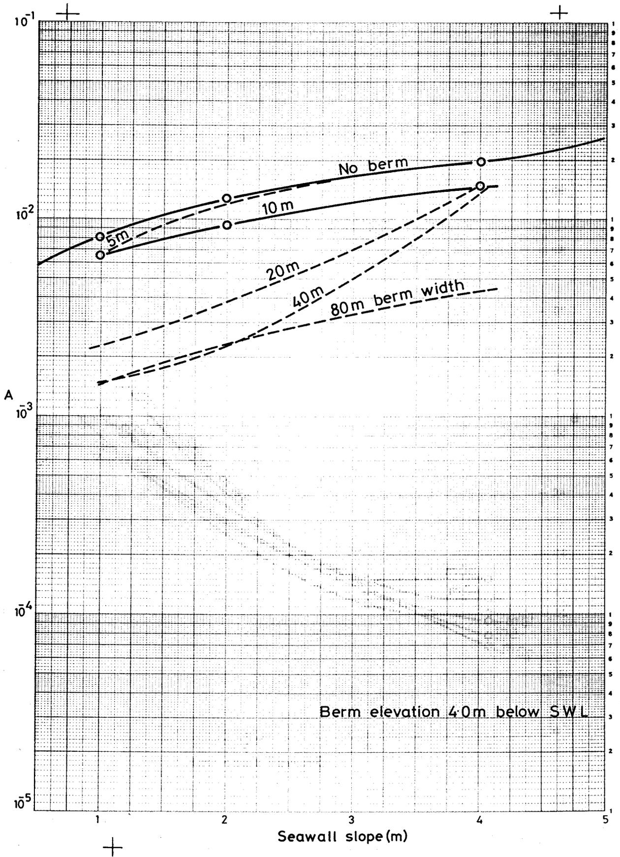
Coefficients A and B: berm elevation at 4m below SWL
