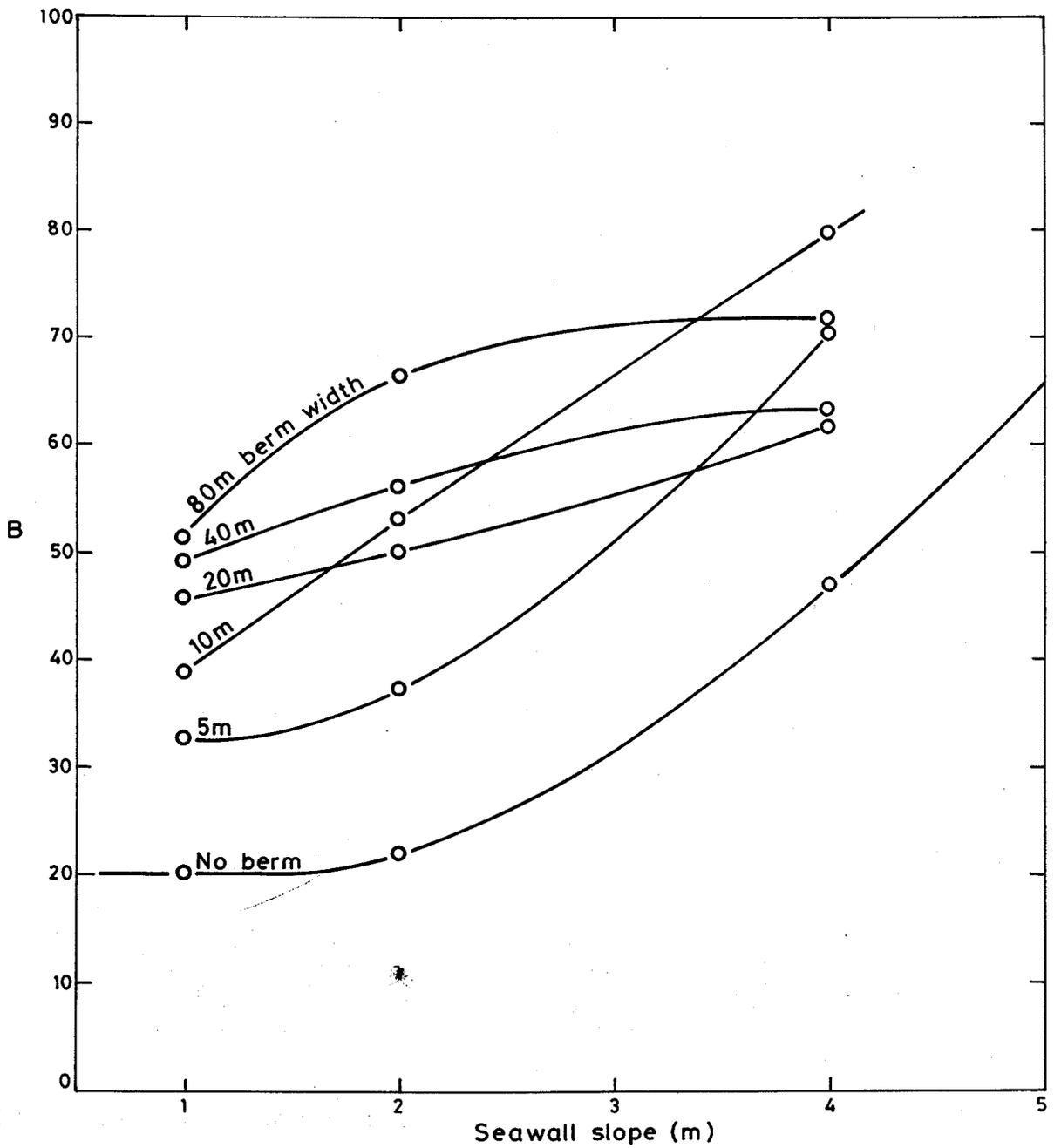
Coefficients A and B : berm elevation at 1m below SWL
