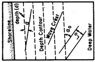
Simple wave refraction and shoaling
