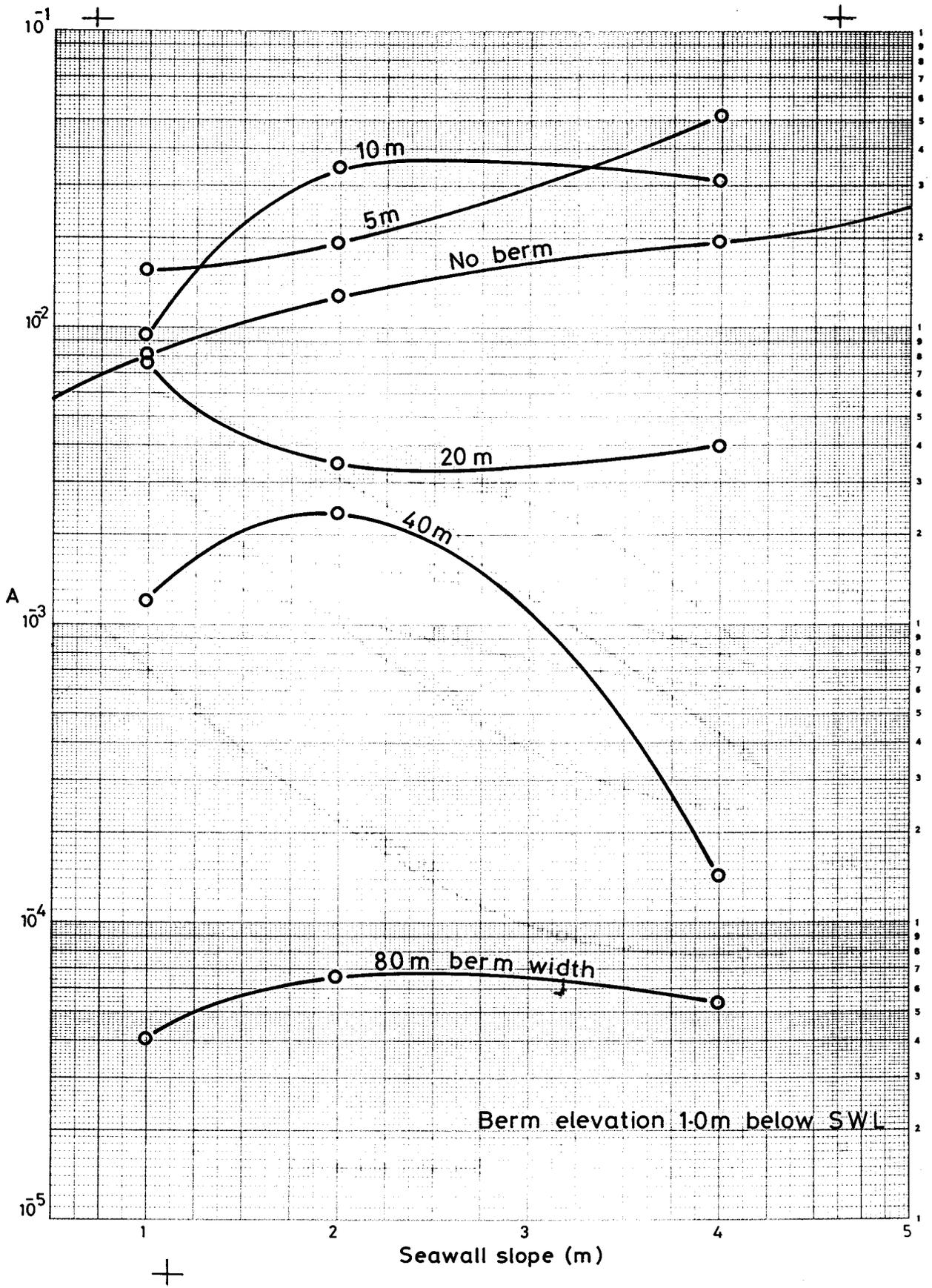
Coefficients A and B : berm elevation at 1m below SWL
