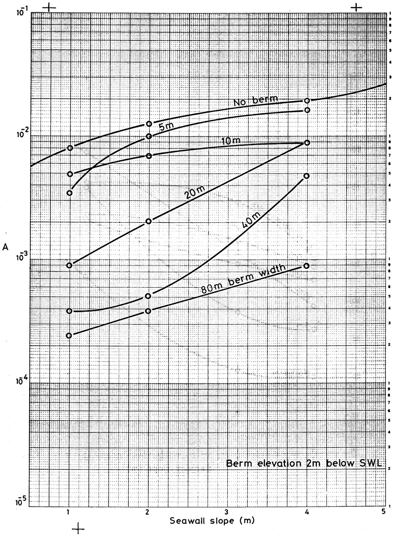
Coefficients A and B : berm elevation at 2m below SWL
