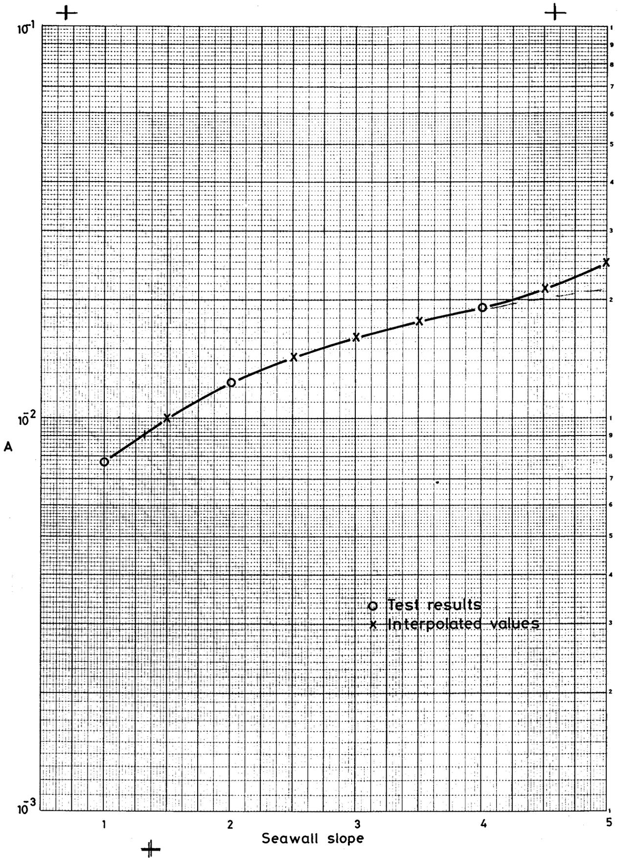
Coefficients A and B for simple seawalls
