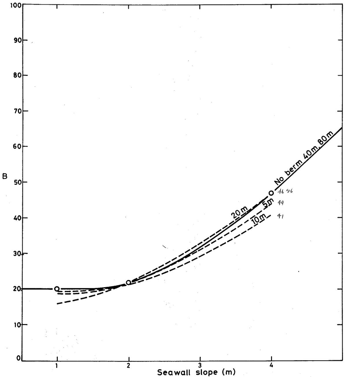
Coefficients A and B : berm elevation at 4m below SWL
