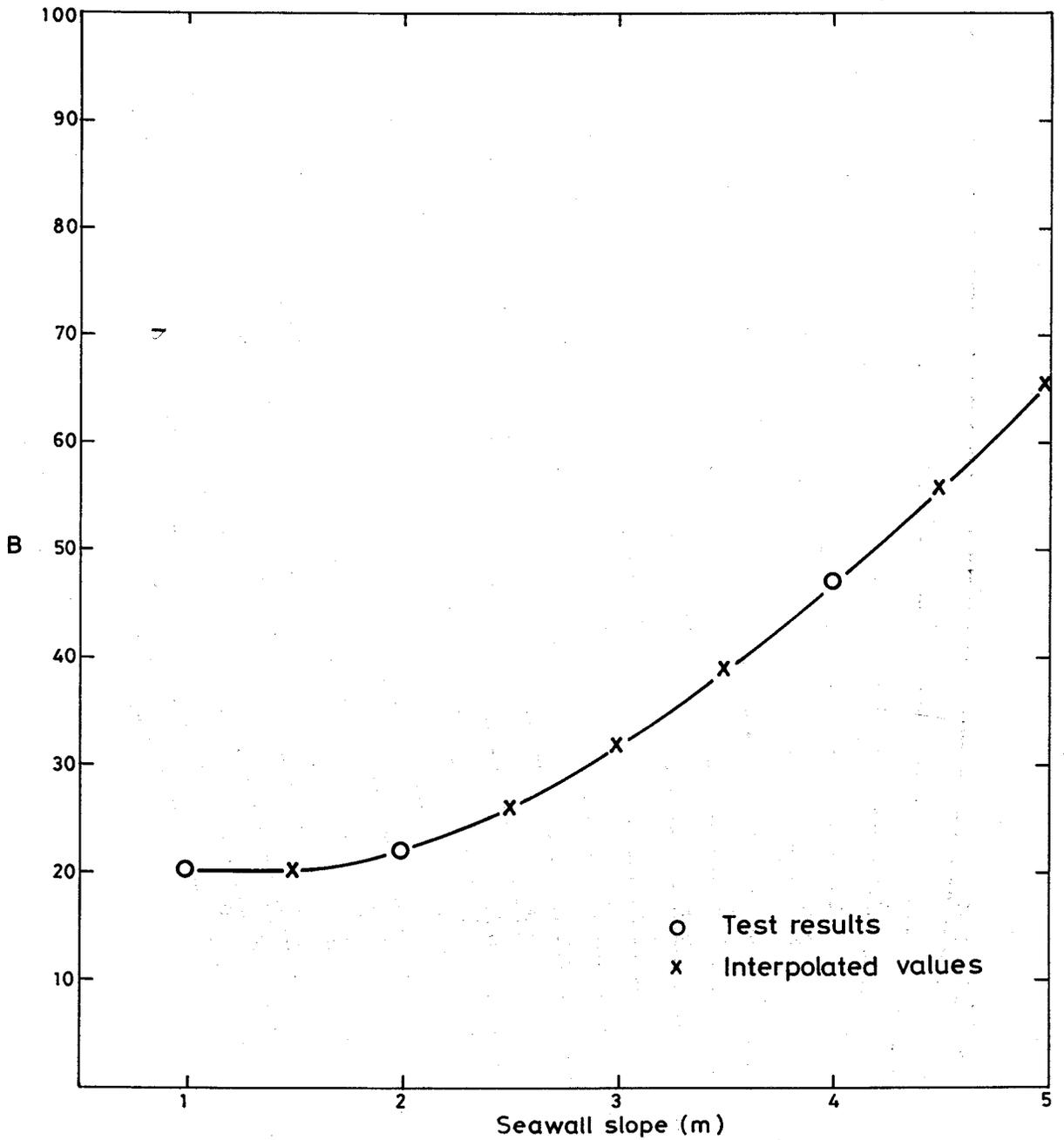
Coefficients A and B for simple seawalls
