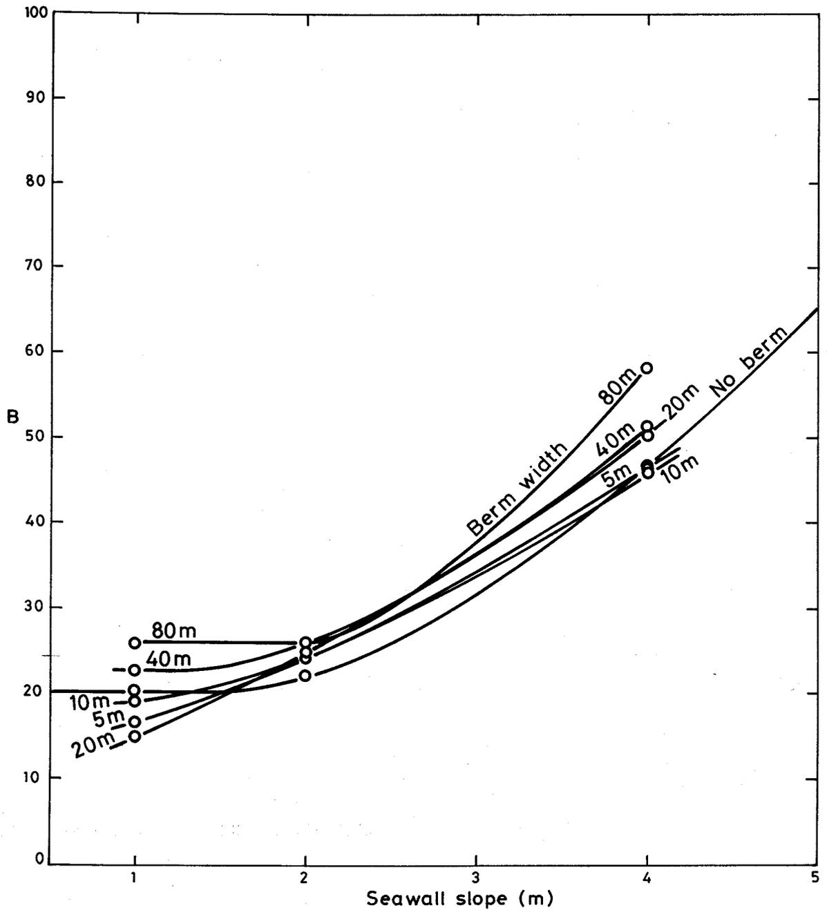
Coefficients A and B : berm elevation at 2m below SWL
