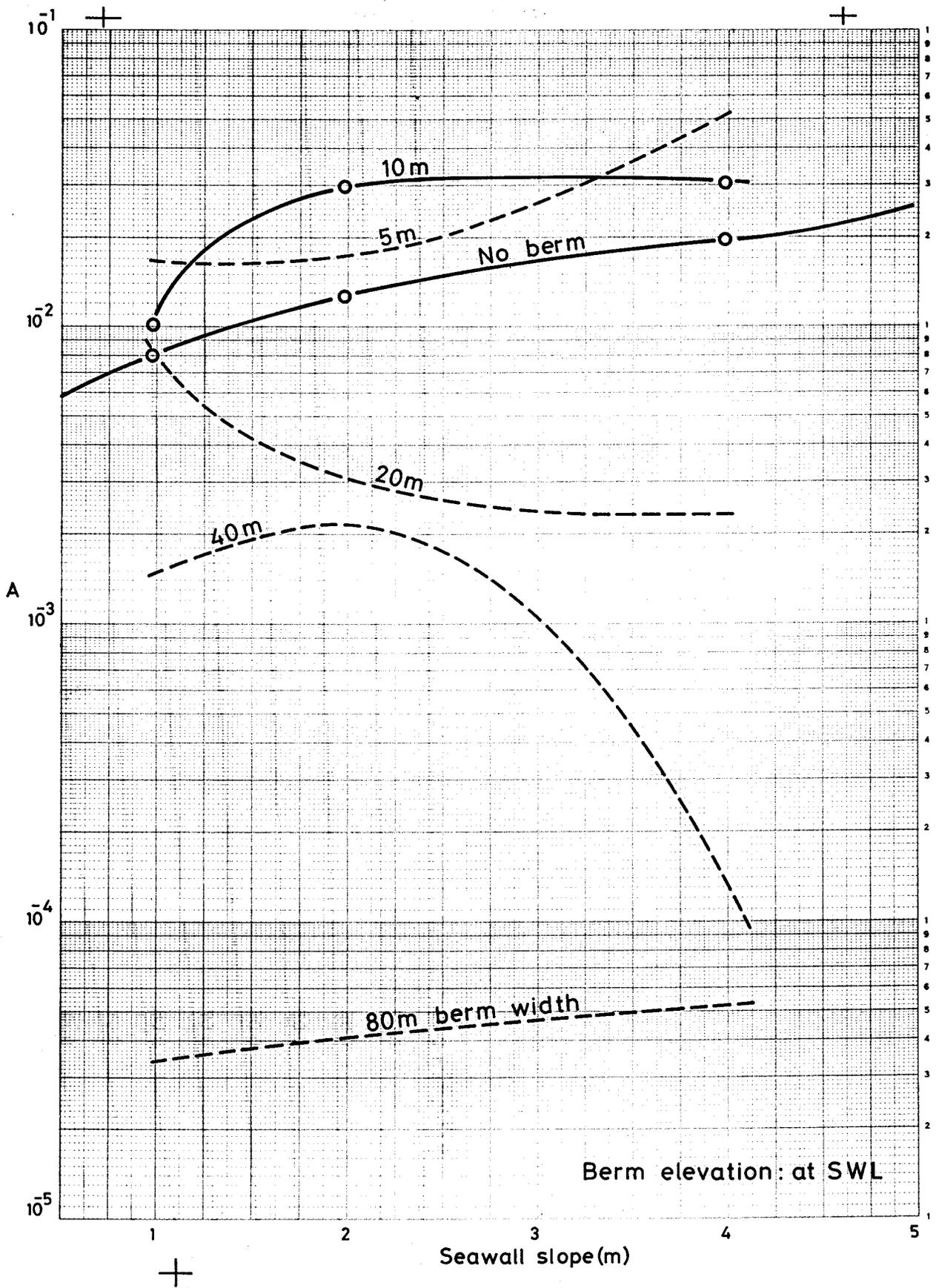
Coefficients A and B : berm elevation at SWL
