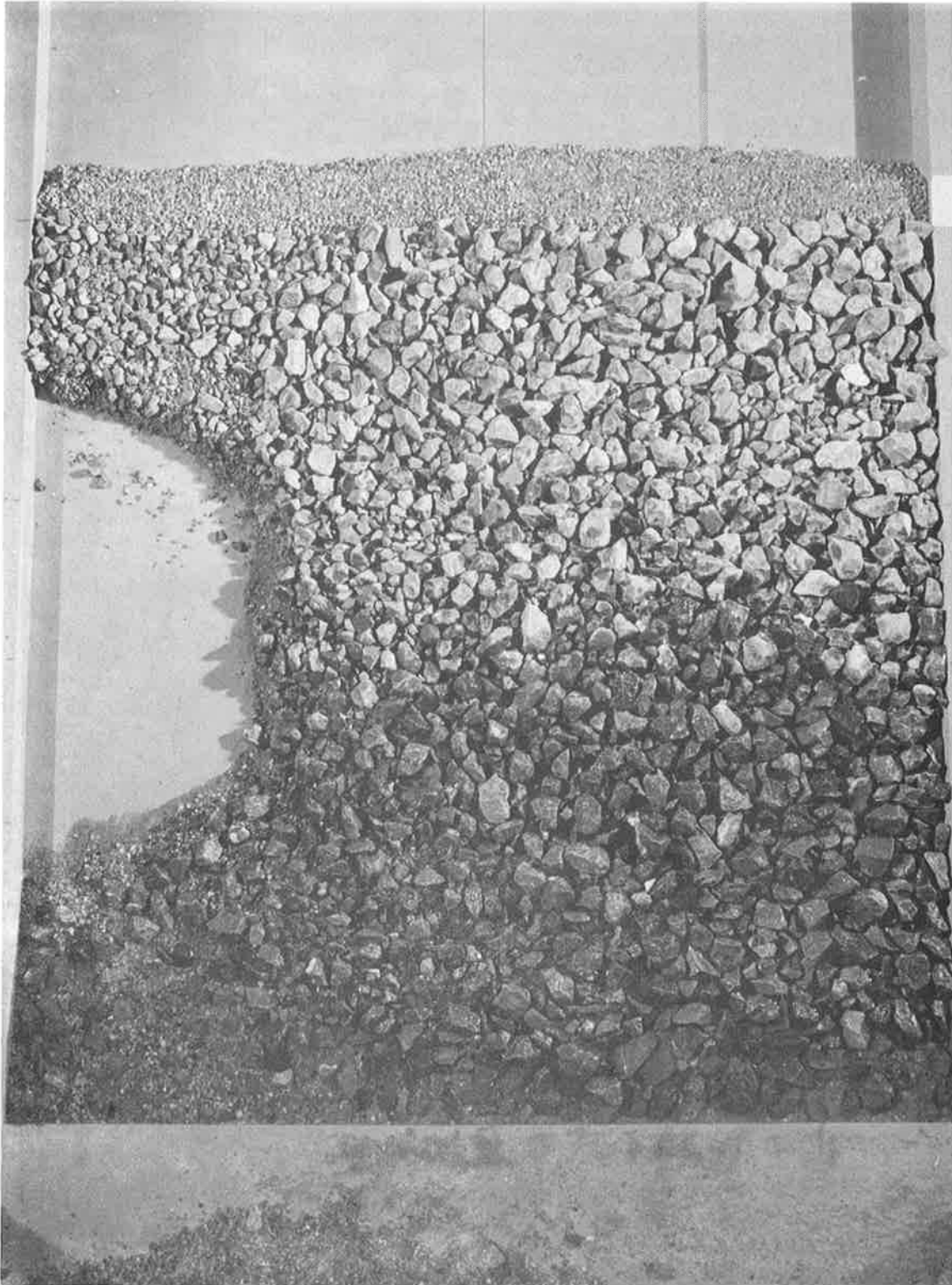
Plate 14 Progress of damage during storm 2 — test run 2
