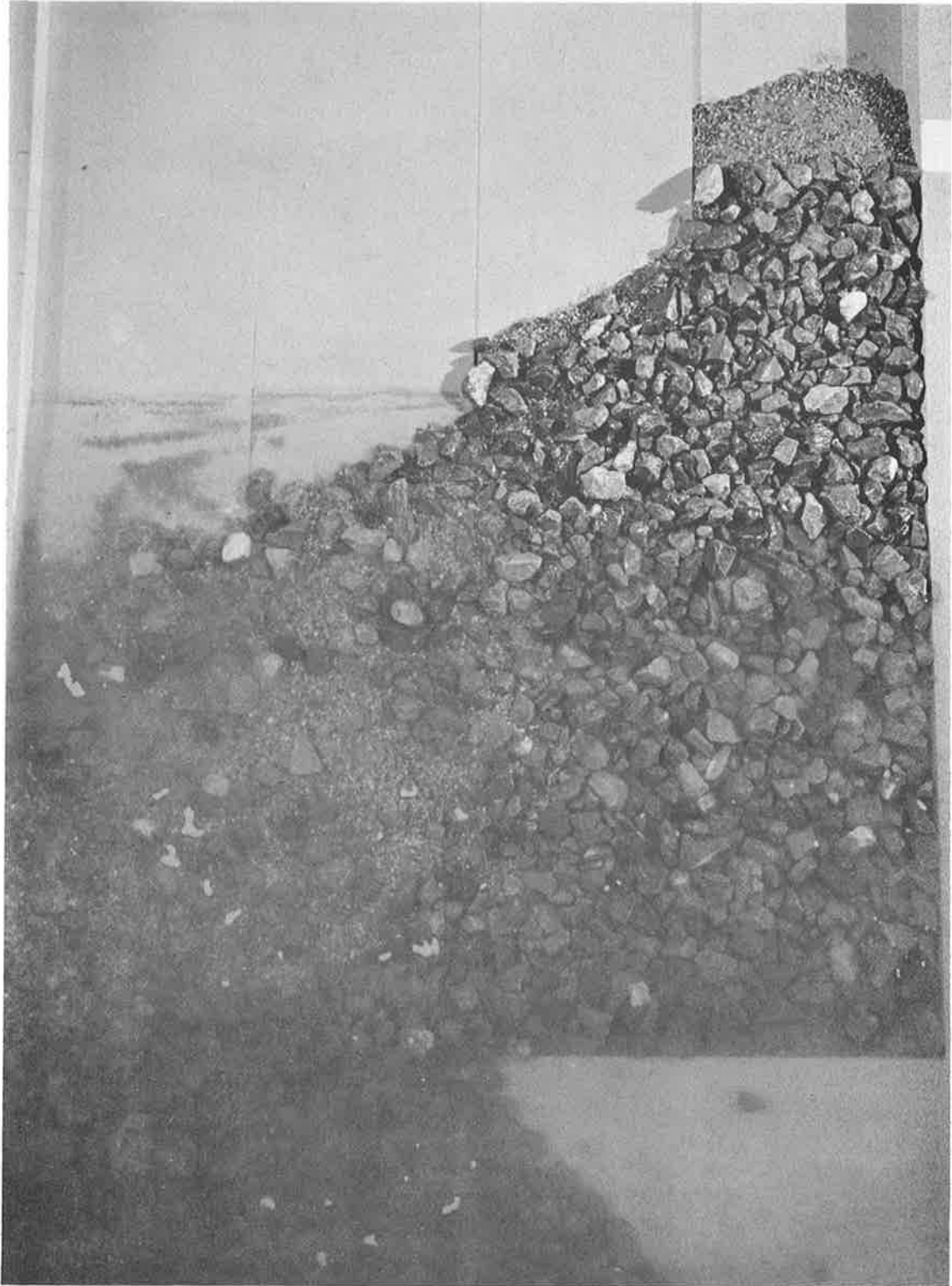
Plate 14 Progress of damage during storm 2 — test run 2
