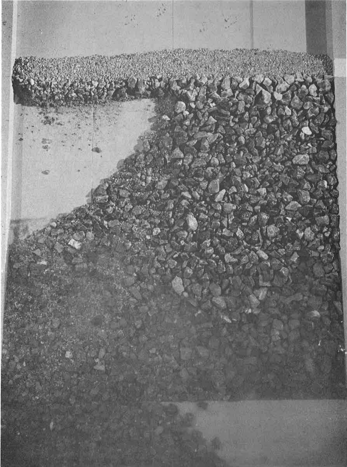
Plate 14 Progress of damage during storm 2 — test run 2
