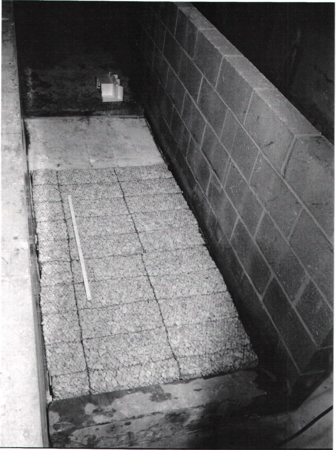
**Plate 2 Reno mattresses placed in the flume**
