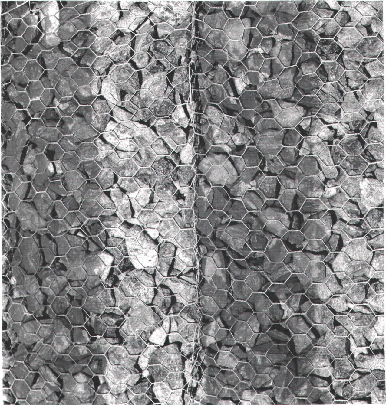
**Plate 4 Reno mattress after a test showing movement of stone**
