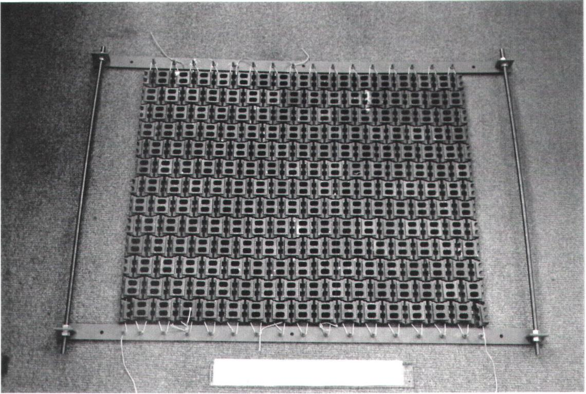
Plate 5 Cabled blocks with frame
