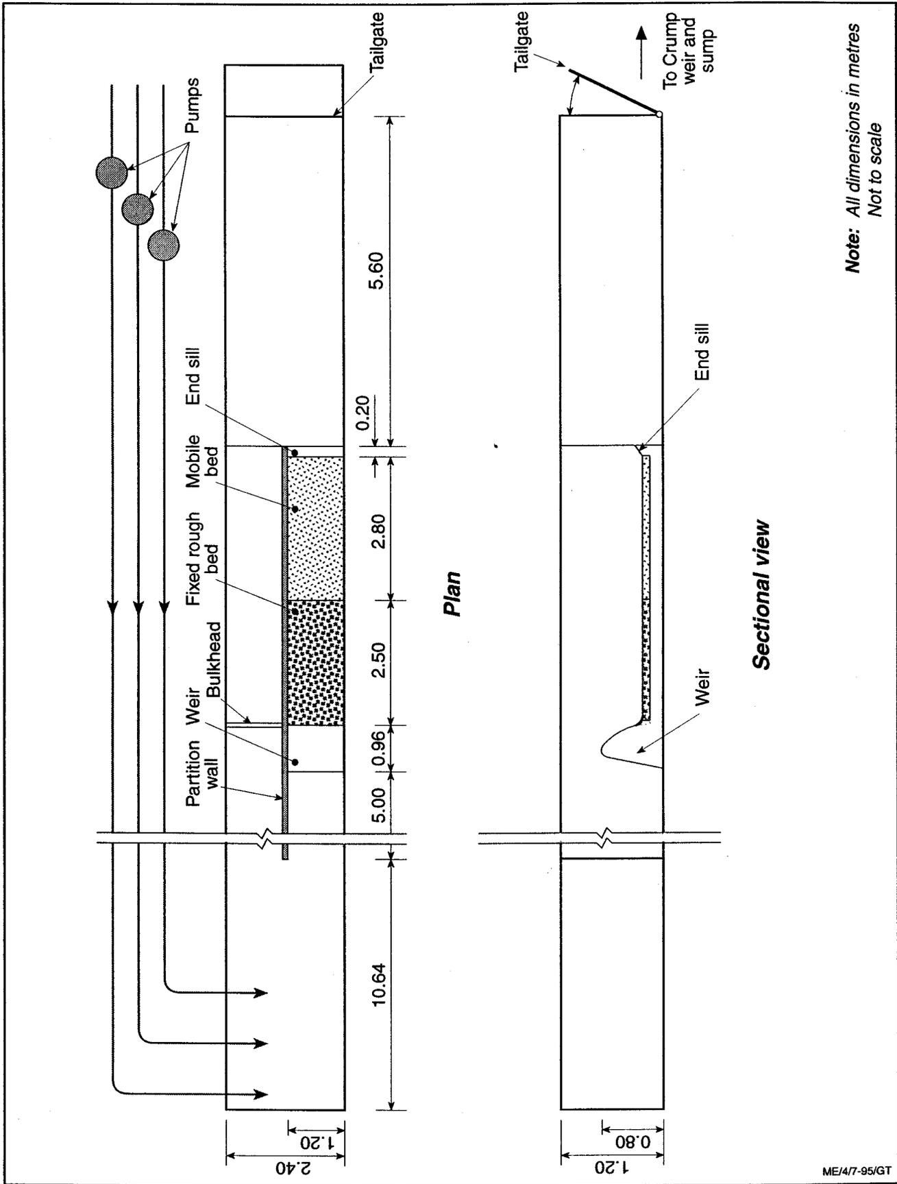
**Figure 4 General layout of test rig**
