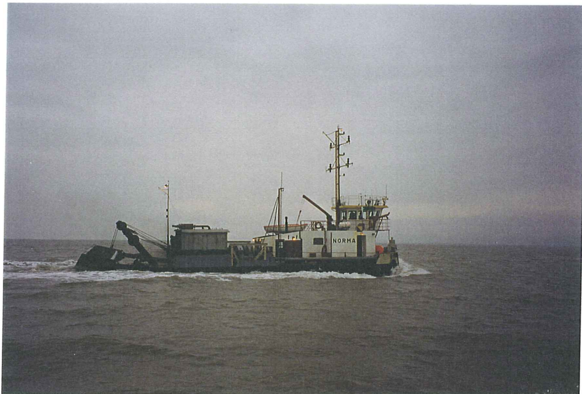
Plate 11 Plough 'Norma' operating in Lough Foyle, Northern Ireland
