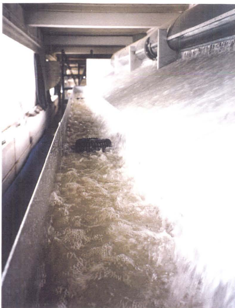
Plate 13 Test of Fullflow system at Q = 23.1 l/s
