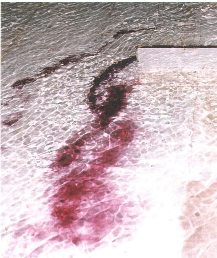
**Plate 5**      **Submerged groyne - Near bed flow**
