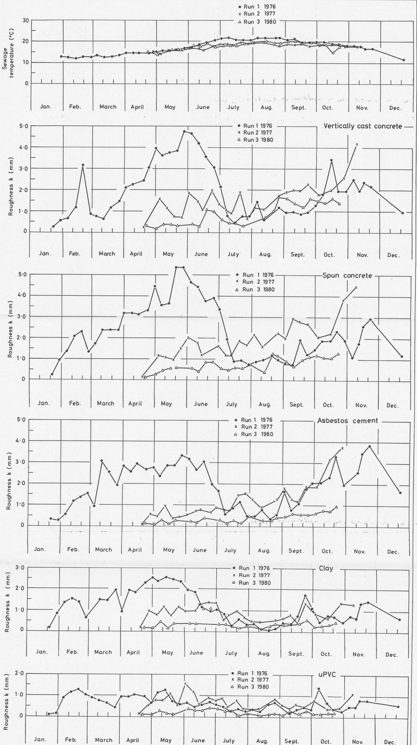
Variation of roughness in test pipes
