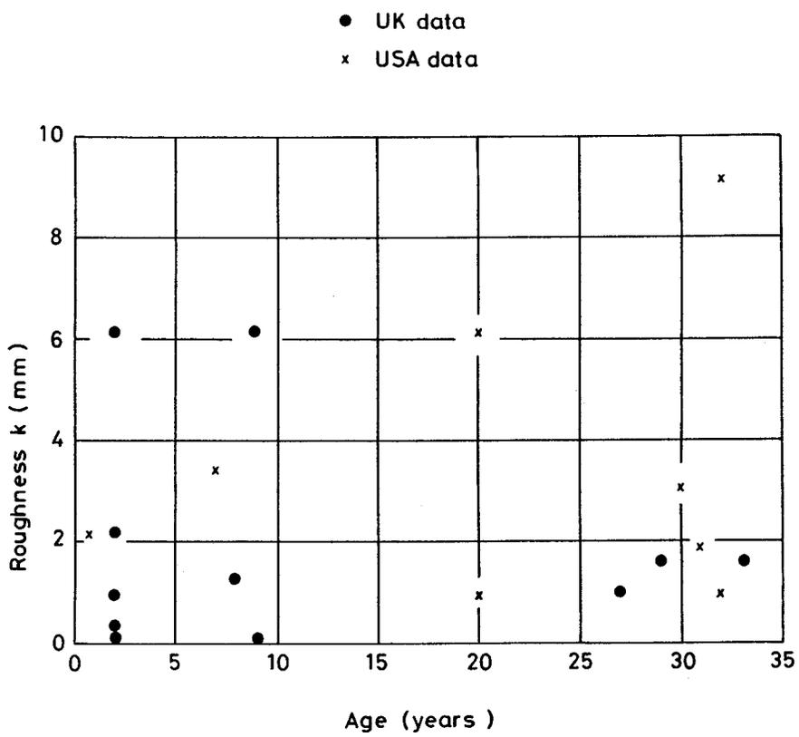
Fig 19 Roughness as a function of age in concrete sewers
