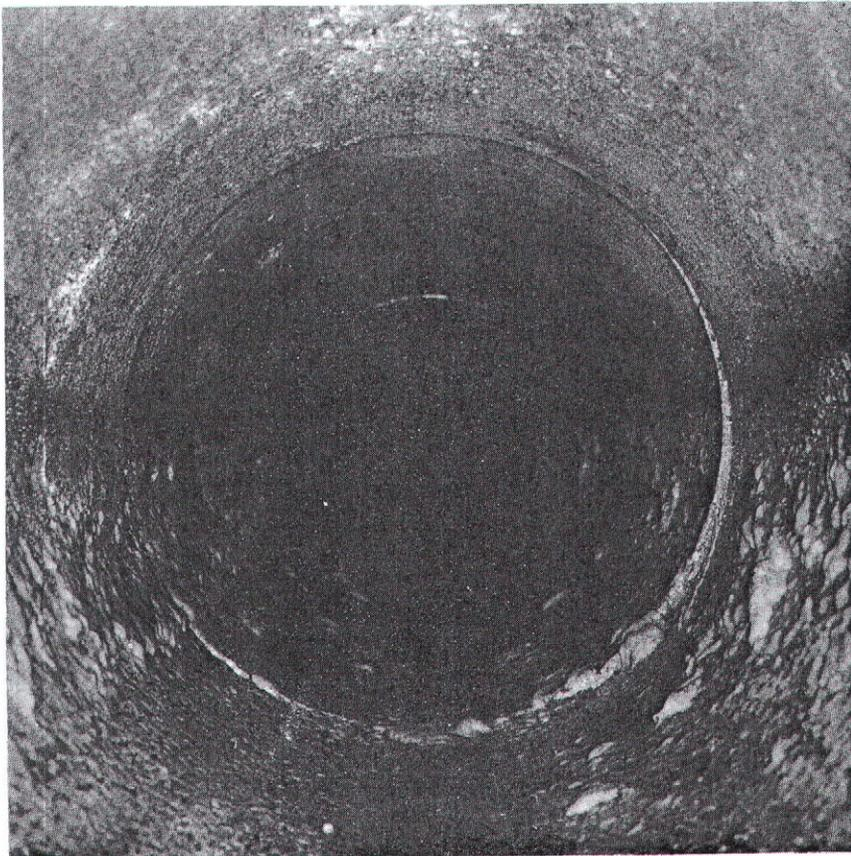
**Plate 5** Roughness of composite surface (pipe-full)  $k_c = 1.2\text{mm}$
