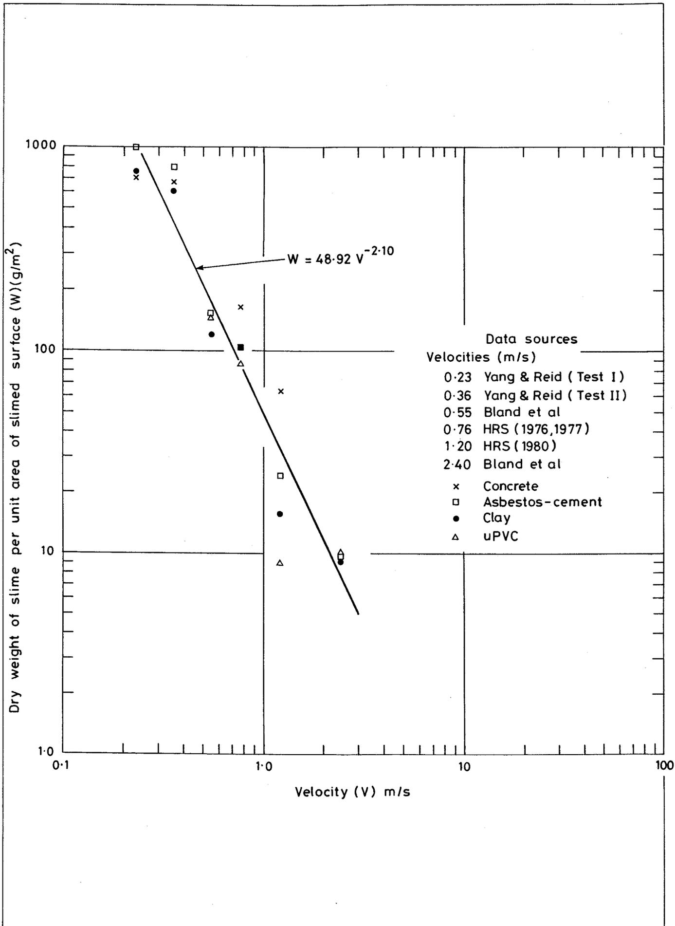
Fig 17 Equilibrium slime weight as a function of velocity
