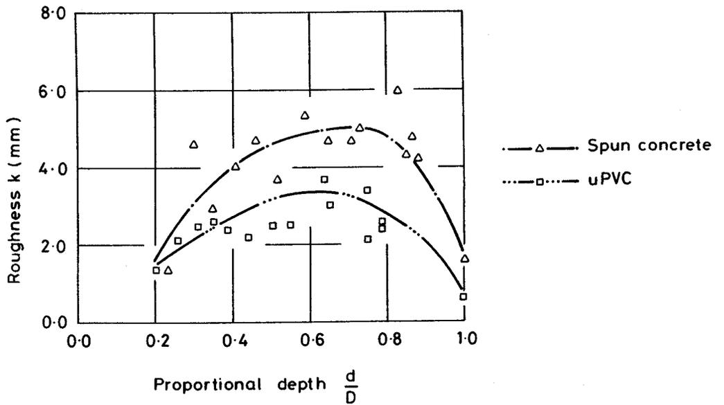
Fig 10 Variation of roughness with depth of flow - Run 1
