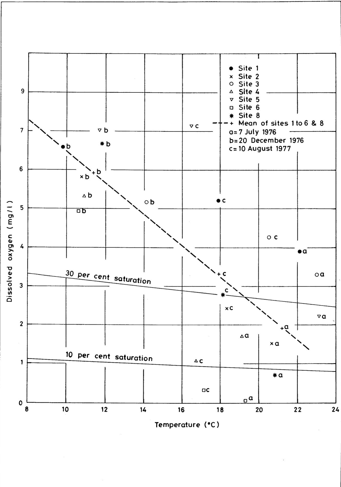
Fig 7 Dissolved oxygen levels in Oxford sewers
