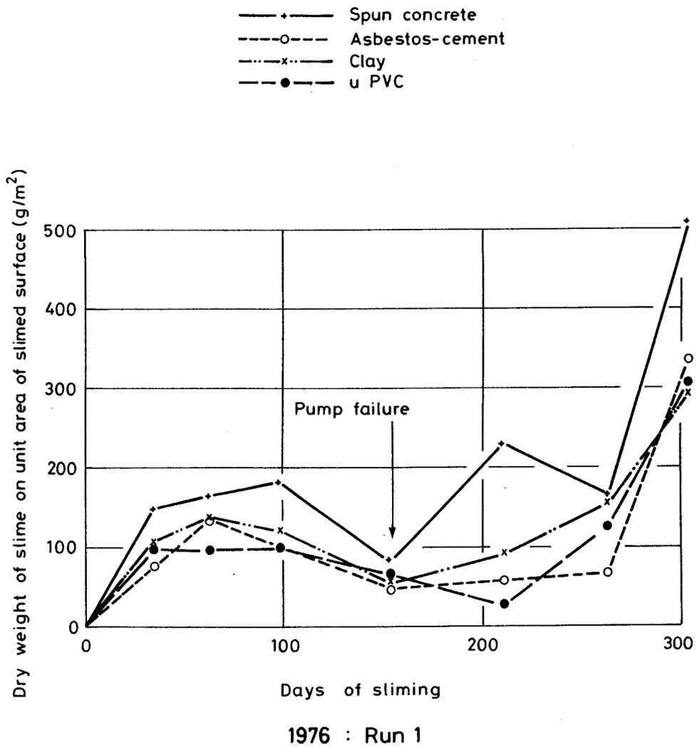
Fig 13 Weight of slime scraped from pipe walls - Run 1
