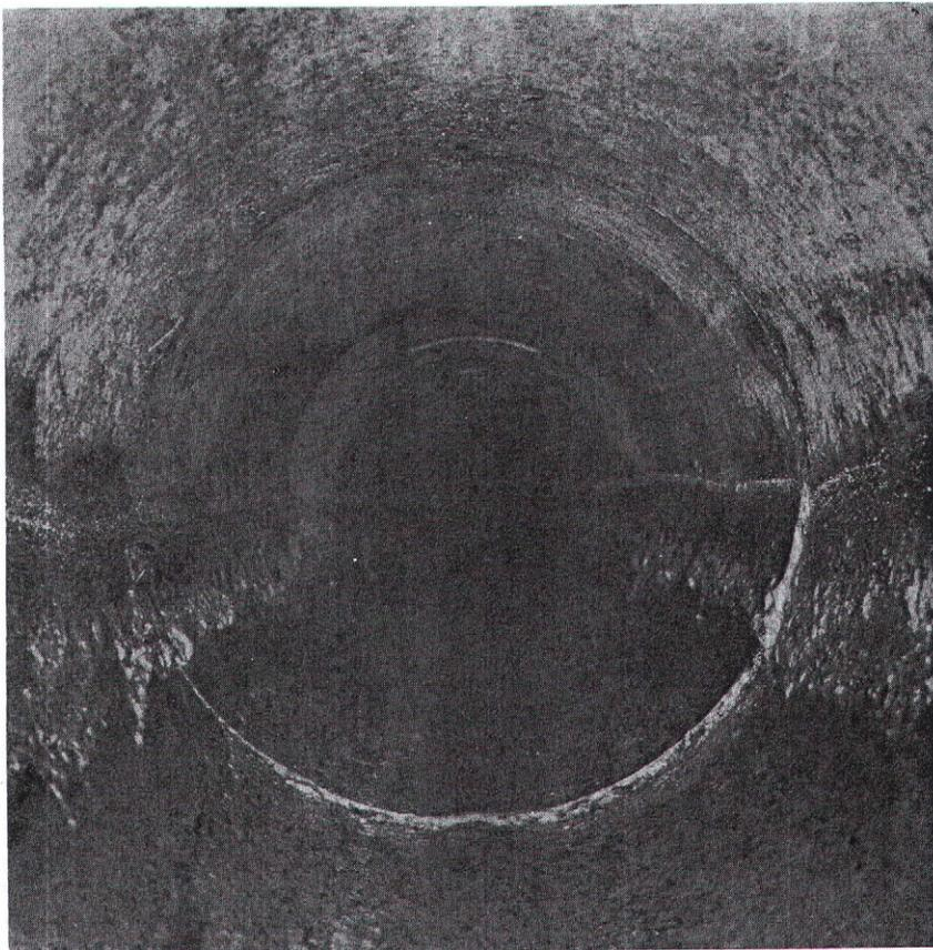
**Plate 3** Roughness of composite surface (pipe-full)  $k_c = 0.4\text{mm}$
