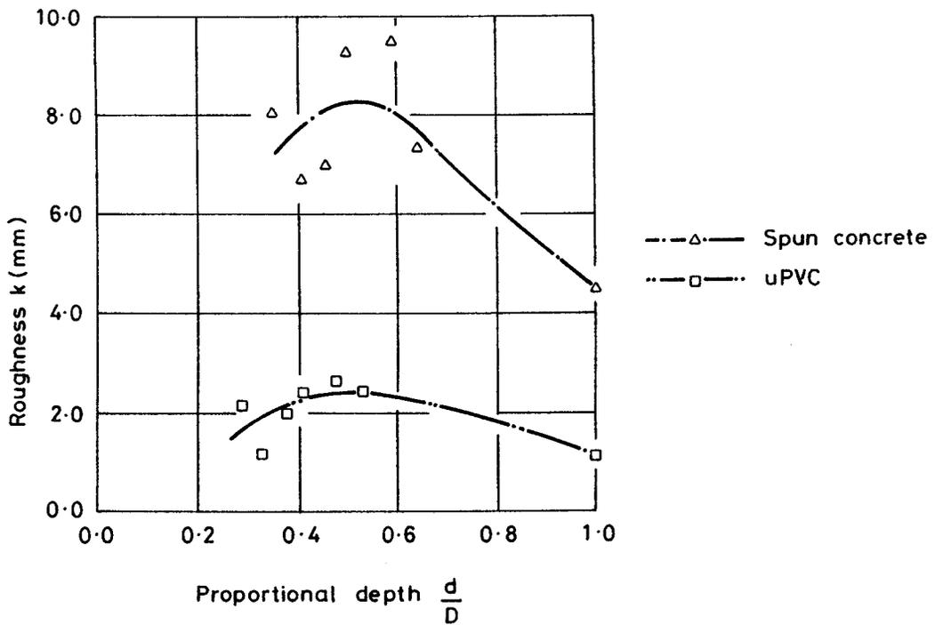
Fig 12 Variation of roughness with depth of flow - Run 2
