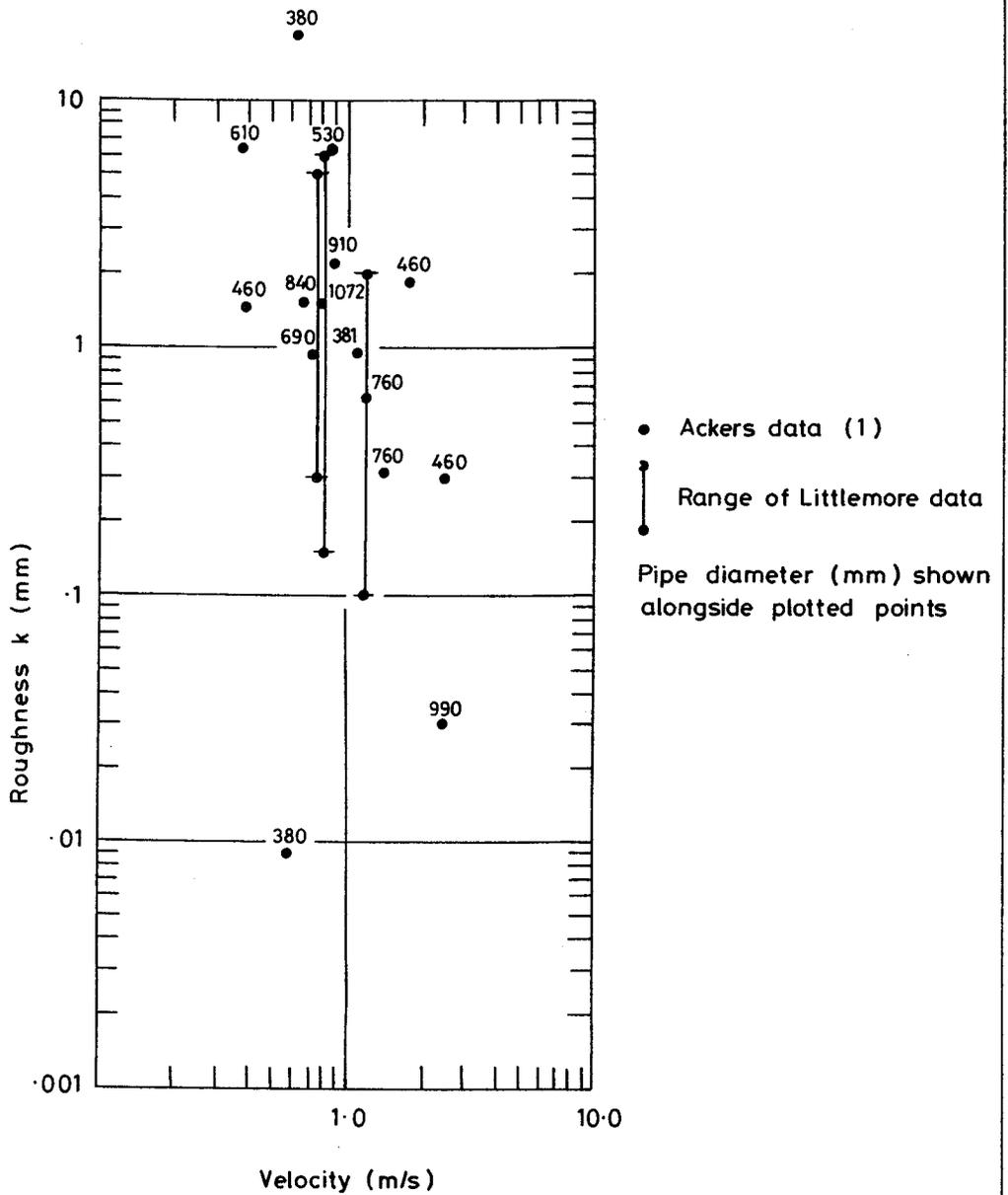
Fig 18 Variation of roughness with velocity : Ackers and Littlemore data
