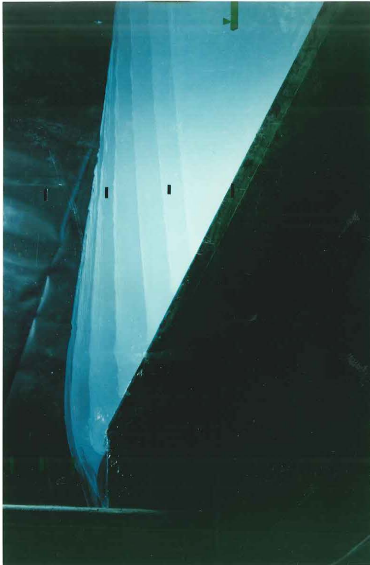
Plate 2 Overtopping 1:2 seawall, H=2.4m
