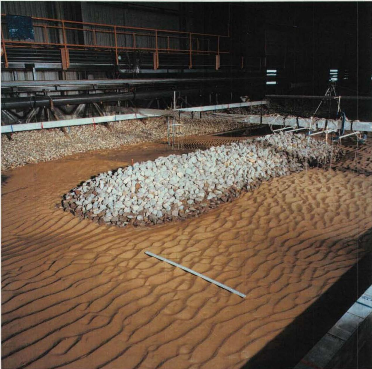
**Plate 3** Test 1 final bathymetry seen from Southeast. Length of ruler is 1m
