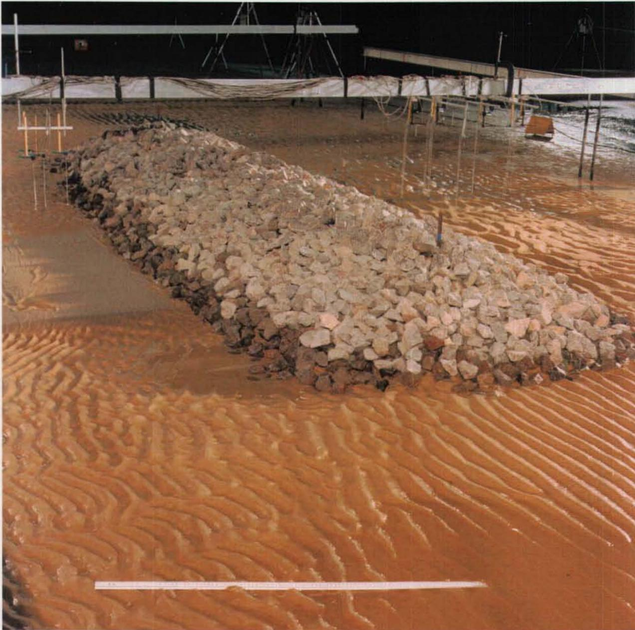
**Plate 8** Test 5 final bathymetry: South roundhead from rear. Length of ruler is 1m
