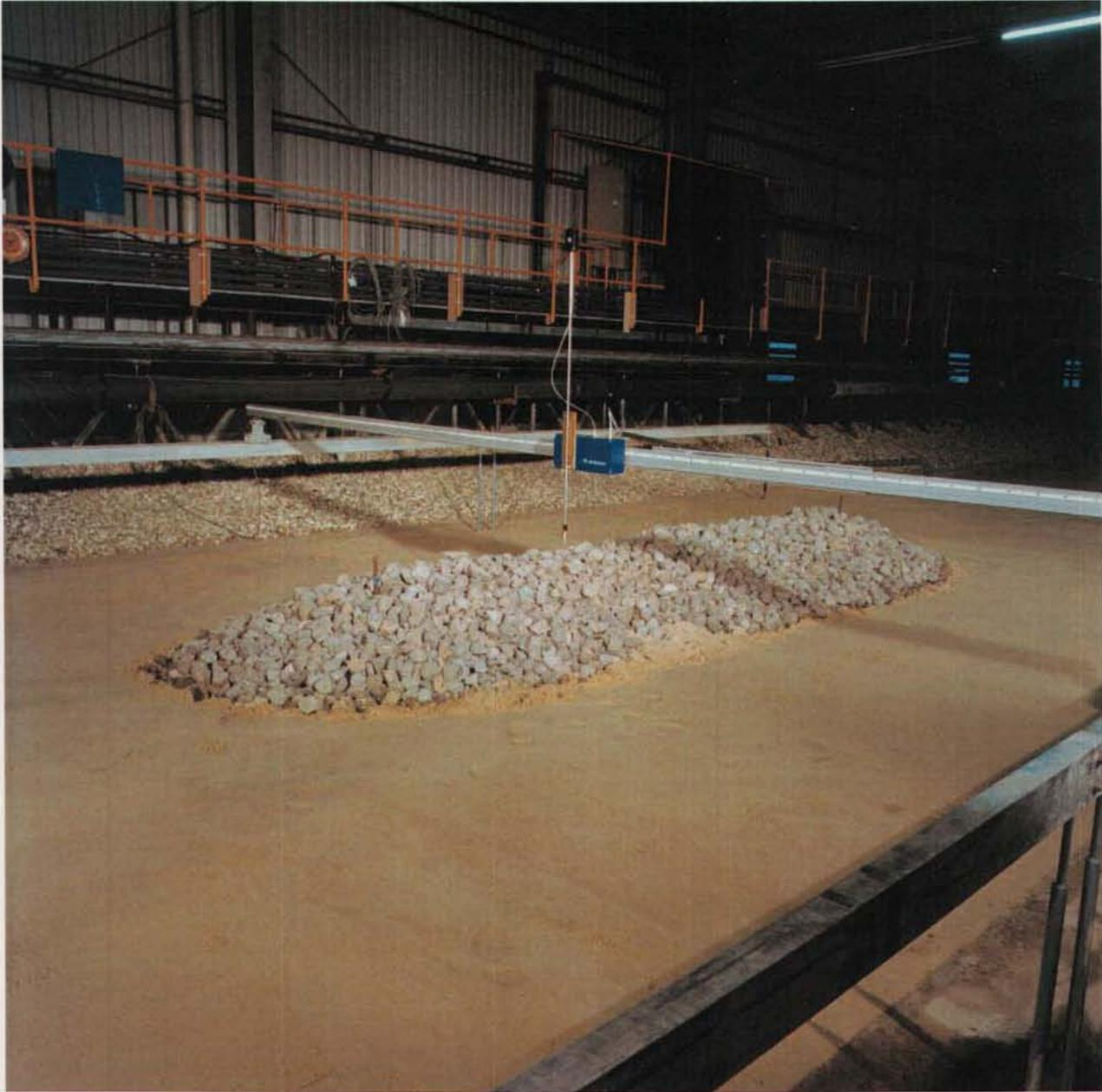
**Plate 2 Breakwater and profiler rails**
