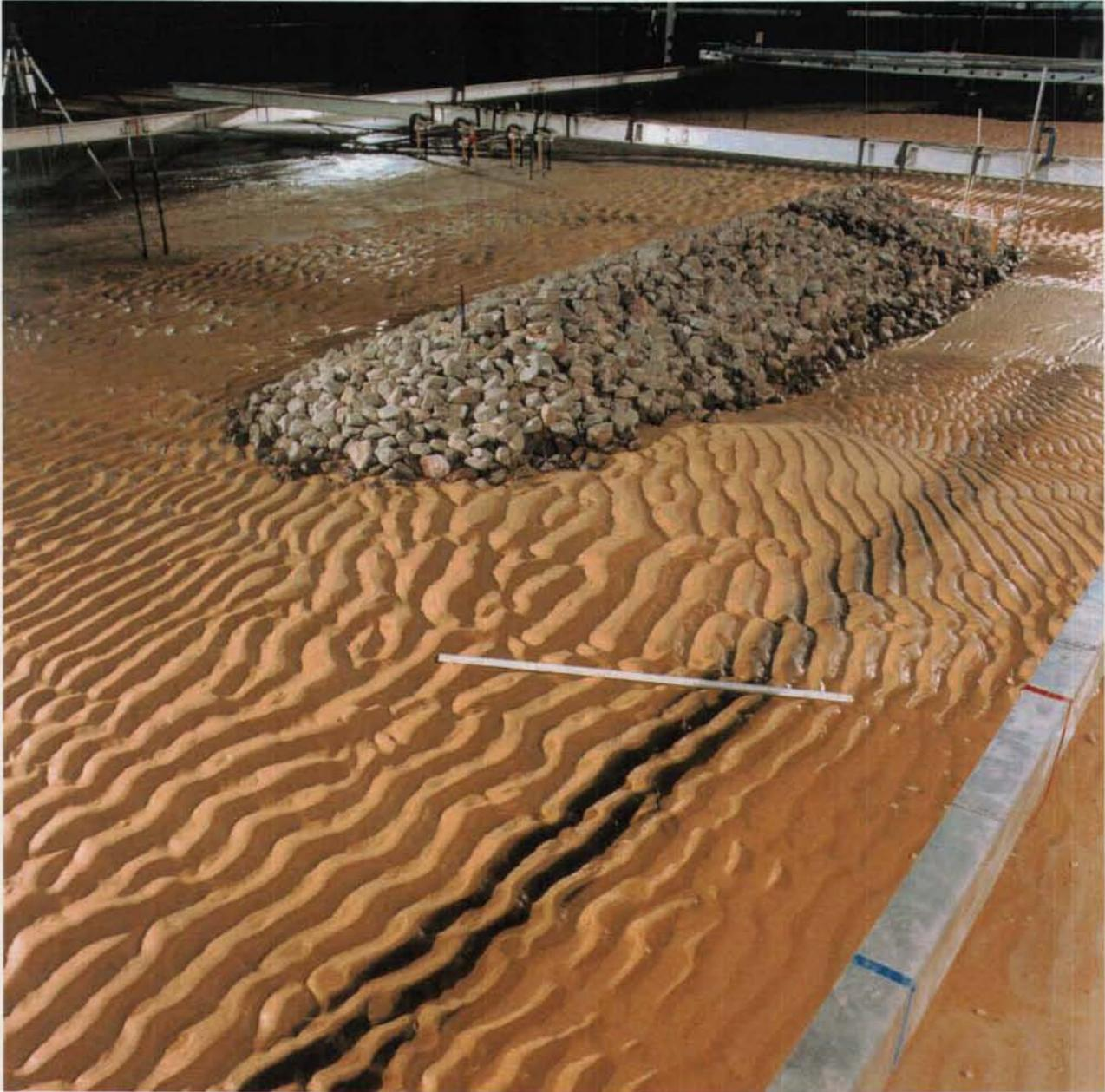
**Plate 10** Test 5 final bathymetry: North roundhead from rear. Length of ruler is 1m
