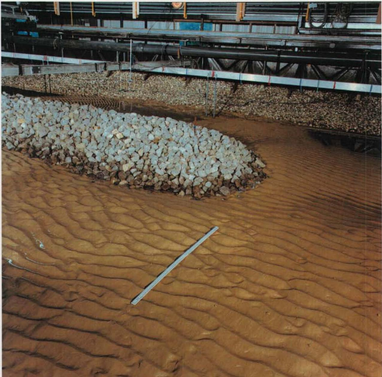
**Plate 5** Test 1 final bathymetry: North roundhead from front. Length of ruler is 1m
