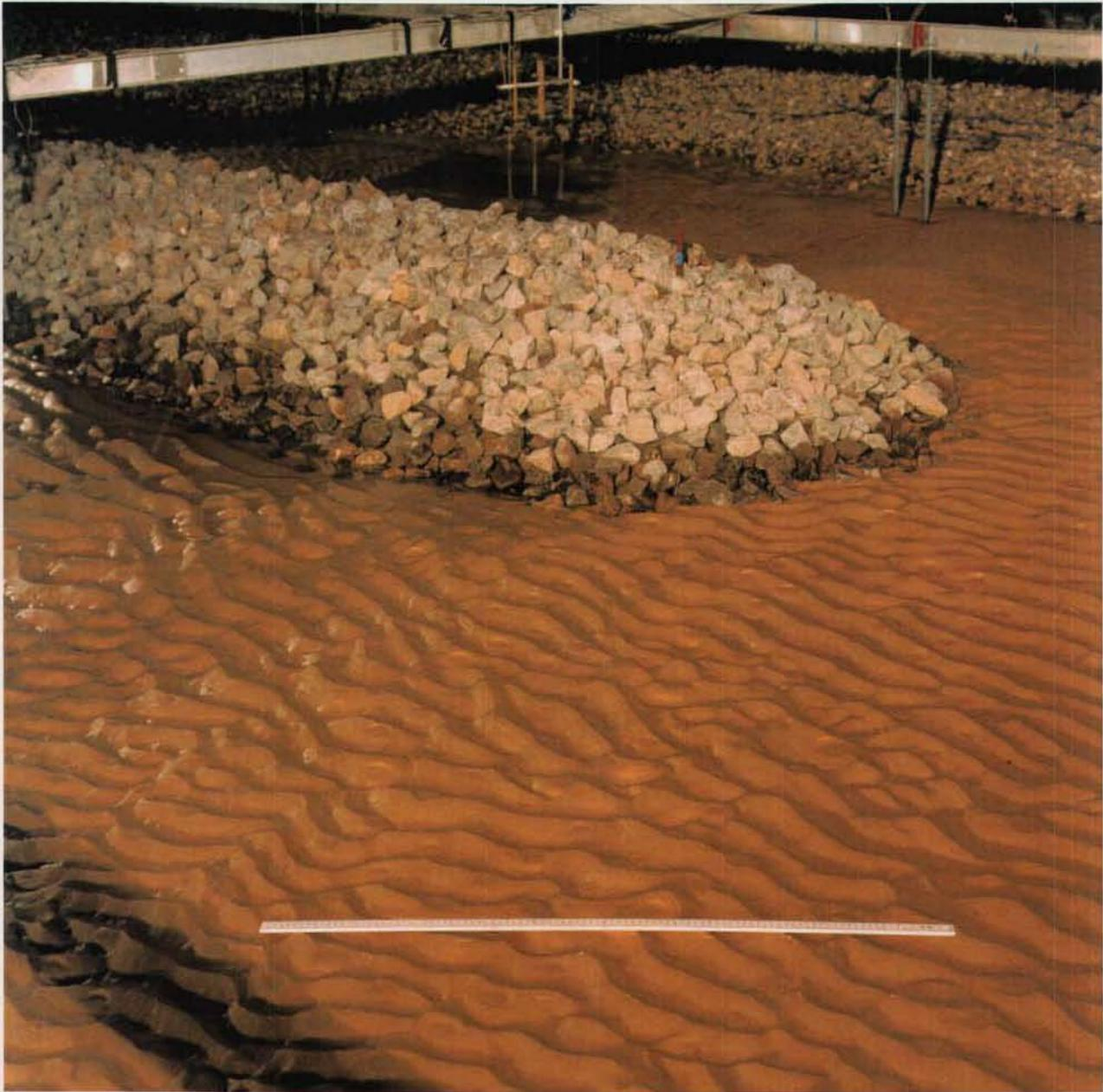
**Plate 9** Test 5 final bathymetry: North roundhead from front. Length of ruler is 1m
