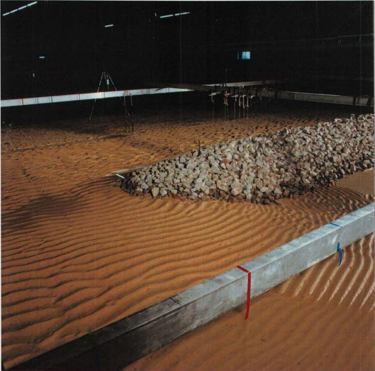
**Plate 6** Test 1 final bathymetry: North roundhead from rear
