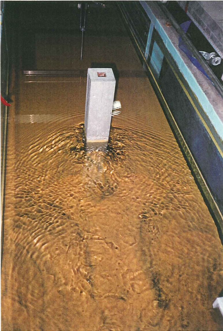
Plate 8 Unidirectional test with sediment size d_{50}=0.44\text{mm}
