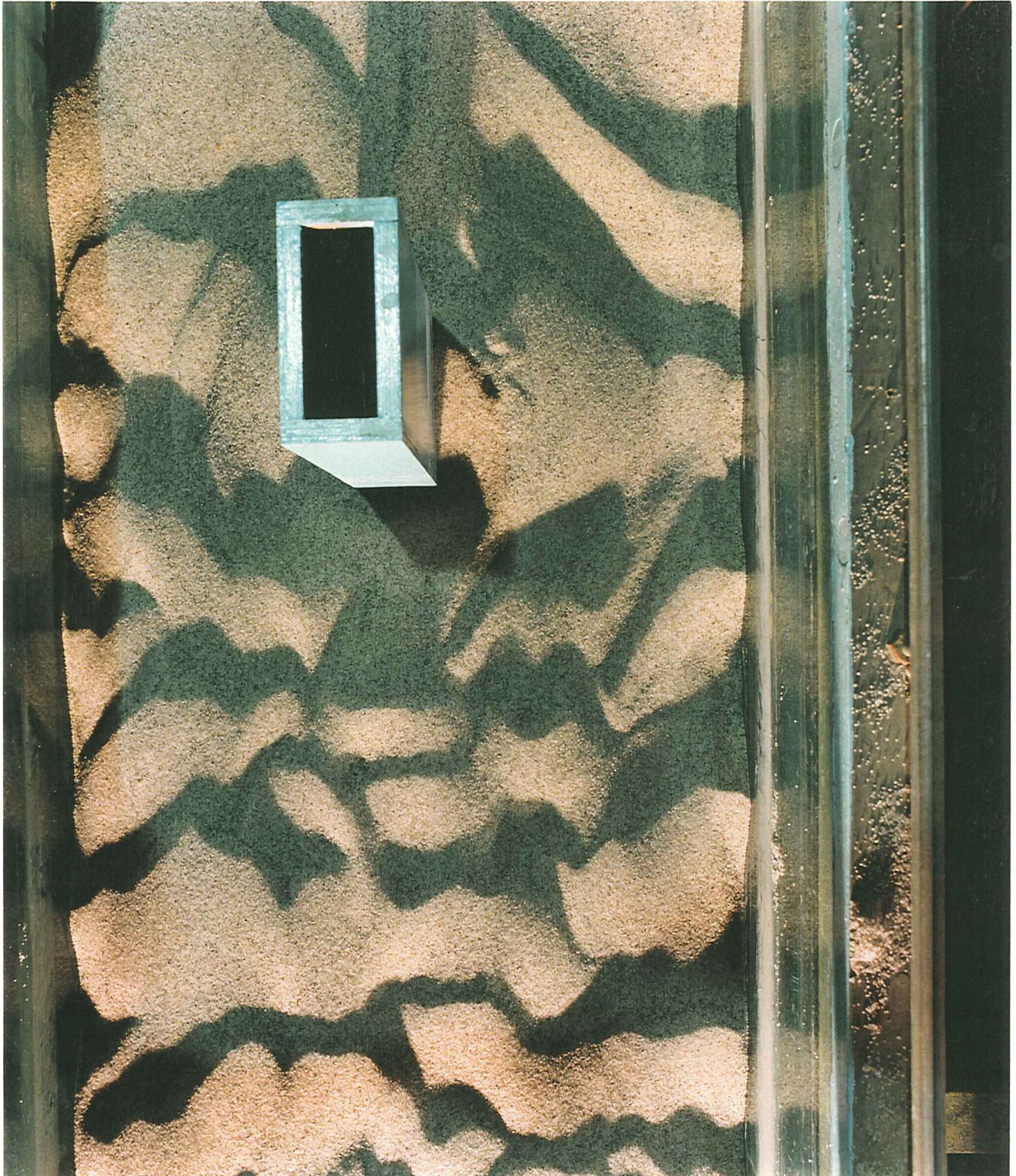
Plate 6 Rectangular structure. Scour pattern (in plan) at end of test RC2
