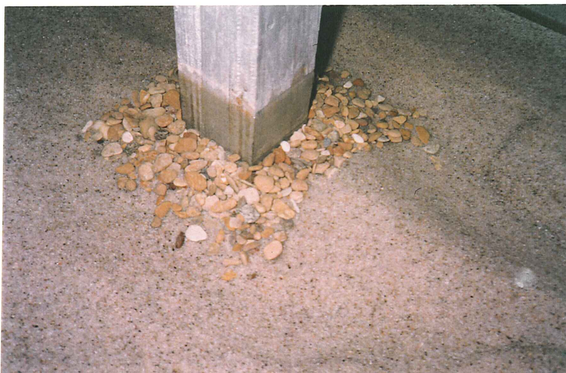
Plate 12 Stone mattress 50mm wide at end of tidal test
