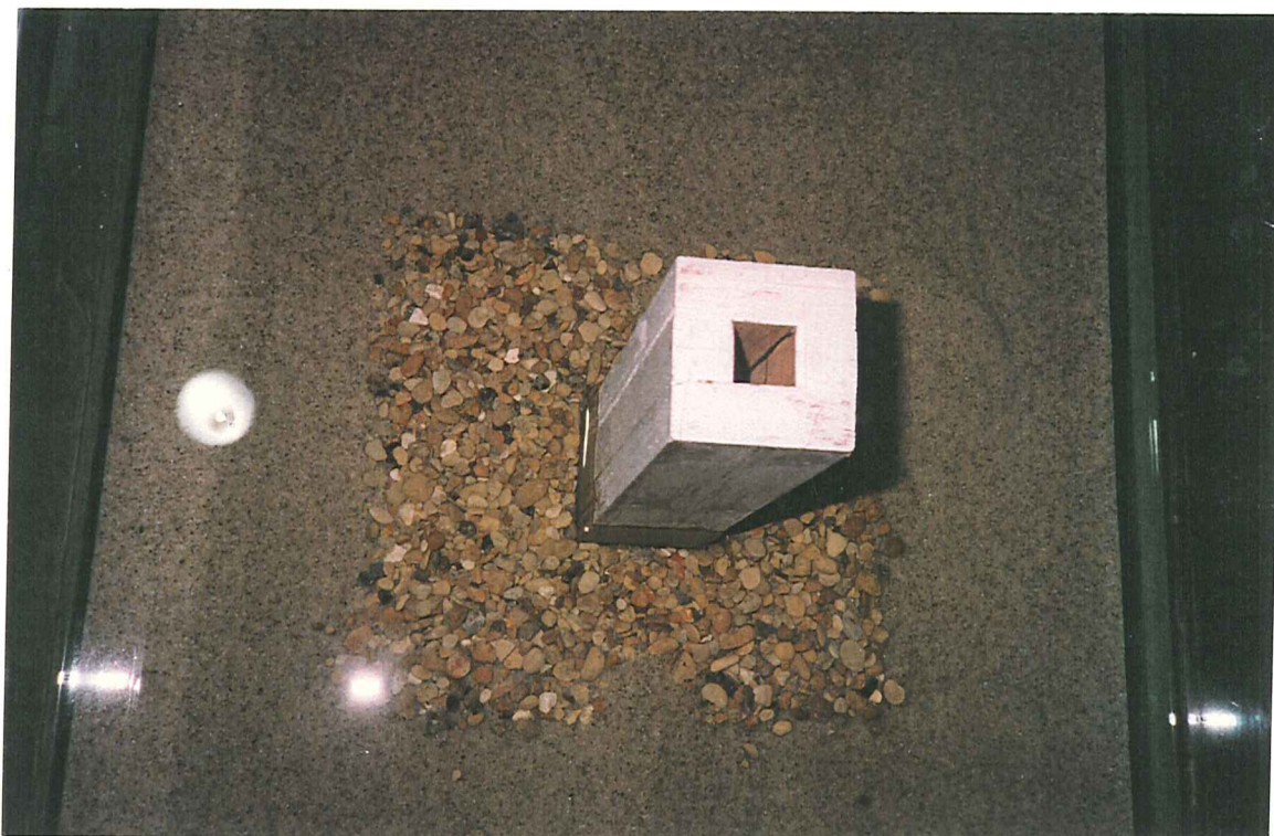
Plate 11 Stone mattress 150mm wide at end of tidal test
