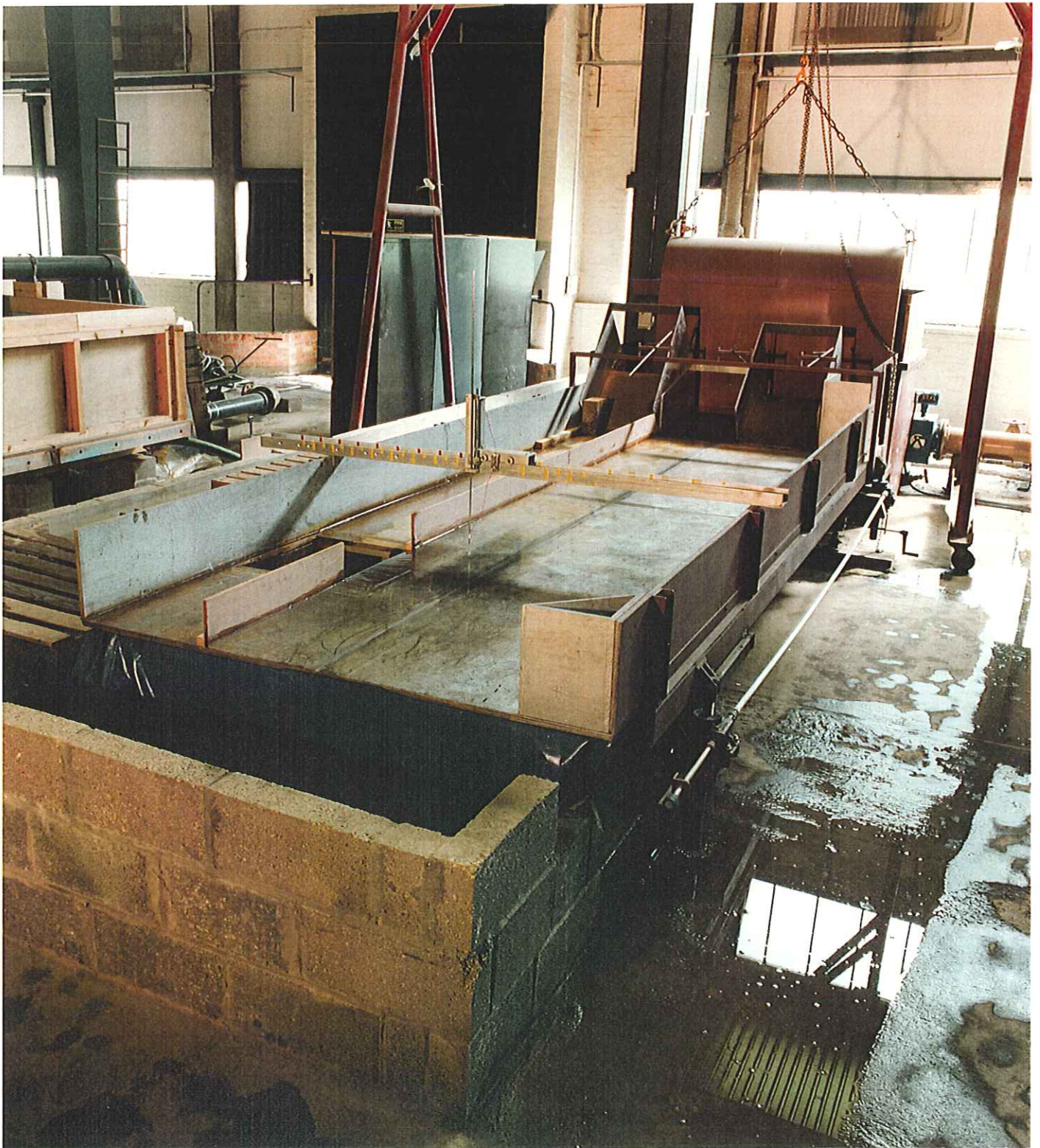
Plate 5 View of test rig showing kerb inlet
