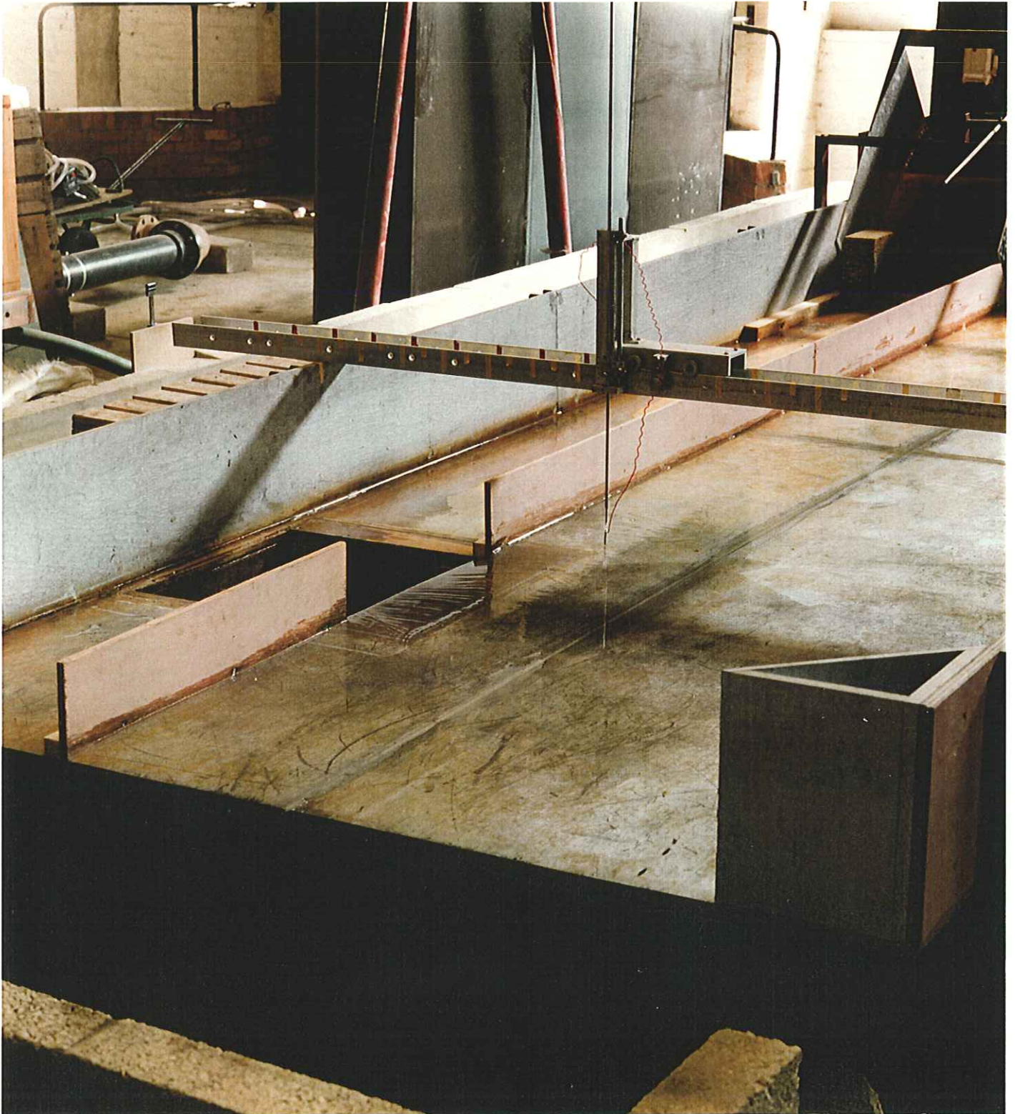
Plate 6 Straight kerb inlet, 0.5m long
