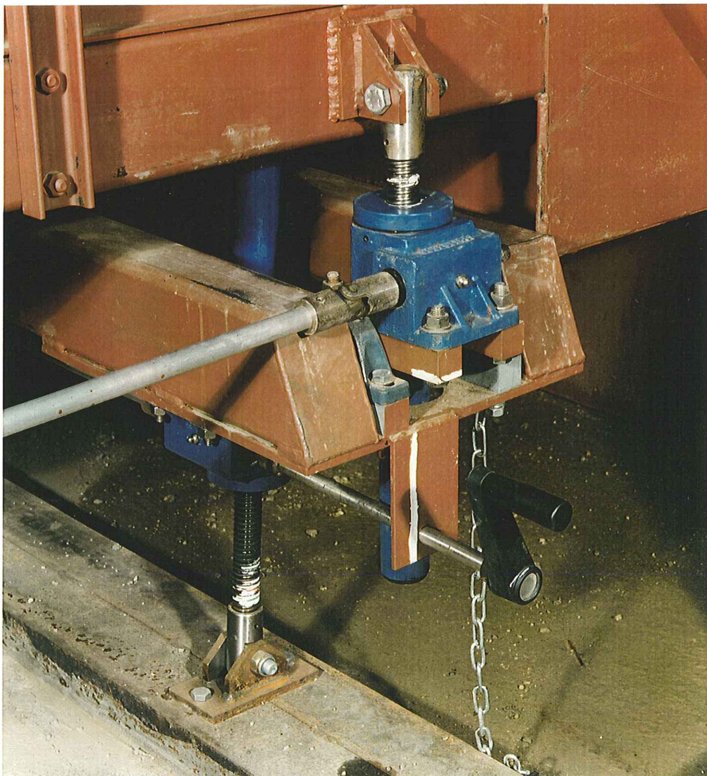
Plate 2 View of the system of jacks (top jack for the cross-fall, bottom jack for the gradient)
