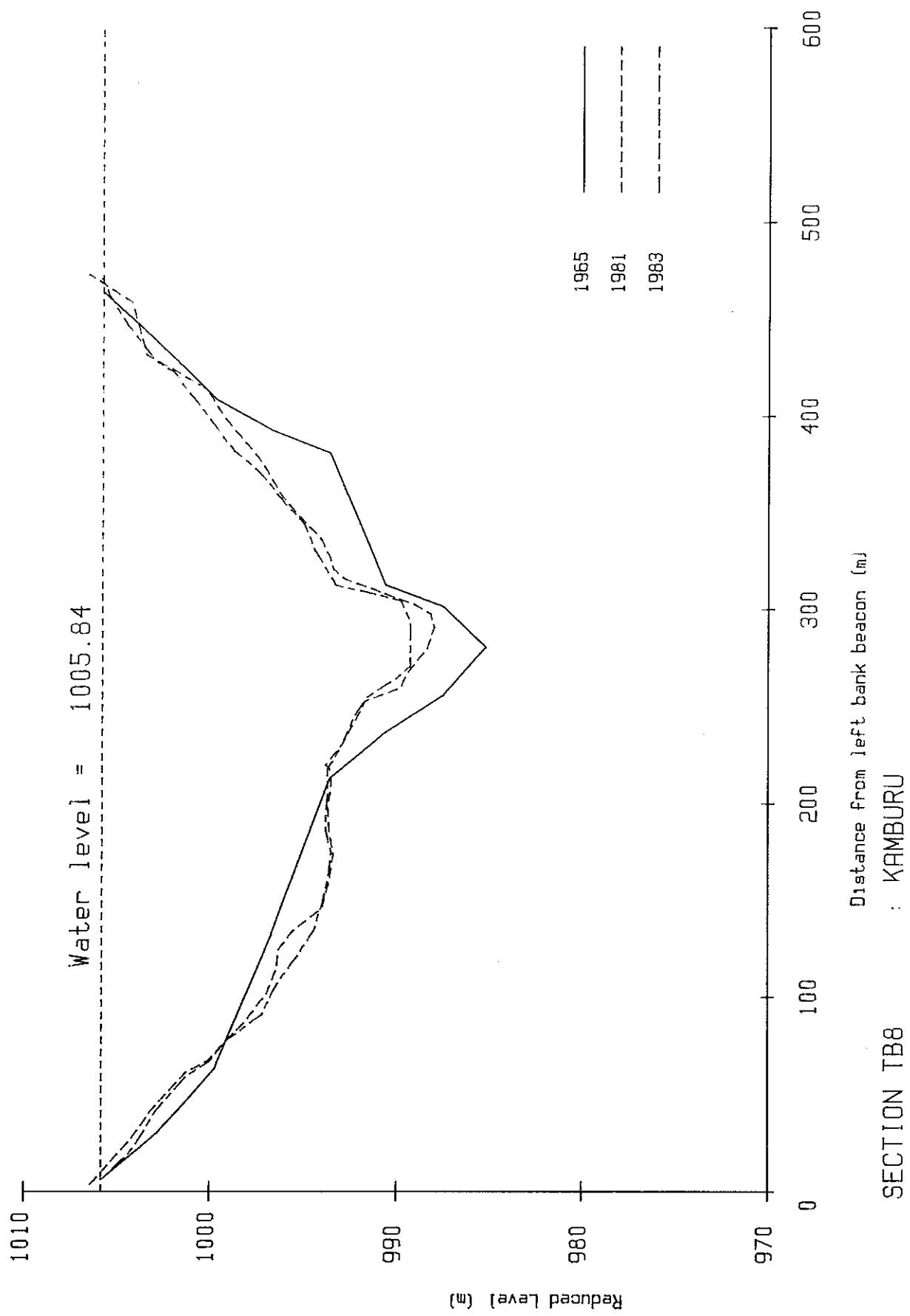
Fig 4.22 Kamburu Reservoir - section TB8
