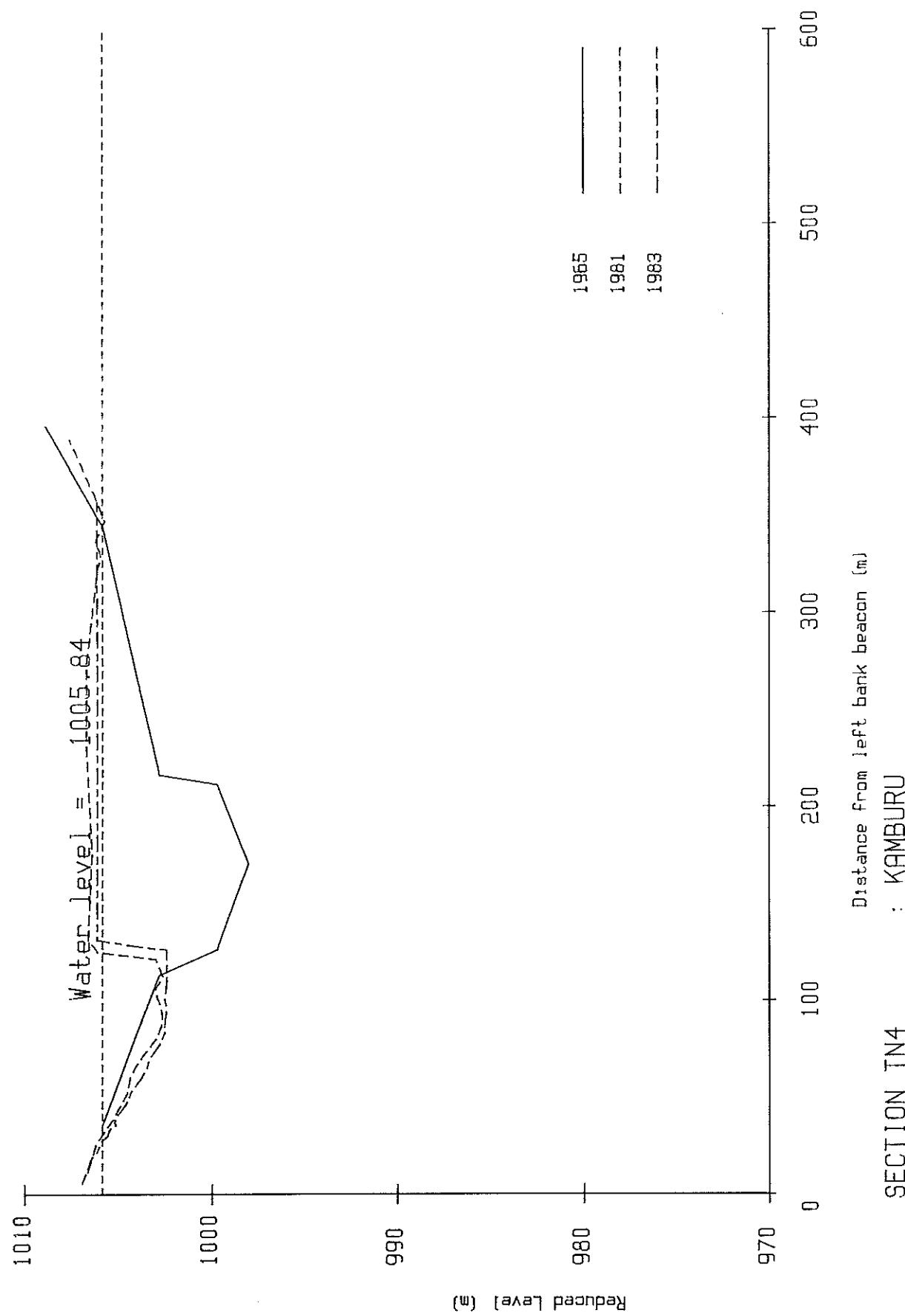
Fig 4.4 Kamburu Reservoir - section TN4
