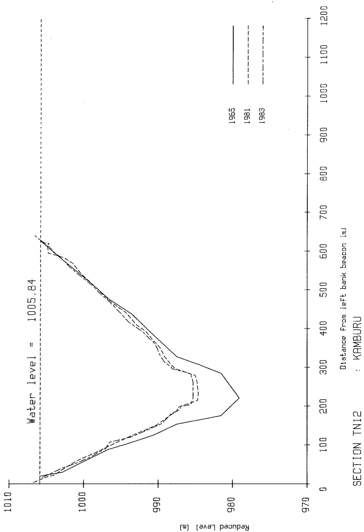
Fig 4.13 Kamburu Reservoir - section TN12
