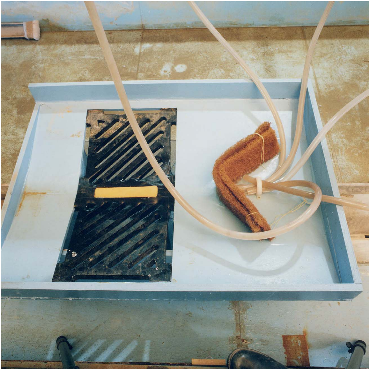
Plate 5 Set-up II – Outfall from surface water channel (in-line)
