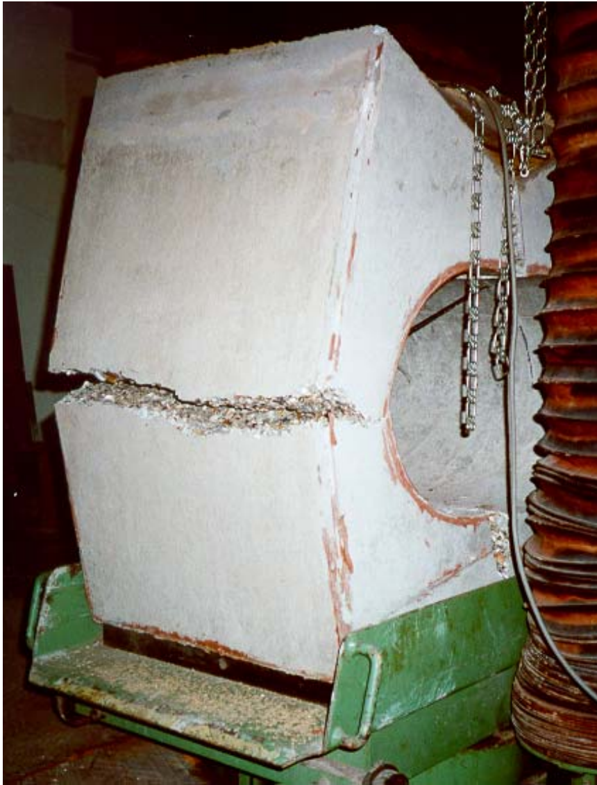
Plate 17 Collapse of TRL Sample 2; 500mm diameter void and 150mm top cover
