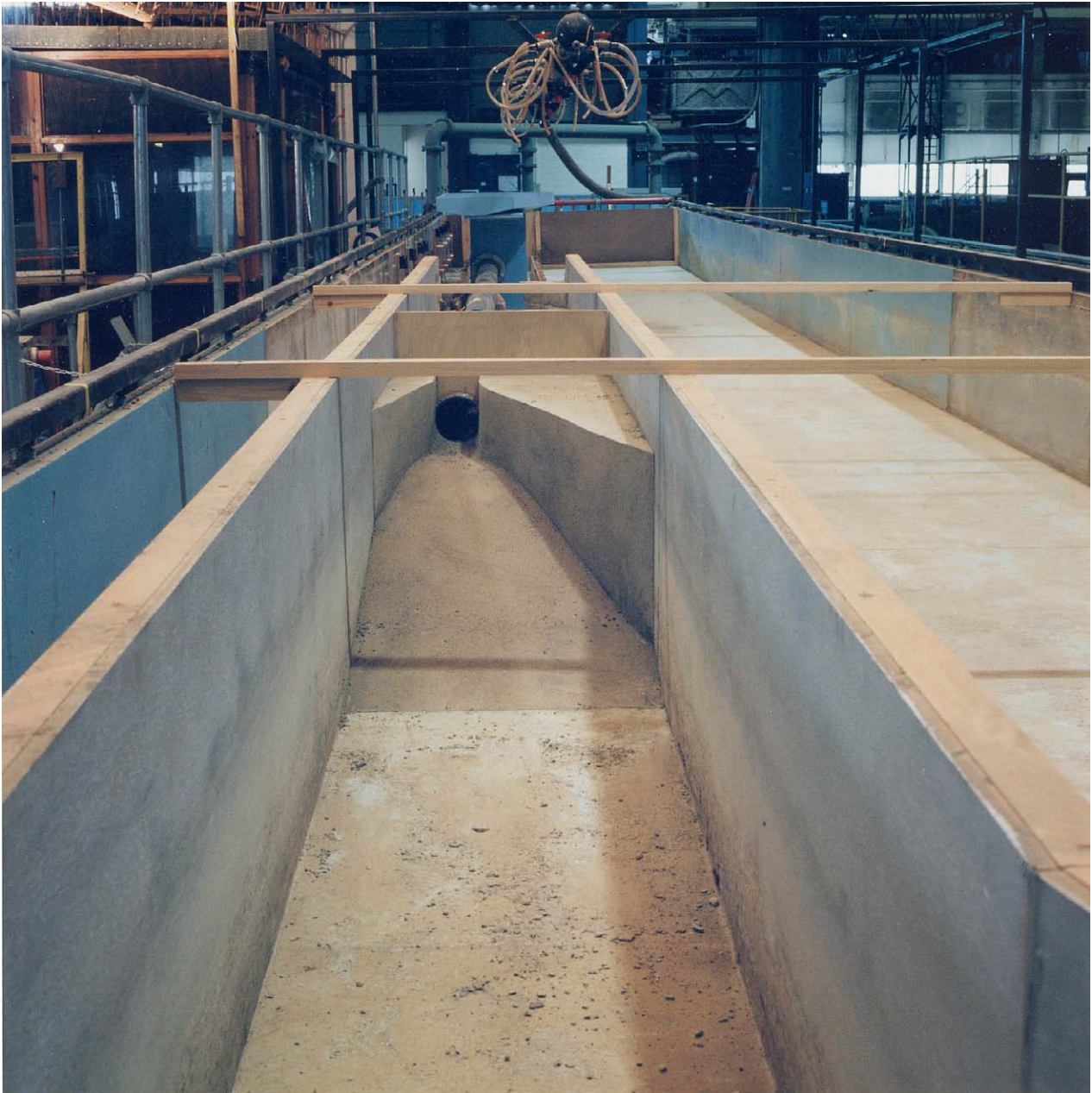
Plate 2 Set-up I – Upstream transition into test pipe
