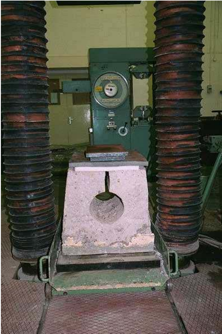
Plate 14 Structural test of Stoney Clouds Section 1: 210mm diameter void
