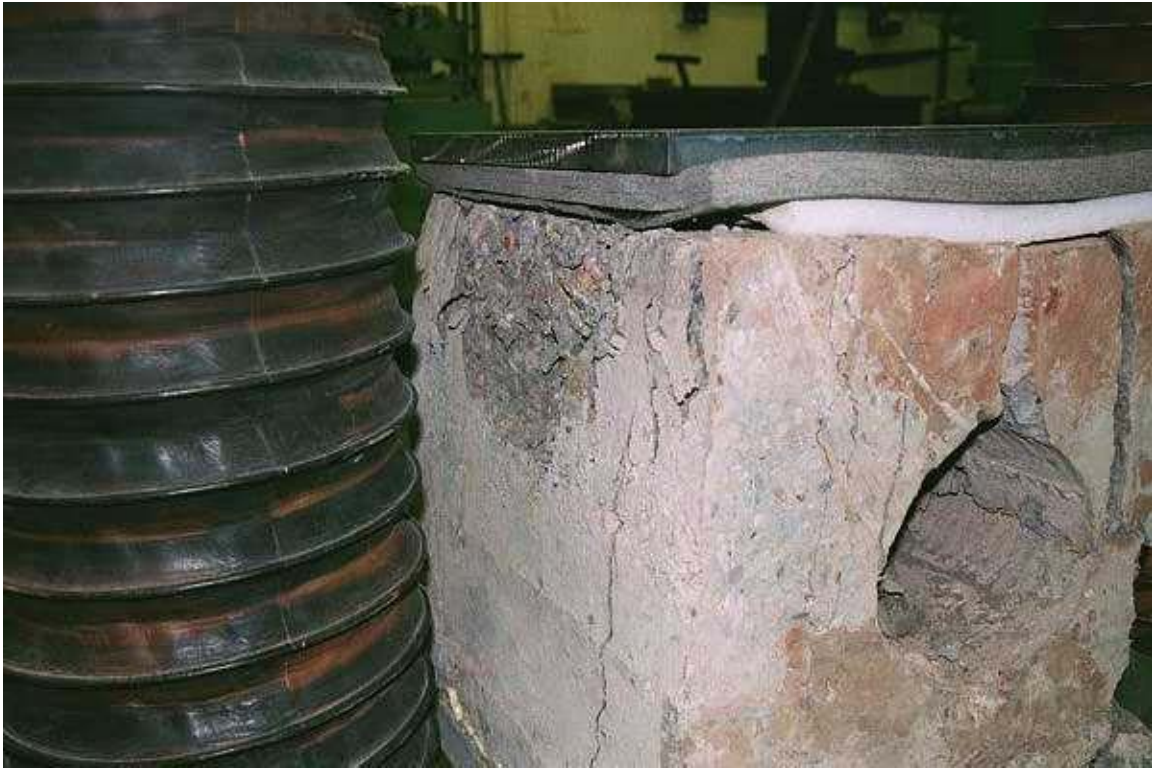
Plate 13 Collapse of Stoney Clouds Section 1: 195mm diameter void
