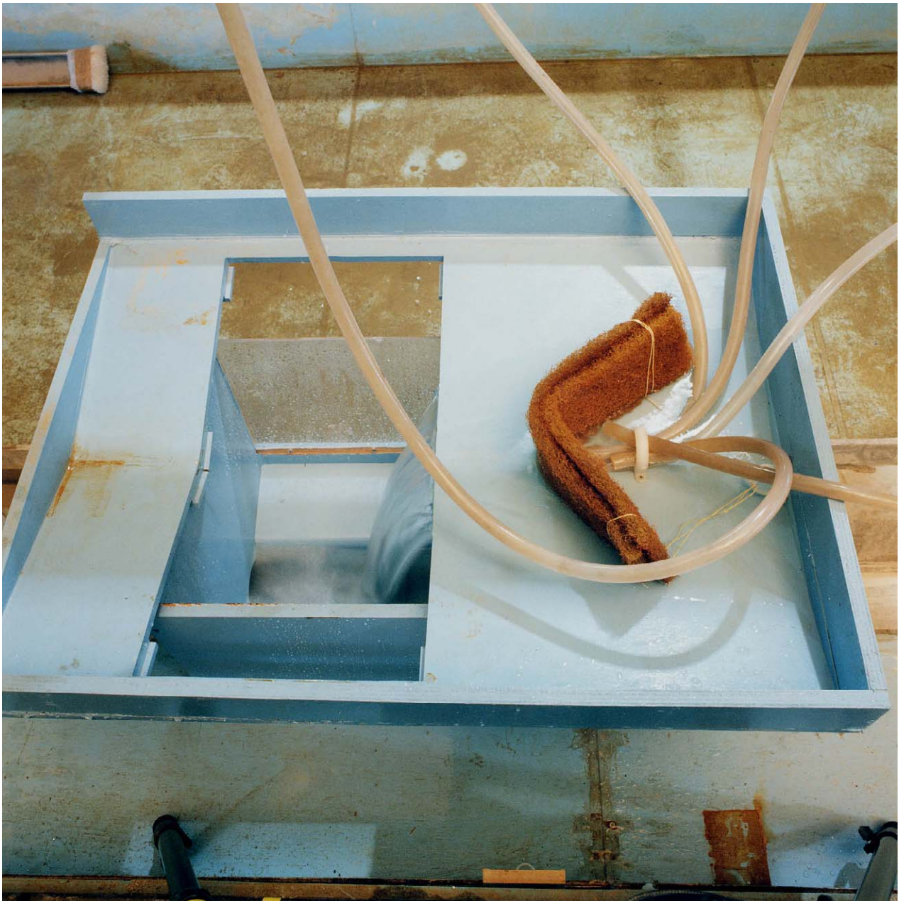
Plate 10 Set-up II (Benching IIa). Flow from surface channel entering the chamber with gratings removed for visual observation
