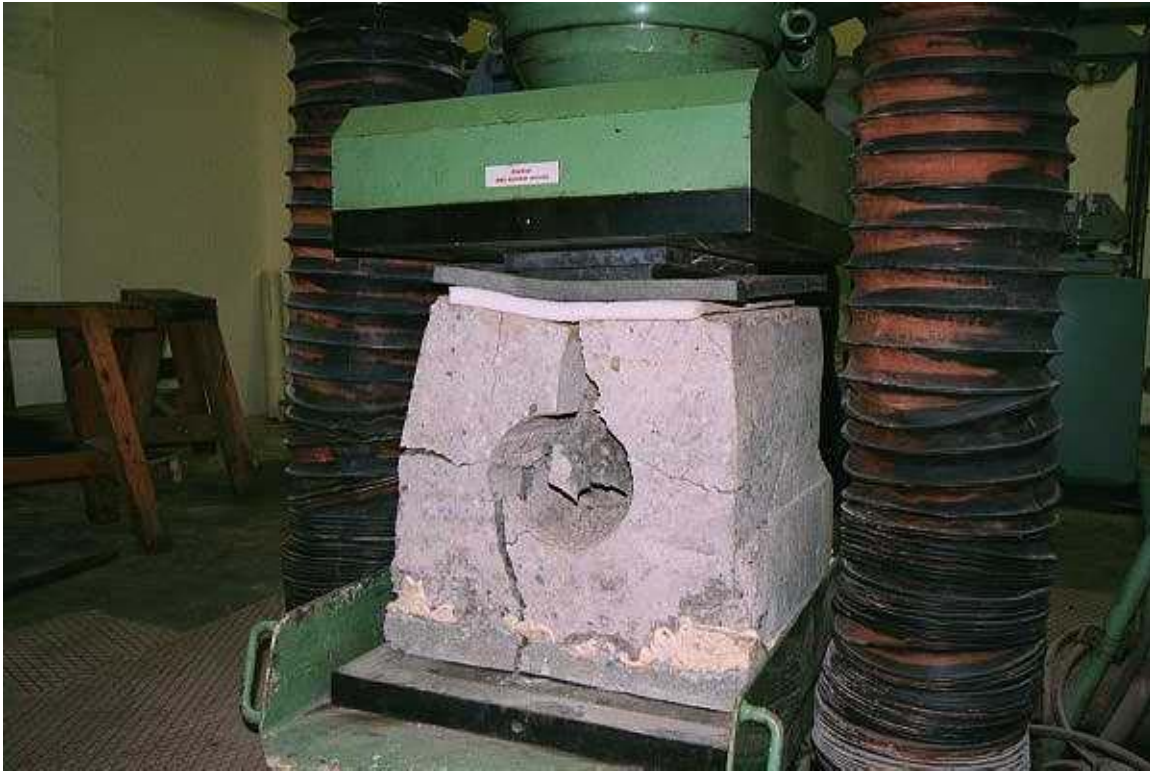
Plate 15 Collapse of Stoney Clouds Section 2: 210mm diameter void
