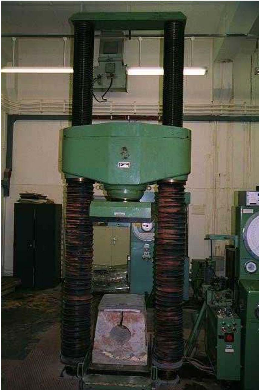
Plate 12 Structural test of Stoney Clouds Section 1: 195mm diameter void
