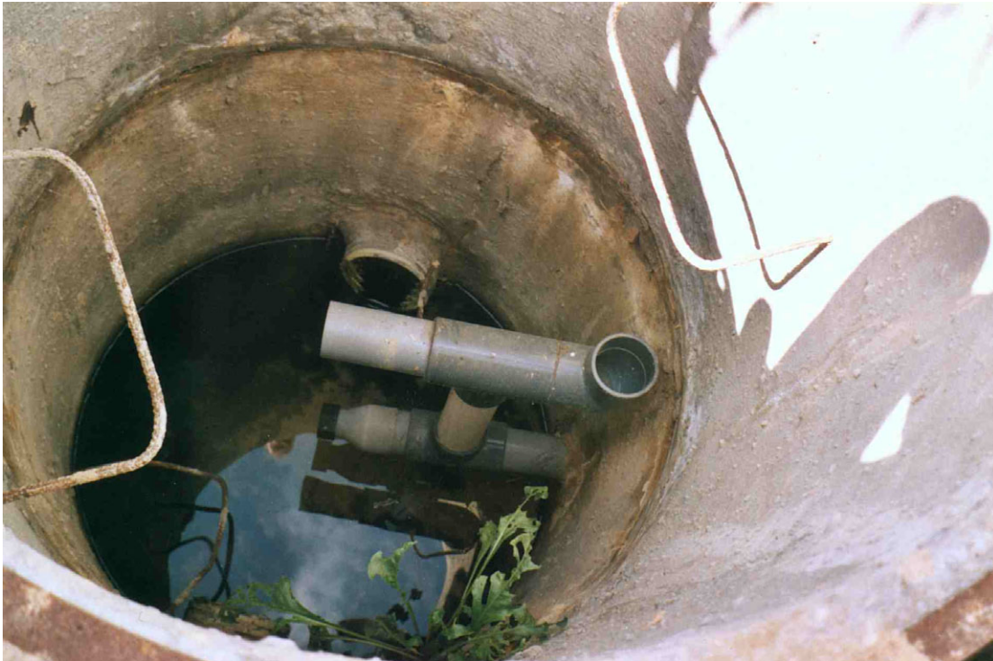
Figure 3 Prototype controlled drainage weir device
