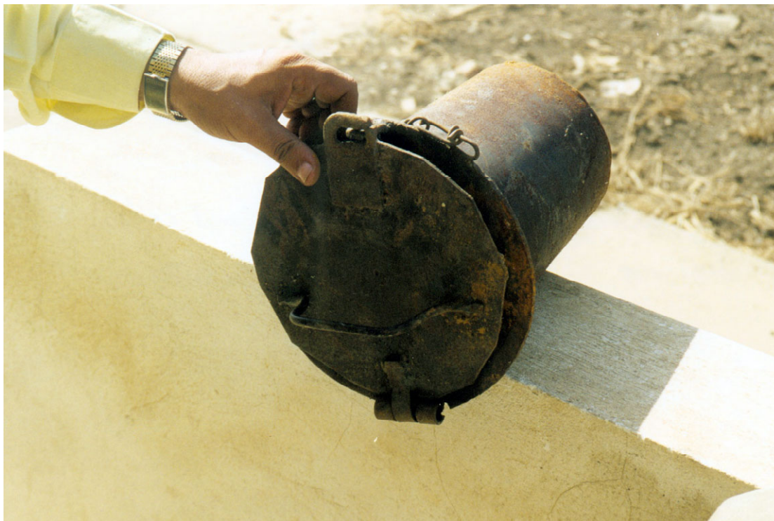
Figure 2 Flapgate used to block drainpipes and control drainage outflows
