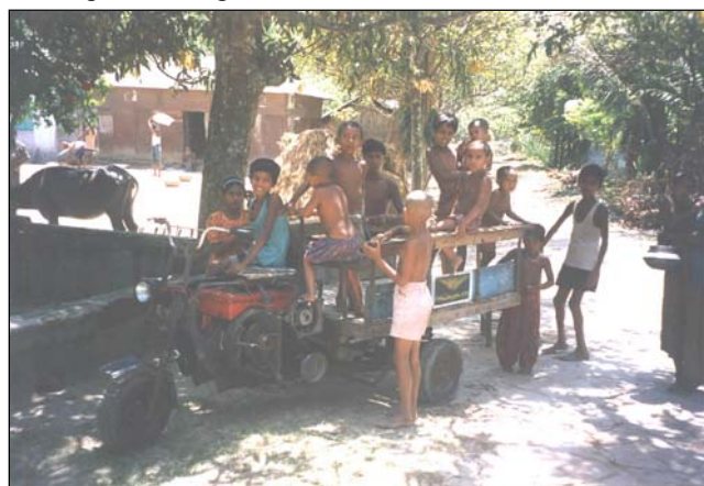
Figure 5: Tubewell engine converted to rickshaw/van
