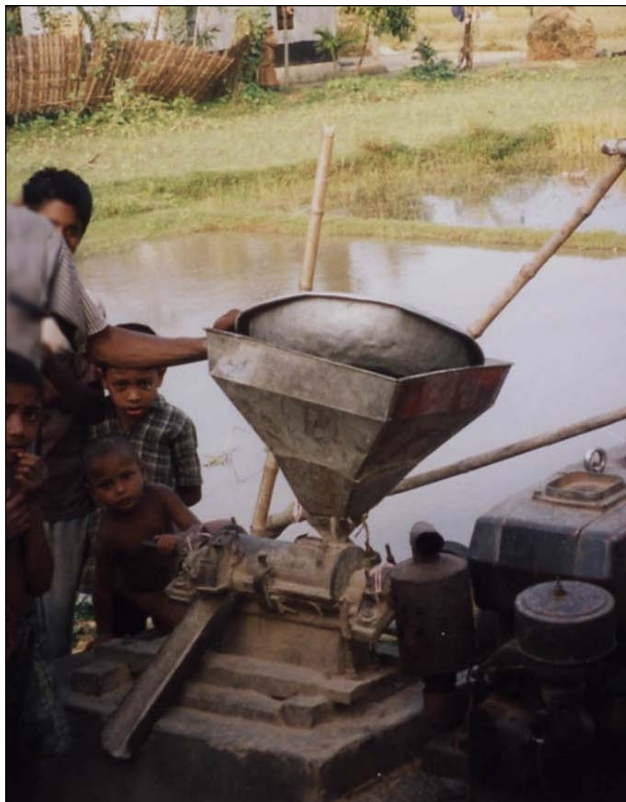
Figure 4: Tubewell engine converted to rice husking machine, Talki, Bangladesh
