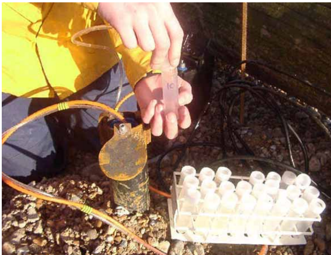
Figure 7.1 Water samples being drawn at Pevensey for chemical analysis
