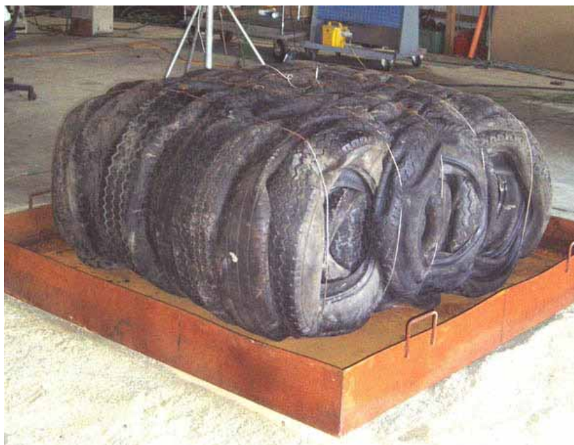
Figure A7.3 Tyre bale used for fire ignition testing
