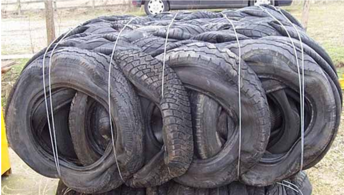
Figure 4.4 Baled product containing approximately 100 used tyres (courtesy Environment Agency)
