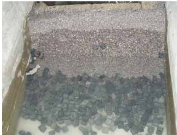
Figure A5.3 Post wave test collapse (Series 2)
