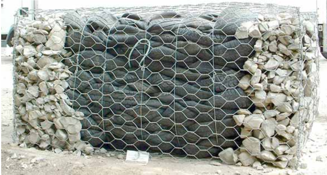
Figure 5.38 Tyre bale as centre fill for gabion box (courtesy Northern Tyre Recycling)
