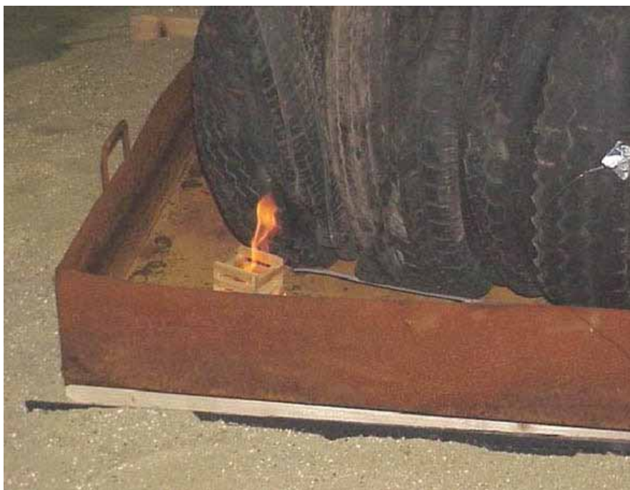
Figure A7.4 Ignition attempt at one corner of the tyre bale
