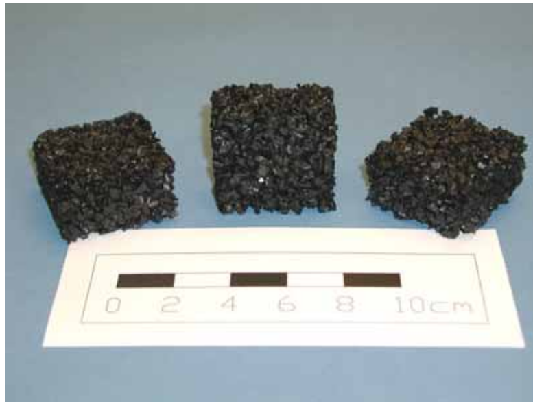
Figure A5.1 Model tyre bales
