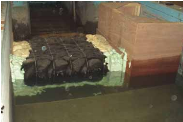
Figure A4.1 Bale being tested for permeability over a long pathway.
