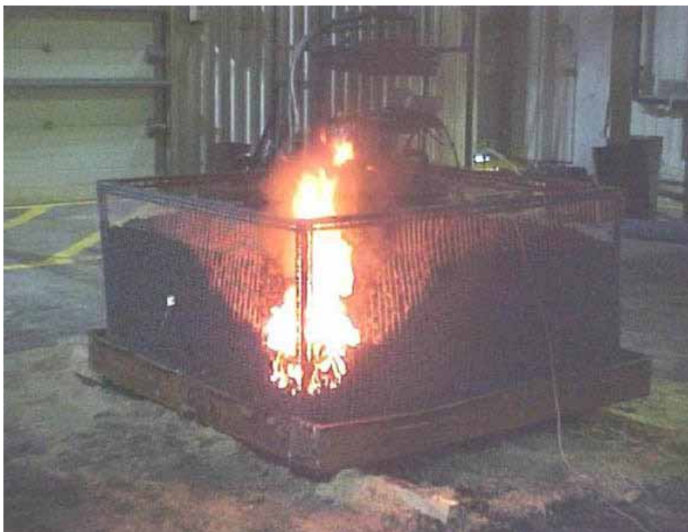
Figure A7.10 Tyre crumb ignition location
