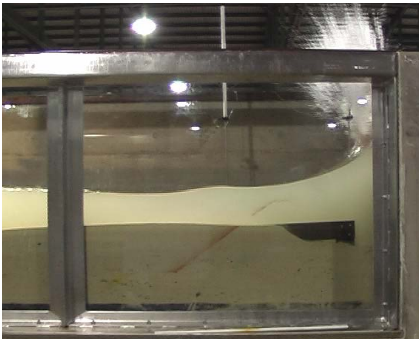
Figure 3: Wave breaking against a vertical wall. Metre stick for scale
