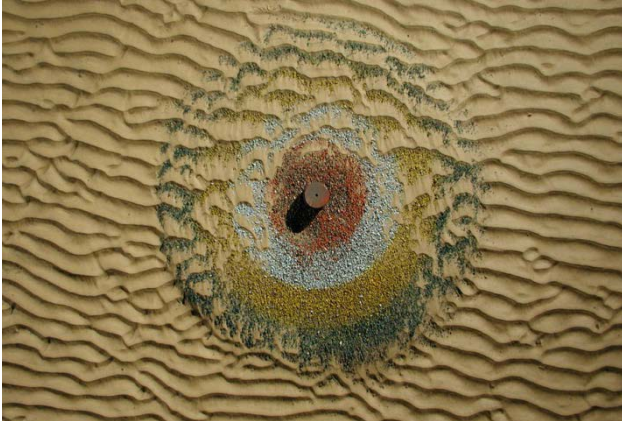
Figure 8: Overhead photograph of end result of one of the physical model tests with a static protection design
