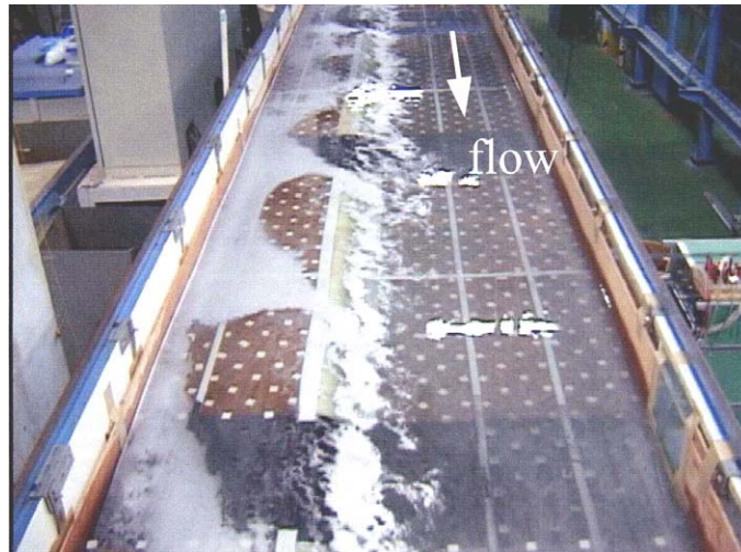
Figure 4 Visualization of planform vorticity in a straight two-stage channel, (H-h)/H = 0.180 (after Ikeda, Sano, Fukumoto & Kawamura, 2006).
