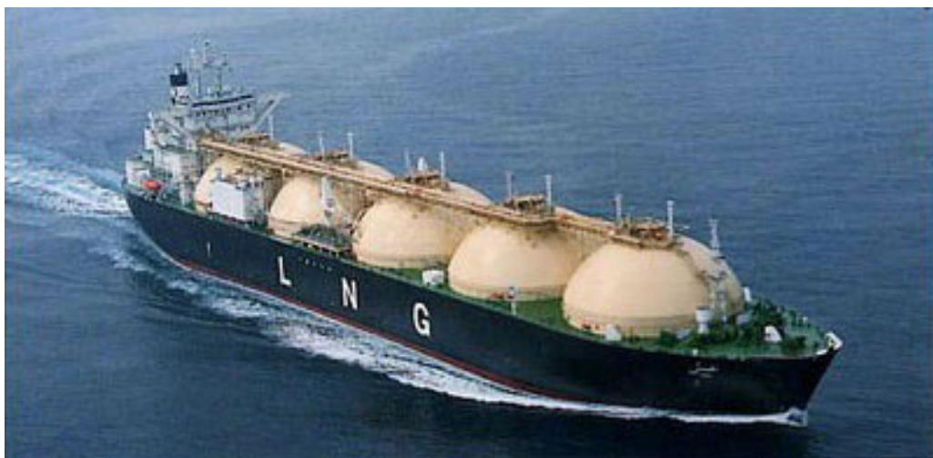
Figure 2: Typical Moss spherical LNG Tanker
