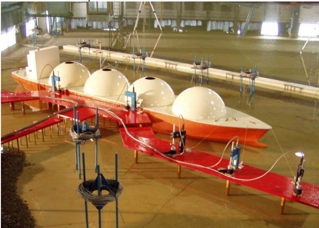
Figure 7: Physical modelling of mooring systems
