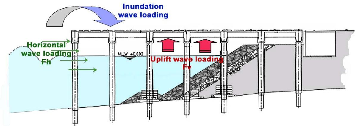
Figure 1. Wave-in-deck loads on a platform supported by piles.
