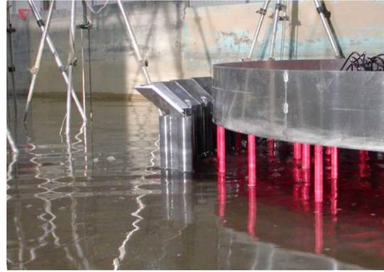
Figure 9f Return wall mounted on 16% porous lower section
