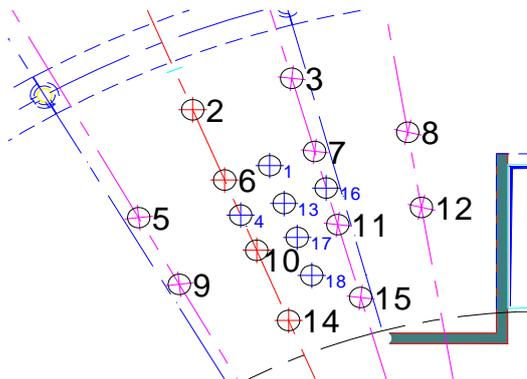
Figure 10 Array of pressure transducers used to measure wave-in-deck loads
