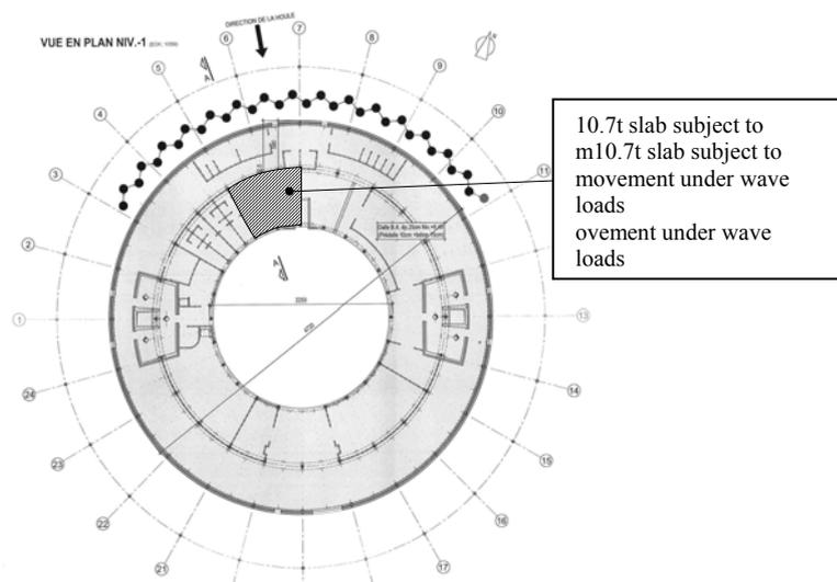
**Figure 5 lower level subjected to wave impacts**
