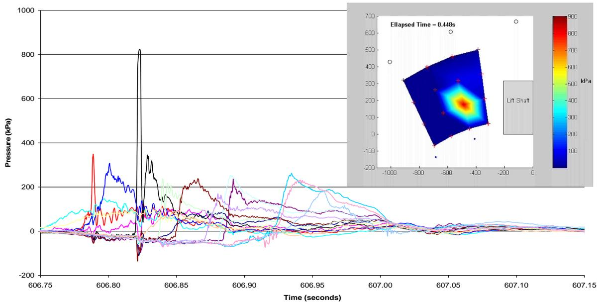
**Figure 11 Time series & spatial extent of wave-in deck load on pier without protection**
