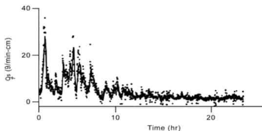
**Figure 1. Bed load pulses in a degradational experiment (from Venditti et al 2008)**
