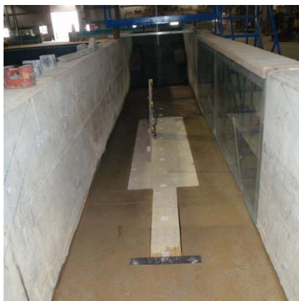
Figure 2 Layout of pressure transducer frame within model rubble mound
