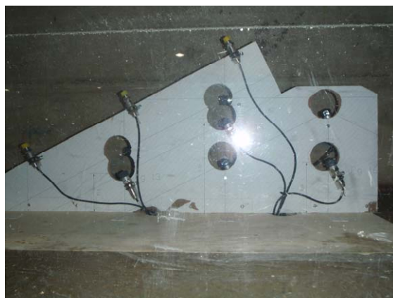
Figure 2 Layout of pressure transducer frame within model rubble mound
