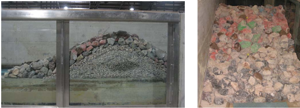
Figure 3 Final model of rubble mound breakwater
