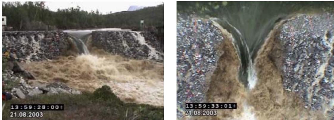
Figure 4 Evidence of flow separation and vorticity generation from field test
