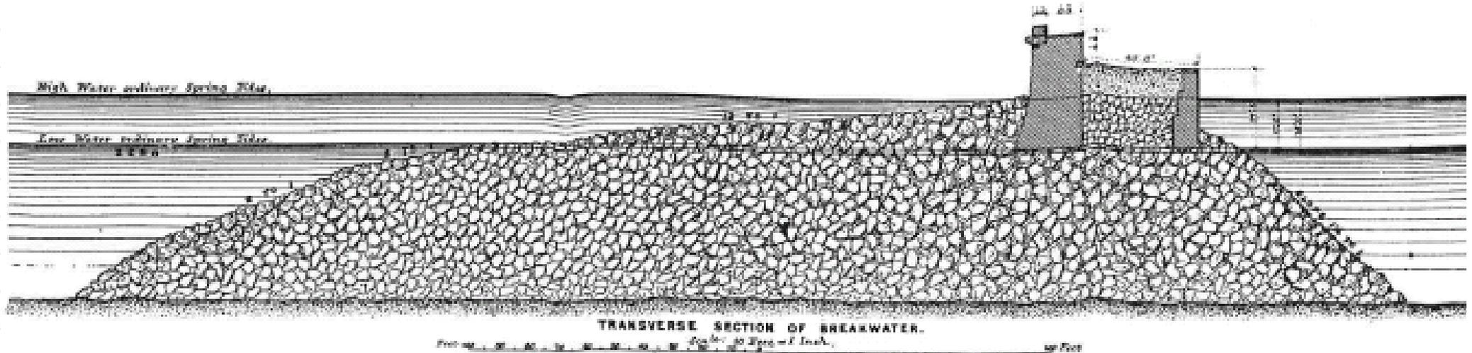
Wide mound to break waves before hitting the wall, but high mound can cause (longer) waves to shoal up and break impulsively against the wave wall
