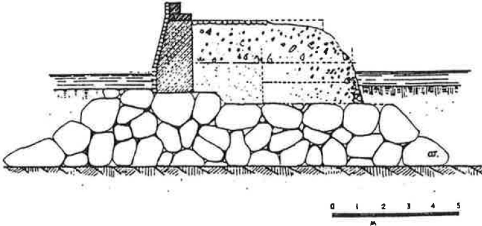
**Composite breakwater at Claudius Port (Rome) with concrete superstructure using ship hulls as lost forms**
