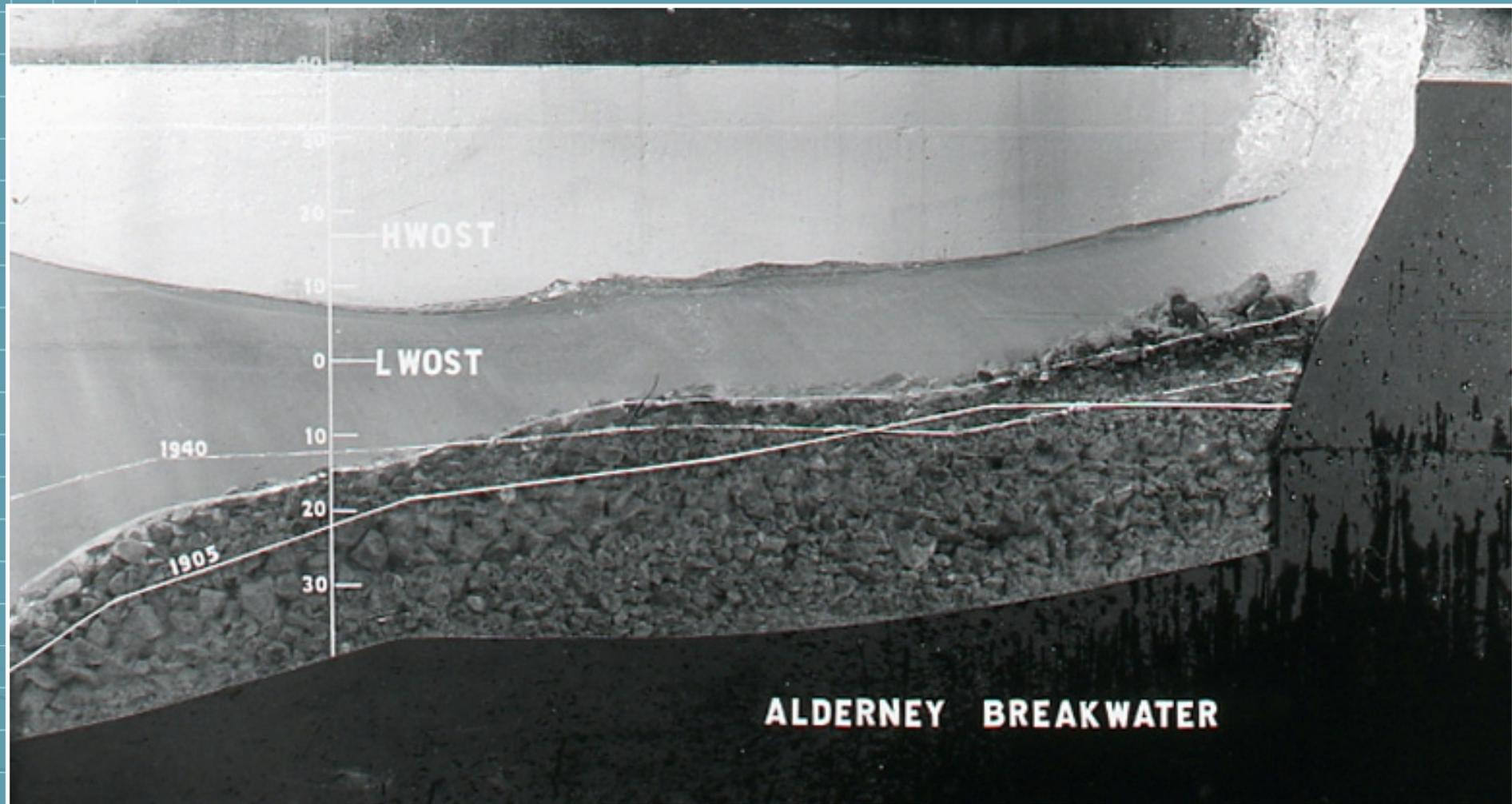
HRS model tests (circa 1965) studying movement of the mound material.
