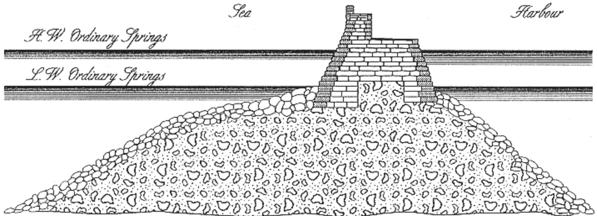
**Original design for Alderney (c. 1845), showing foundation mound up to just below low water, stone blockwork walls, un-cemented fill**
