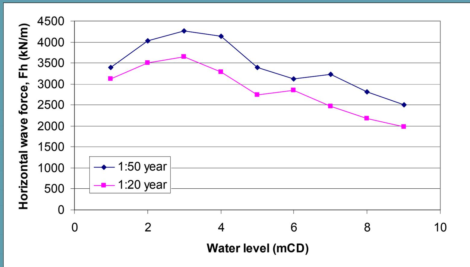
Wave loads (per m run) calculated using Goda + Takahashi for 1:50 or 1:20 year waves of  $H_s = 8.4\text{m}$  (or  $7.4\text{m}$ ).
