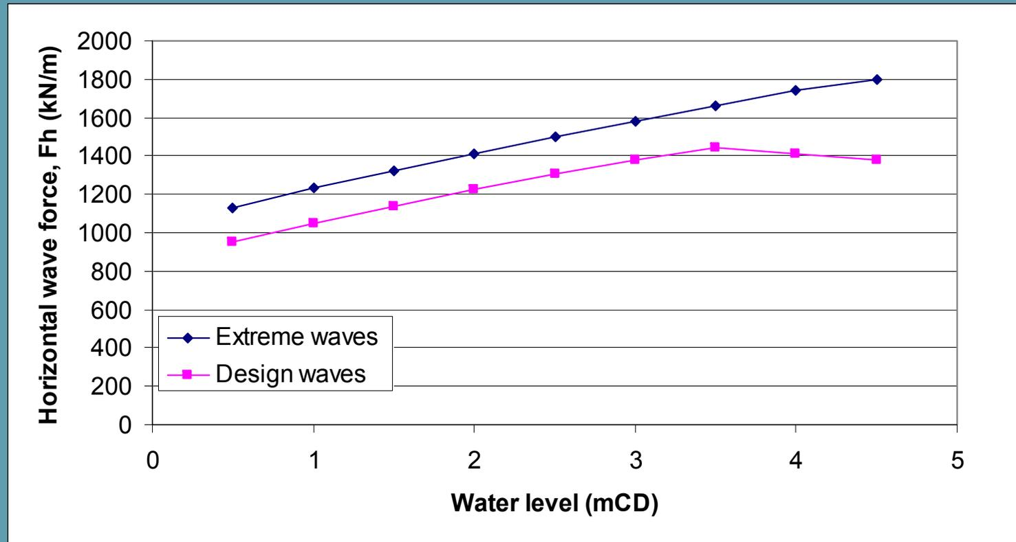
Wave loads (per m run) calculated using Goda + Takahashi for 1:10 bed slope, design wave of  $H_s = 5\text{m}$ , and extreme (revised?) condition of  $H_s = 8\text{m}$ .
