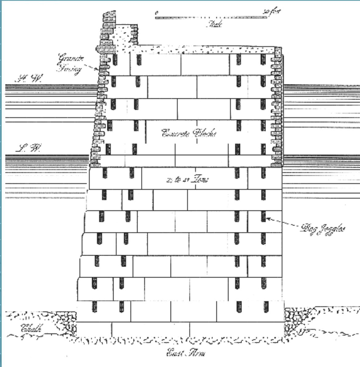
Dover breakwater, showing concrete blocks, use of bag joggle jointing, no foundation mound. Required large plant and divers
