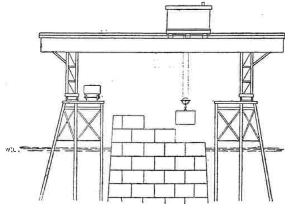
Construction tools, including placement frames and travelling gantry, diving bell for mound preparation
