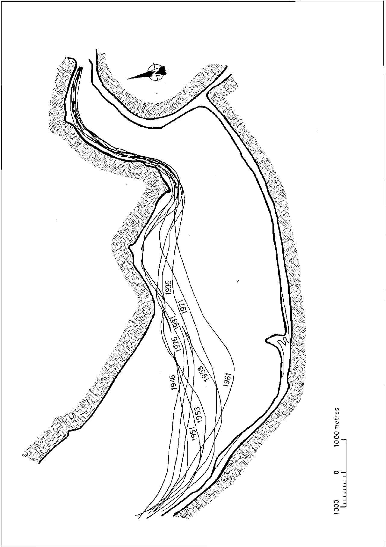
Fig 14 Mersey low water channel 1921 - 1961
